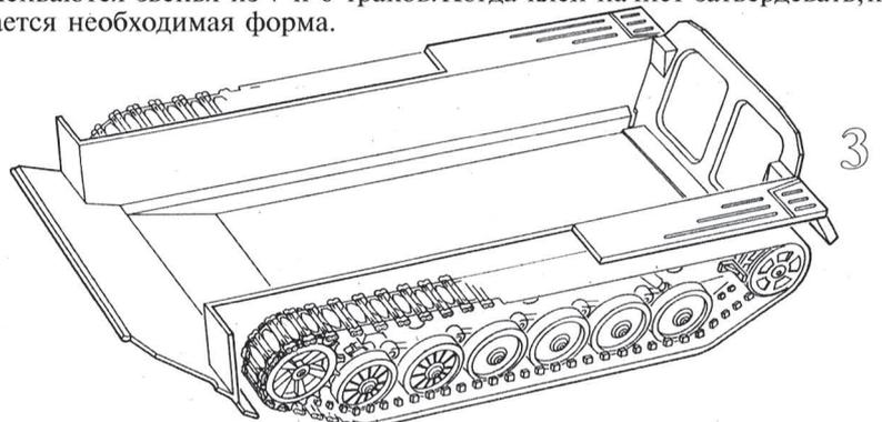
Catepillars are assembled of links made of 4,5,6,7,21, and 23 tracks. First glue the links of 23,21,4, and 5 tracks and only then the link of 7 and 6 tracks. When the glue begins to harden, shape the caterpillar.
