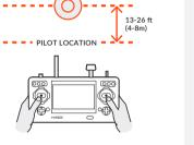
NOTICE: If the signal of remote control is lost, the TYPHOON H will automatically return to home point and hold its position (with a suitable GPS signal/lock) over the home position except for low battery.
