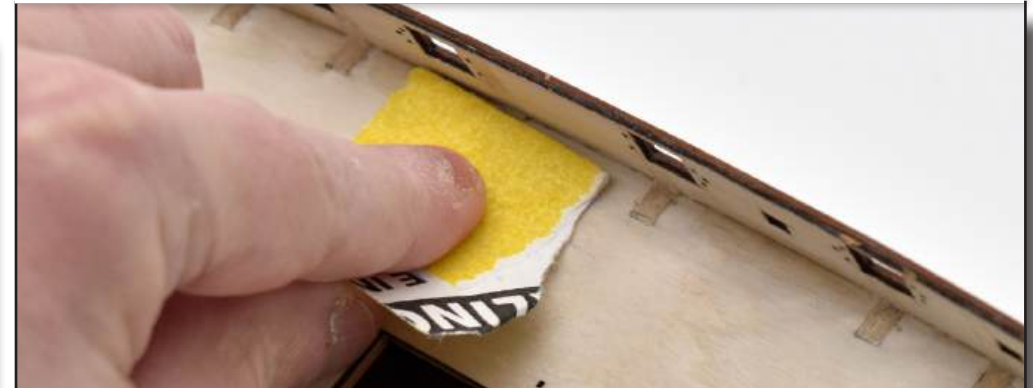
53. Remove all bulkhead tabs above deck level by carefully bending and twisting with a pair of pliers or similar. Once removed, sand any remaining stubs flush with the deck.
