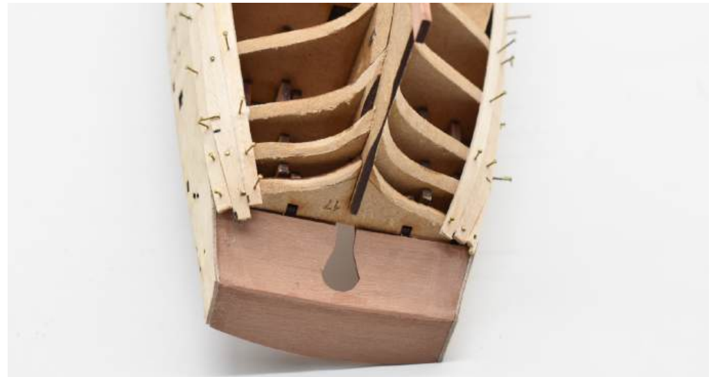
Three planks per side successfully pinned and glued in place.
