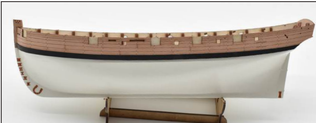
52. Paint copper and apply the depth markings (PE-27), the horse shoe (PE-18) and the stern fish plate (PE-19) to both sides. Use cyano gel sparingly to fix these parts in place.
