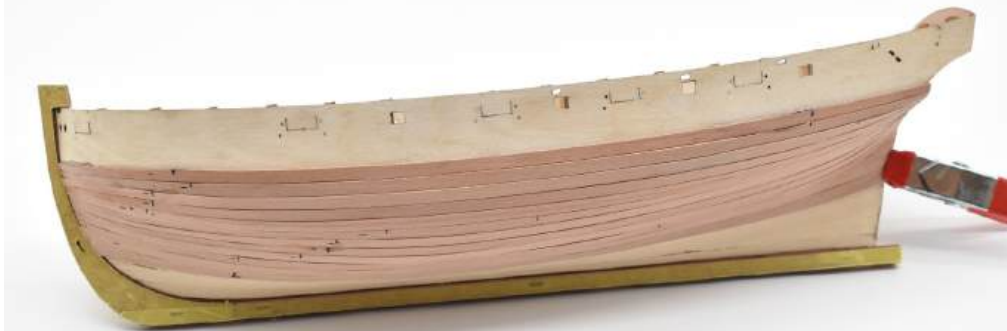
Planking progress with 12 planks per side done. Some stern planking is clamped to ensure they are fully adhered to the hull.
