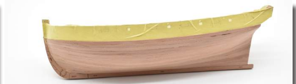
40. Second planking complete, sanded and filled. To get to this stage, several filling and sanding sessions were required. The filler used is a water based type, so it can be diluted and thinned, so it is able to flow into every gap. Before the sanding and filling process started, the engraved upper bulwark pattern area and the areas not to be painted white were masked off, as can be seen.
