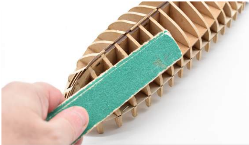
21. The hull can now be sanded to follow the smooth run of the planking and laser cut bulwark patterns. This process takes around half an hour of sanding.
