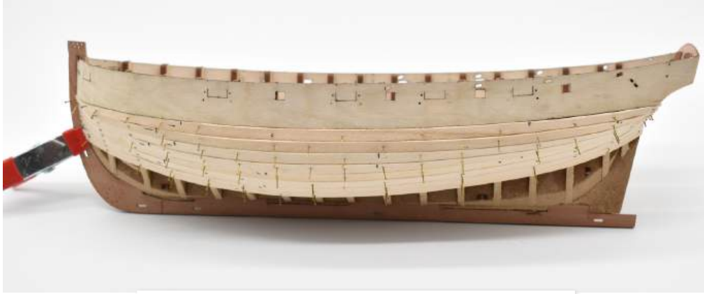
Several planks per side successfully pinned and glued in place.
