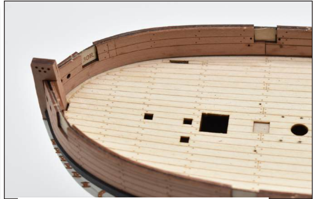
61. After 24 hours, remove the clamps. The bulwarks should now be firmly in place
