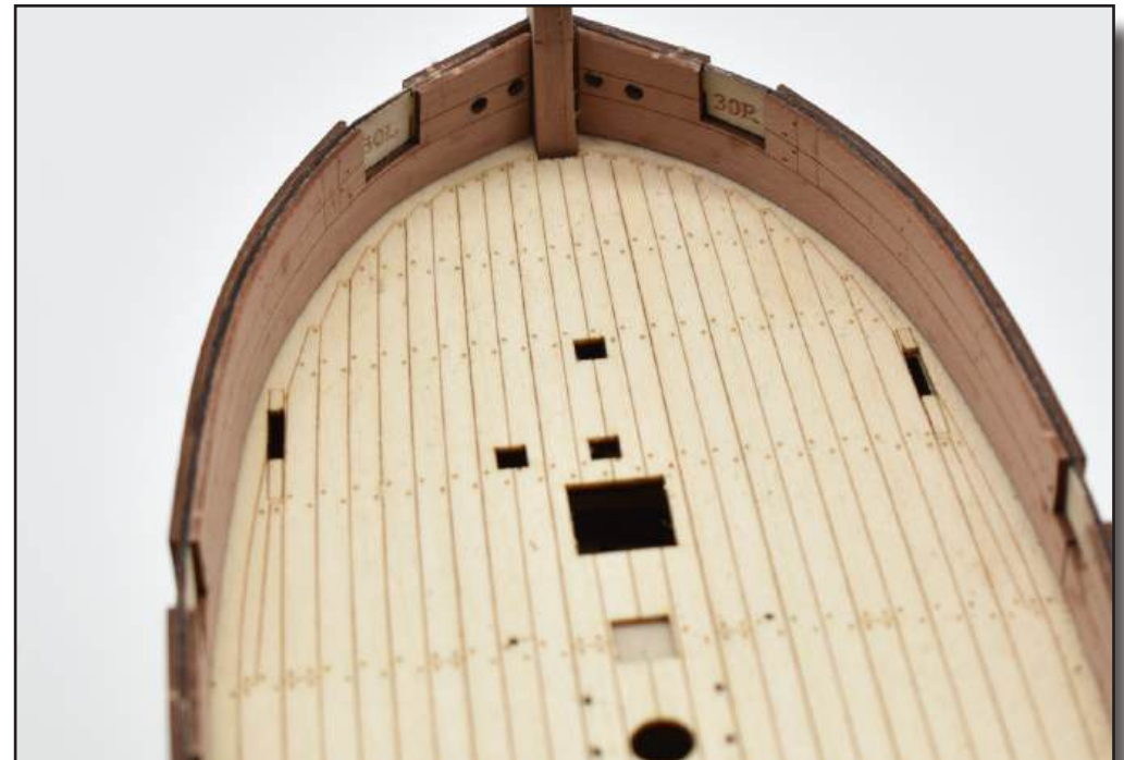
61. After 24 hours, remove the clamps. The bulwarks should now be firmly in place
