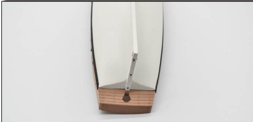
54. The laser engraved 1mm lime wood deck is now ready to be glued in place. Trial fit the deck and sand/file (below) any tight spots around the edges. Because there is another 'spirketting' plank that covers the inner bulwark, it does not matter if there is a slight gap between the deck edge and the bulwark sides.
