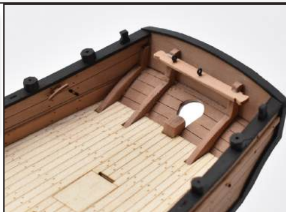
76. Remove the stern cross beam (87) from the 1.5mm wood sheet. Paint black and add the two eyebolts (PE-1), and then using PVA wood glue, fix the cross beam into the slots on the inner stern frames.
