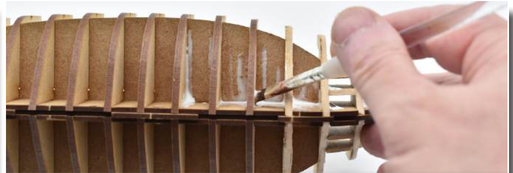
15. To further strengthen the hull assembly, you can brush on watered down PVA wood glue under the lower and upper decks.
