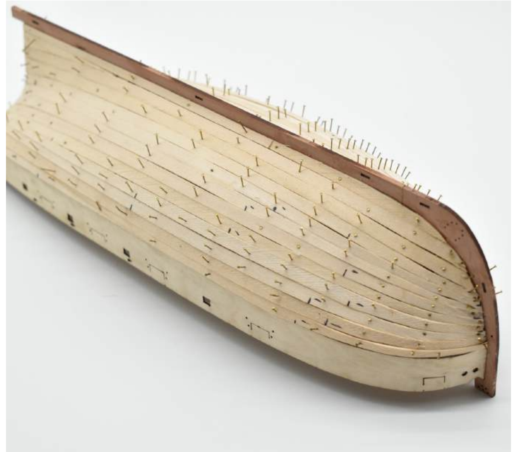
First planking complete. There are 12 planks per side, with a few 'Stealers' at the stern.
