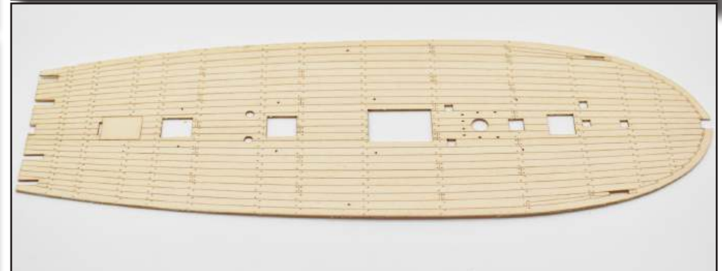
54. The laser engraved 1mm lime wood deck is now ready to be glued in place. Trial fit the deck and sand/file (below) any tight spots around the edges. Because there is another 'spirketting' plank that covers the inner bulwark, it does not matter if there is a slight gap between the deck edge and the bulwark sides.
