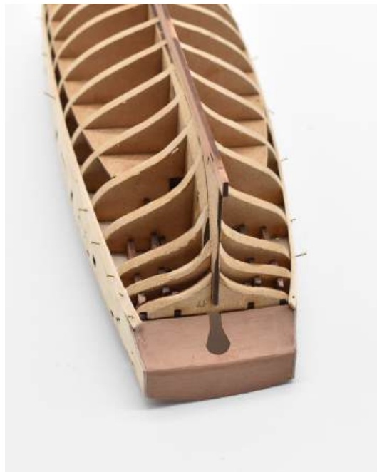
The first plank successfully pinned and glued in place.
