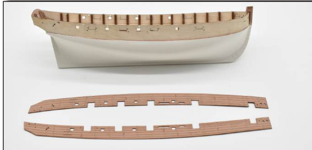
47. Now that all of the 'messy' work has been done, the outer bulwark patterns can now be glued into place. No pins were used, just claps. As with almost all wood to wood fixing, PVA wood glue was used. This was brushed onto the ply side, and the wood engraved bulwark placed and clamped in place, as shown.
