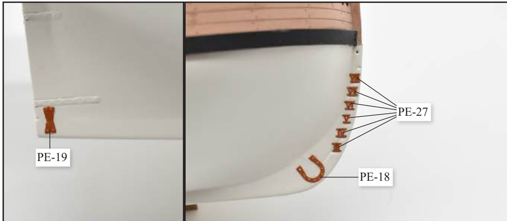
52. Paint copper and apply the depth markings (PE-27), the horse shoe (PE-18) and the stern fish plate (PE-19) to both sides. Use cyano gel sparingly to fix these parts in place.
