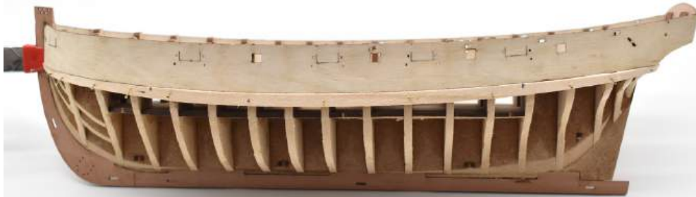
The first plank successfully pinned and glued in place.
