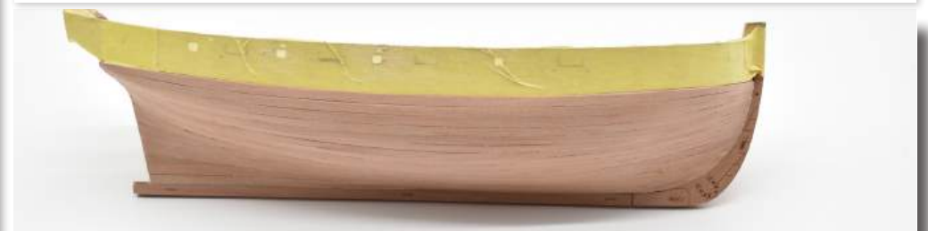
40. Second planking complete, sanded and filled. To get to this stage, several filling and sanding sessions were required. The filler used is a water based type, so it can be diluted and thinned, so it is able to flow into every gap. Before the sanding and filling process started, the engraved upper bulwark pattern area and the areas not to be painted white were masked off, as can be seen.
