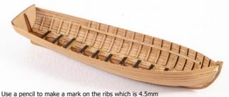
Use a pencil to make a mark on the ribs which is 4.5mm down from the upper bulwark. Glue the seat support strip, L31, underneath those marks and allow to thoroughly set. Note the rear ribs have been cut down so the seat, L27, can sit in place.
