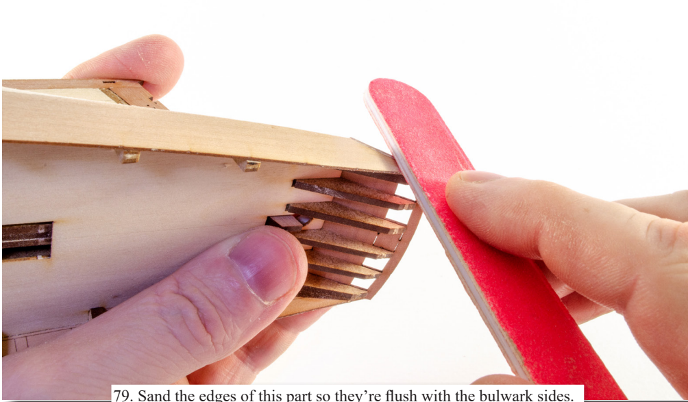
79. Sand the edges of this part so they're flush with the bulwark sides.
