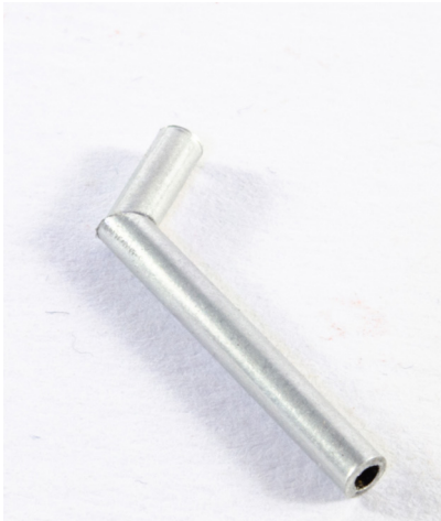
182. Take the 40mm length of aluminum tube and cut as shown on plan sheet #3. Glue together with CA gel.
