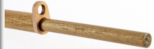
208. From the 1.5mm wood sheet, remove one part #95 and glue into position as seen here so the part sits snug into the shoulder where you reduced the dowel diameter.
