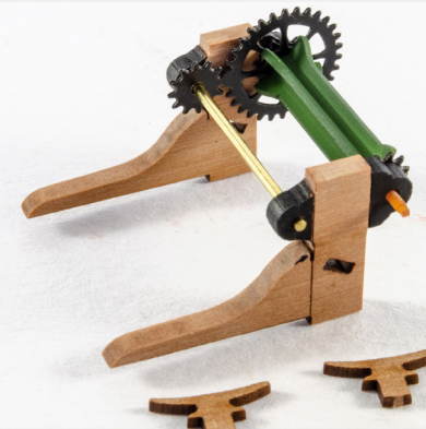
179. Make sure the brass rod protrudes at either side by around 0.5mm. Do NOT glue anything. From the 1mm wood sheet, remove both parts #82.
