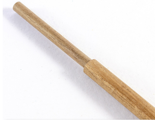
207. MAIN MAST: Using plan sheet 5 as your reference, cut the lower section of the main mast from 6mm dowel. This is 250mm long. You now need to evenly reduce one end of this to 4mm for a length of 39mm. Use a knife and sandpaper to achieve this.
