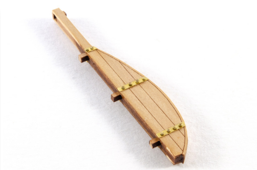
122. From the 0.2mm PE sheet, remove both sets of parts #PE-20, 21, and 22. Glue onto both sides of the rudder as shown on plan sheet #4. Use brass pins as bolt heads.
