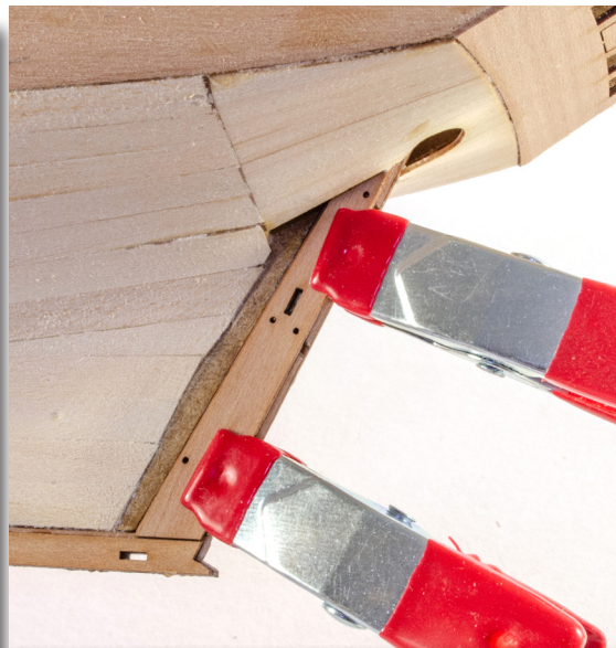
86. Glue and clamp parts #50 to either side of the rudder post, ensuring the peg holes are aligned. Now glue the pegs #58 into place. Once all keel parts are set you can trim all of them back, so they are flush with the outside of the keel.
