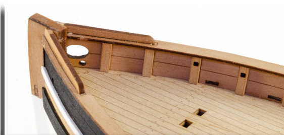
142. Glue into position on the engraved gunwale areas. You will need to bevel the forward edge, so they sit against the prow. You can now paint the gunwales in matt black paint.
