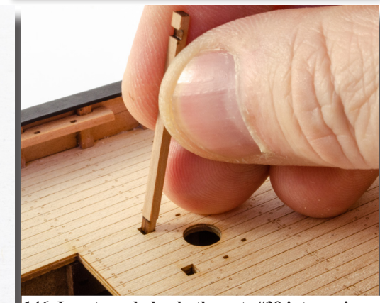
146. Locate and glue both parts #39 into position, with the slot in the upper area, facing aft. NOTE: The bottom of these parts MUST locate in the MDF sub deck. You can clearly see this by looking through the adjacent deck opening.
