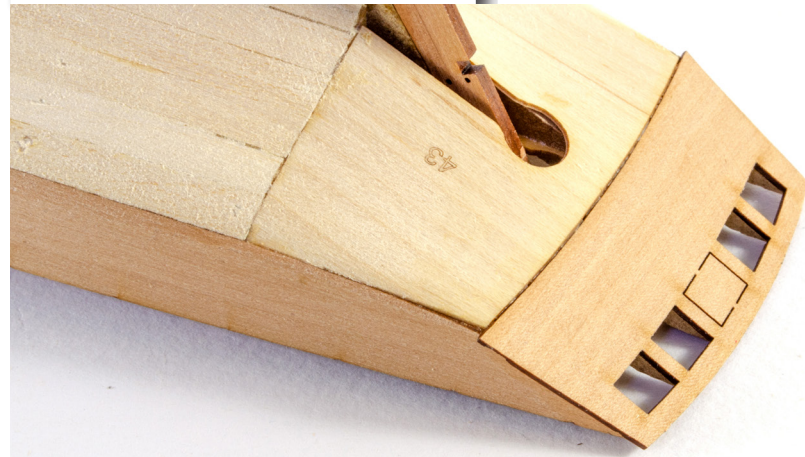
78. Glue into place as shown here and clamp until set.
