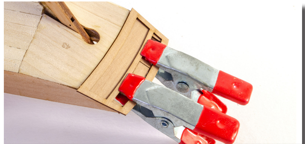
89. IMPORTANT!!! DO NOT GLUE this part into place. Instead, just align it with the stern and simply clamp it into place, temporarily. We are doing this so we can put the following part in its correct position.
