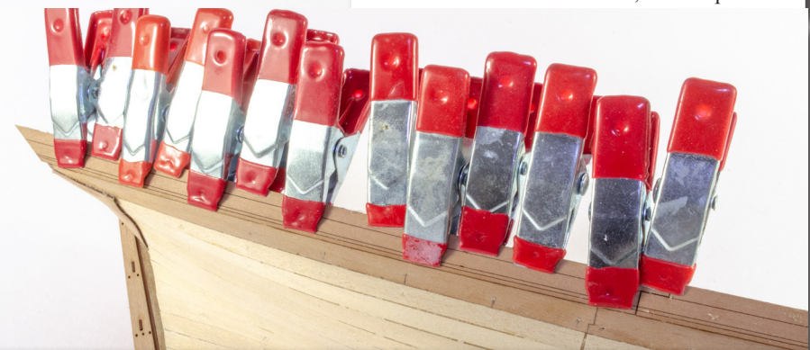
97. Glue and clamp this into position as shown here, with the top edge running along the top edge of the inner bulwark. Leave to dry.
