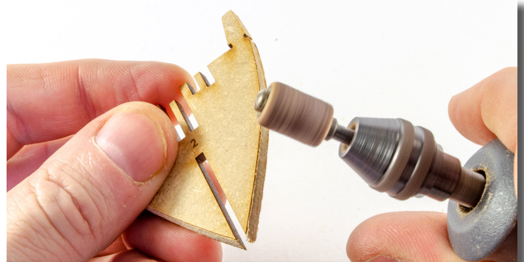
7. Take all bulkheads that have engraved lines and separate from the others. These are bulkheads #1, #2, #3, #11, #12, and #13. You now need to bevel these from the outside edge to the engraved lines on each part. You can do this with either sandpaper, sanding stick, or a rotary tool such as a Dremel.
