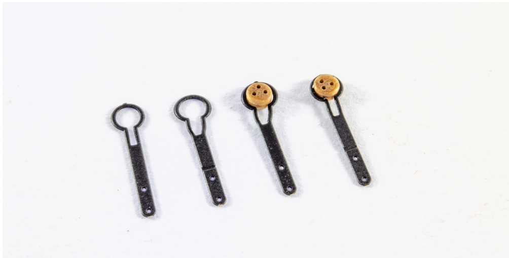
199. From the 0.4mm PE sheet, remove eight parts of #PE-2. Here you see the sequence for inserting the 3mm deadeyes. Use a tool (tweezers, pliers etc.) to open up the loop a little. Insert the deadeye, and then close up the loop to how it previously looked.
