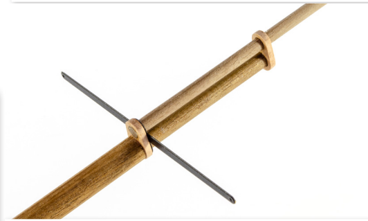
210. Make the upper section of the mast, complete with the taper towards the top, and then fit this to the assembly you've made, using the other part #95 at the very top of the lower mast section. Make sure everything is properly aligned. This is important.
