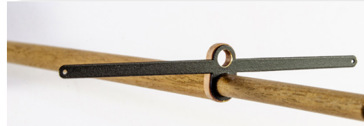
209. From the 0.4mm PE sheet, remove part #PE-15 and paint black. Glue into place as seen here. It's a good idea to use a length of 3mm dowel to make sure the opposite hole aligns with the one in the wooden block.
