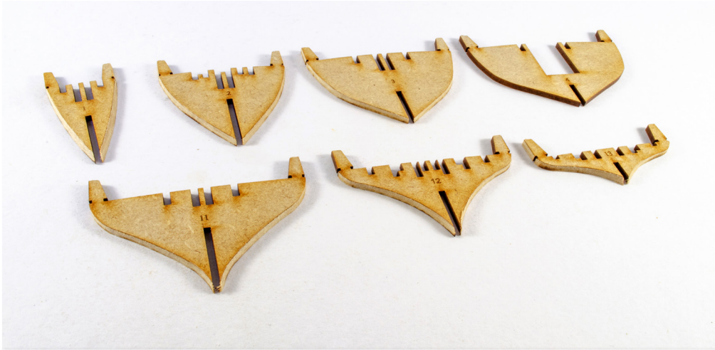
8. This is what the seven bevelled bulkheads will look like. Don't worry if you went a little too far as these will be further bevelled when the hull frame is sanded (faired).
