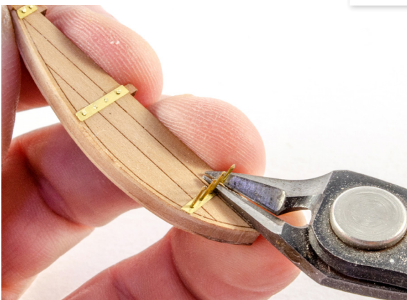
123. Snip off the remaining length of brass pins. You can, if you wish, use shortened pins, and have the domes heads on each side of the rudder.
