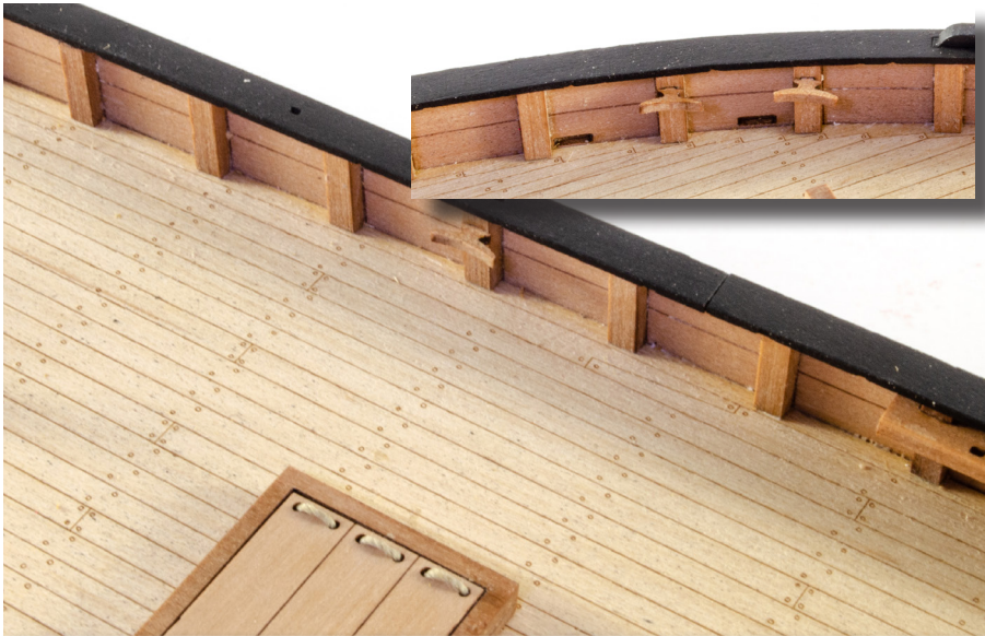
187. From the 1mm wood sheets, remove the cleats #83 and glue into the positions shown on both sides of the hull.
