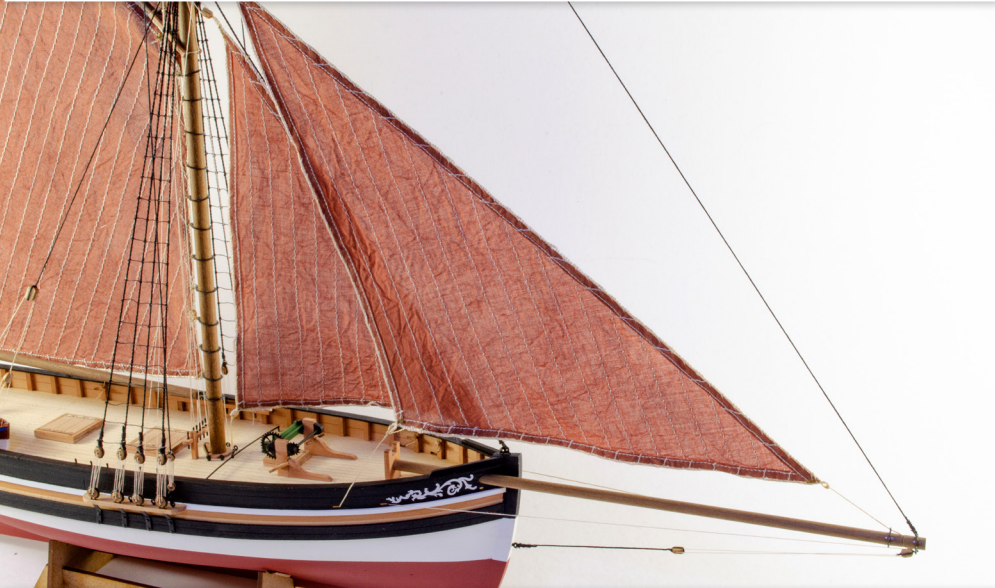
231. The upper jib can now be fitted. This is very easy. Use the plan and photo as an approximation of the sail position.
