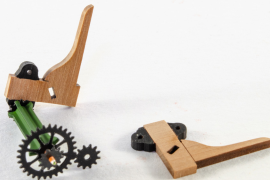
177. On the wooden parts, paint the brackets in black. Now take part #36 and fit (no glue) to the previous assembly.
