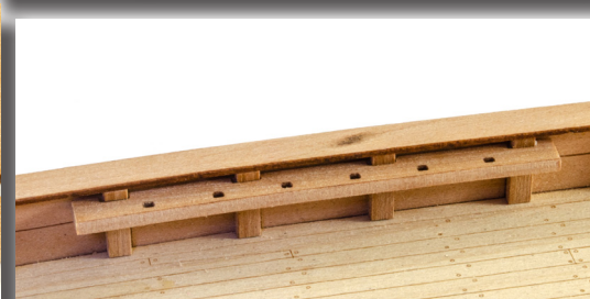
144. Remove one at a time and glue into the engraved recesses on the previously co-joined timberheads, making sure the front of the rail is facing the bow. Do this for both parts on opposite hull sides.
