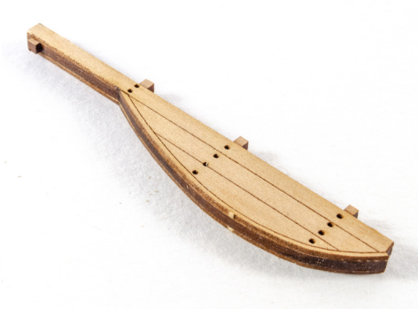
121. Your rudder should now look like this. You can now remove the char from the edges.
