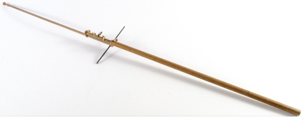
212. At this stage, your mast will look like this. Don't add any further PE to it unless you aren't fitting the sails. If you aren't using sails, then you can slip the main sail rings #PE-16 into place (no glue) followed by #PE-9 which needs to be glued 52mm from base of mast.
