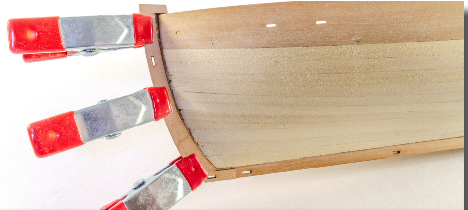
81. Glue both parts #49 to the prow, as shown, one on each side. Make sure the locating peg holes are aligned.
