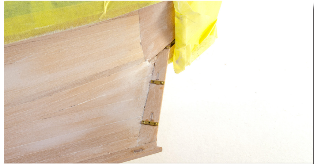
118. From the 0.2mm PE sheet, glue parts #PE23, 24 and 25 (both sides) as seen here and on your plan sheet #4. Use brass pins as bolts and cut off the remainder at the opposite side.
