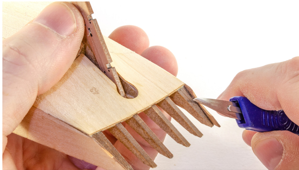
75. Use a knife to trim the excess length from the bulwarks, so they are about flush with the stern timbers.
