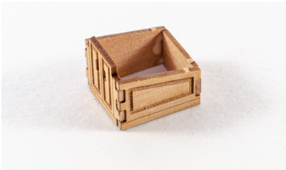
163. Now glue the rear panel into position to complete the housing.
