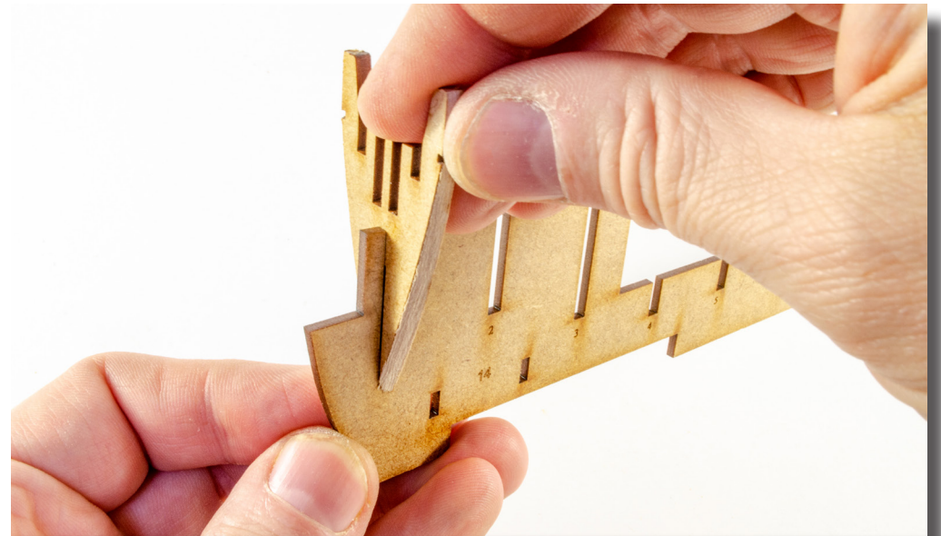
11. Take bulkhead #1 and slot into position as shown. Note that the bevelled side faces forward. Also, DO NOT glue any bulkheads at this time.
