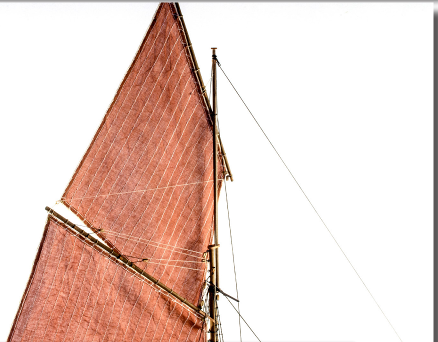
229. And here you see the position of the top sail in relation to the main sail.
