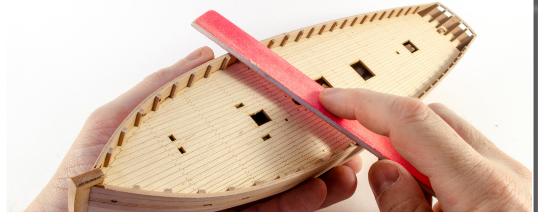
115. Use a sanding stick or a ruler wrapped in sandpaper and draw this along the top of the bulwarks. This will sand the timberheads to the same height as the bulwark. A good indicator that you have sanded properly will be when the char is removed from the top of the bulwarks. Remember to sand the stern fascia top to the same height as the bulwarks.
