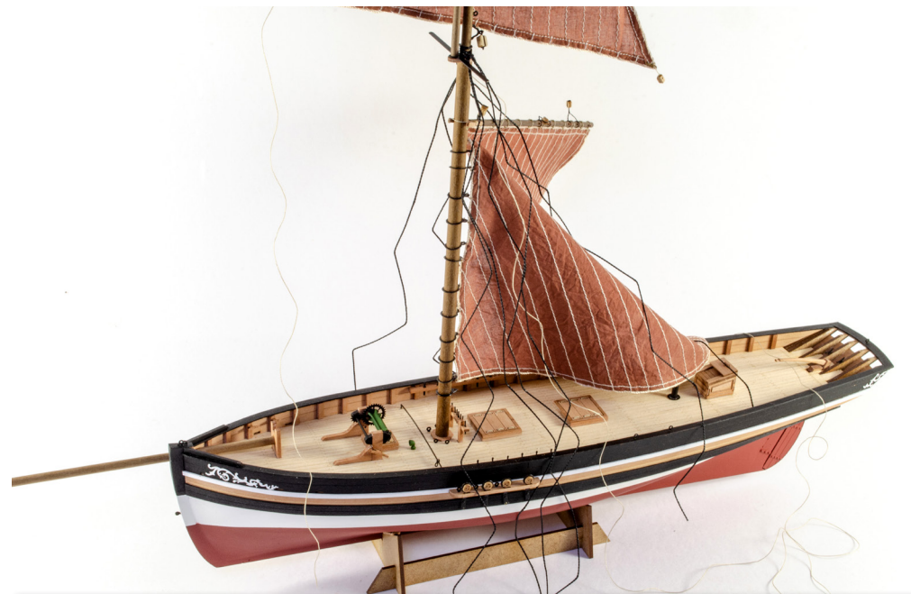
219. We now need to add the shroud lines, as per plan. These are from 0.75mm black thread. These are added in pairs, on alternate sides, each time.
