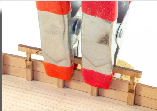
111. Now glue and clamp this part next to the other timberheads, as shown.
