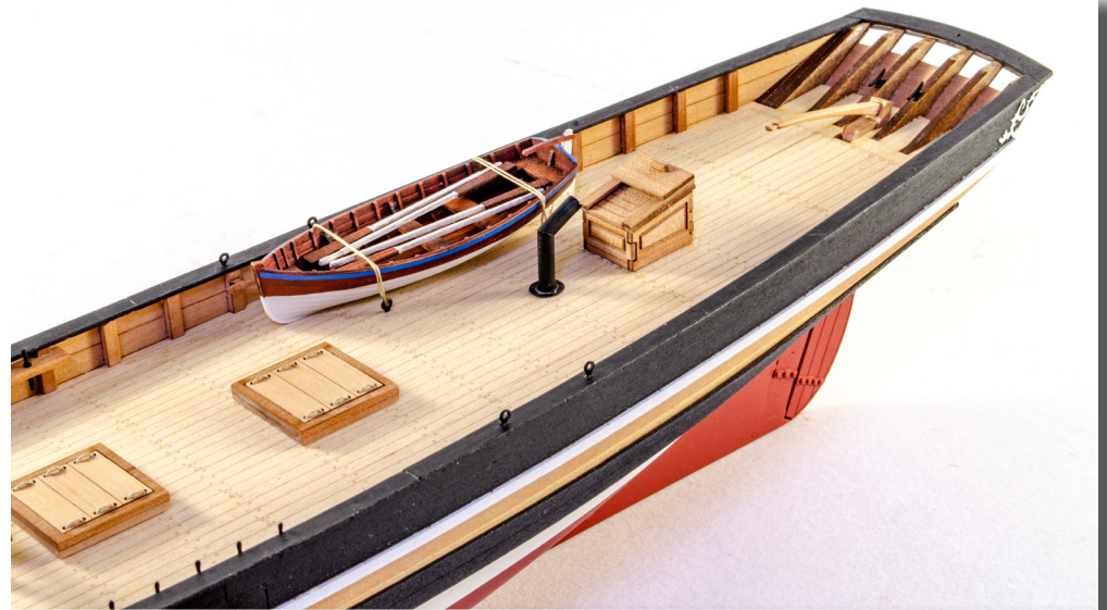
203. The boat is now lashed to the deck via the four eyelets and some 0.25mm natural thread. In these photos you can see the completed deck works.
