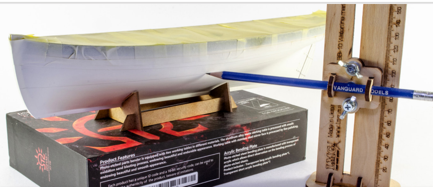
127. Using your plan sheet #4 for reference, add the waterline mark from bow to stern, both sides. If you don't have a waterline tool, we sell them in our online store, and they are inexpensive.
