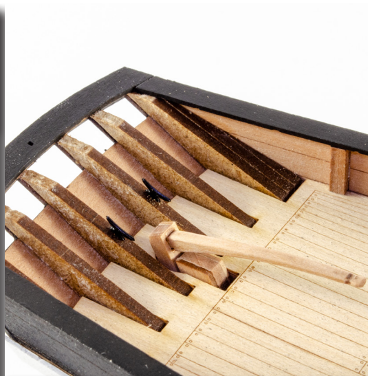
188. From the 0.4mm photo etched sheet, remove the cleats #PE-17 and glue into place on the two innermost stern timbers. Paint the parts black.
