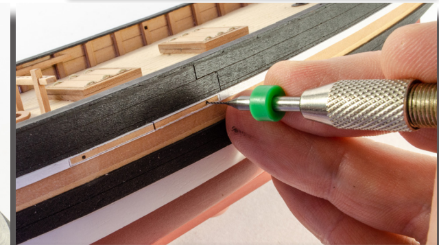
197. Drill the accompanying holes in the outer rails, about 2mm deep, taking into account the thickness of the rail into that calculation.
