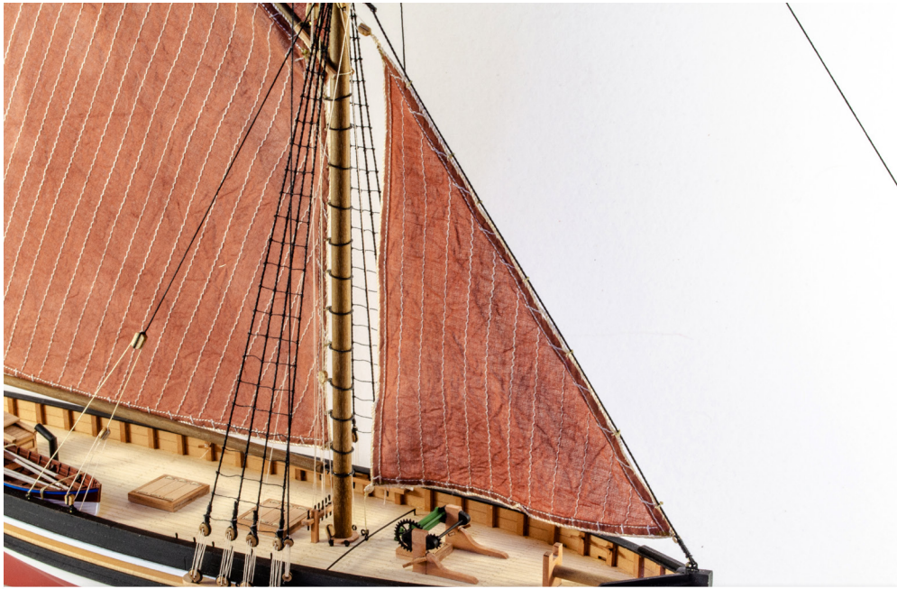
230. Fit the lower jib sail as shown. Start by threading it to the fore stay and then rig the lines and blocks.
