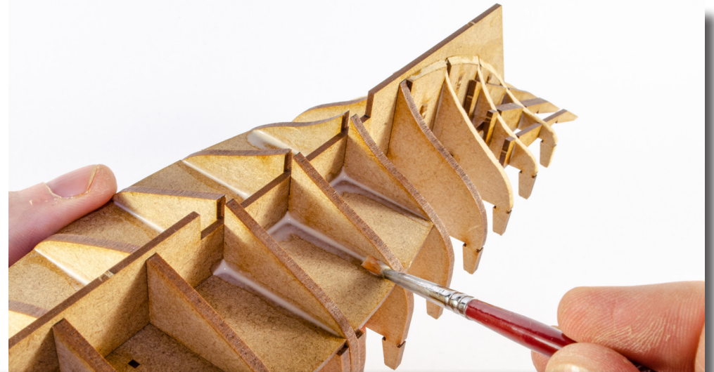
40. Make sure that everything is pushed firmly together, and nothing is misaligned. Now, brush slightly diluted wood glue into the various slots and joints around the hull. Once done, leave to dry for a few hours.
