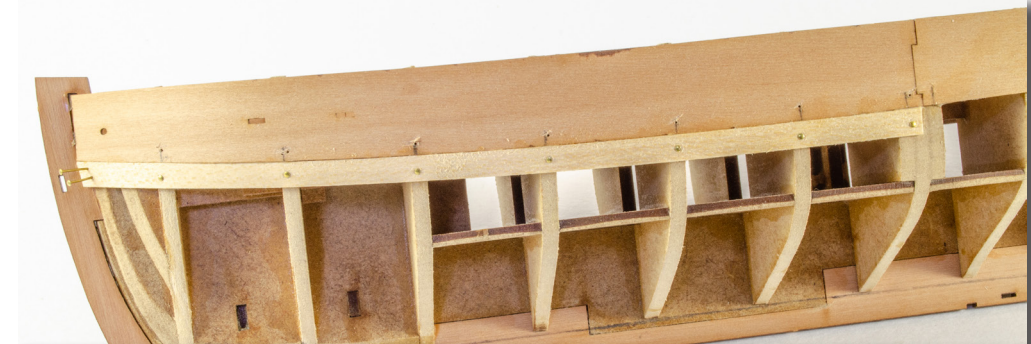
67. It's now time to start adding the first layer of lime planks. Take of the wider and thicker lime planks and glue it immediately underneath the bulwarks. This does not need to be tapered. You can also install the plank in halves if you wish, as we have done here for you. Remember to pin the planks and also glue them to each other along their length.
