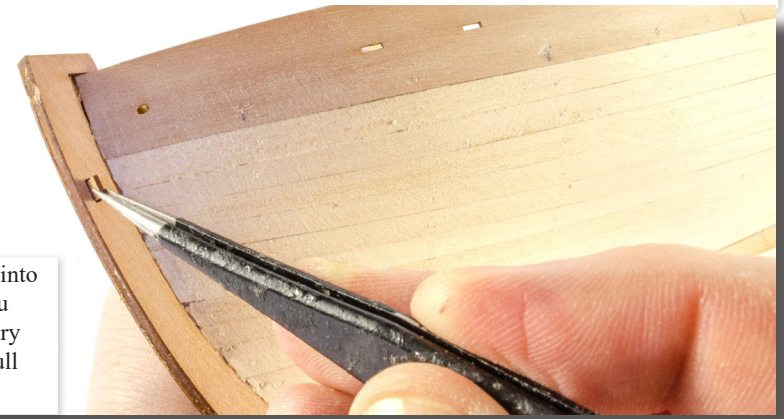
81. Glue both parts #49 to the prow, as shown, one on each side. Make sure the locating peg holes are aligned.
