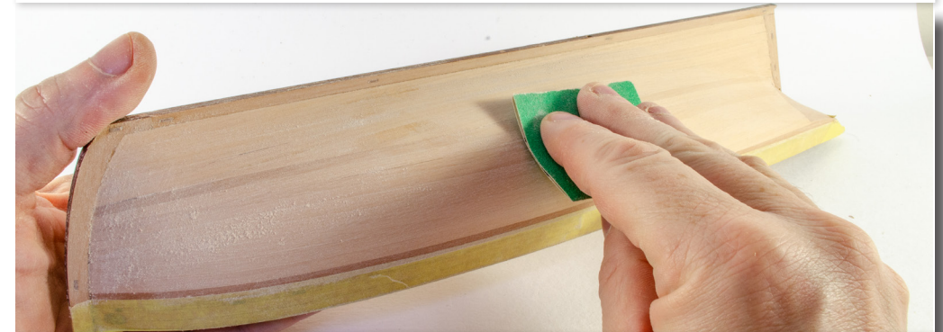
101. Mask off the engraved areas on the upper bulwarks and sand the hull so that it's smooth. If there are any areas that require filling, then we'll do that later.
