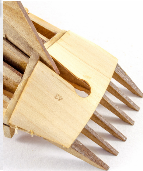
58. Glue this into position as shown here, with the narrow edge meeting the stern timbers at the point where they change angle. Maple veneer is very easy to bend. You may wish to glue the narrow edge first and then leave to dry before forming the wider edge against the underside/bulkhead #13.
