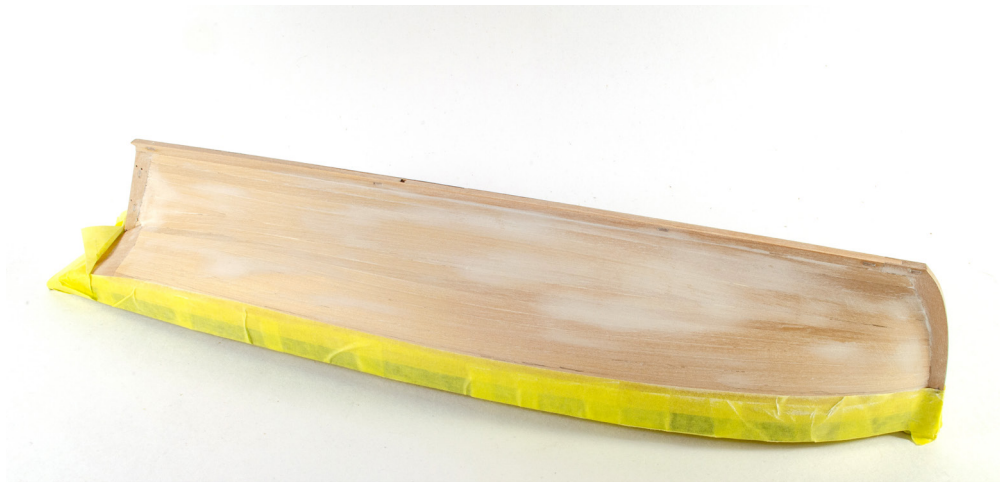
117. From the 0.8mm wood sheet, remove the wales, parts #65 and #66. The top edge of these will be approximately 14.6mm from the top of the bulwark. Draw a pencil mark along the bottom edges of these parts then put them safely away until later. Now mask the hull to just inside your pencil line and then proceed to use wood filler to fill any imperfections in your planking. Keep checking your work, refilling, and sanding until you are happy with it. We use acrylic wood filler, slightly diluted with water and applied with a brush.
