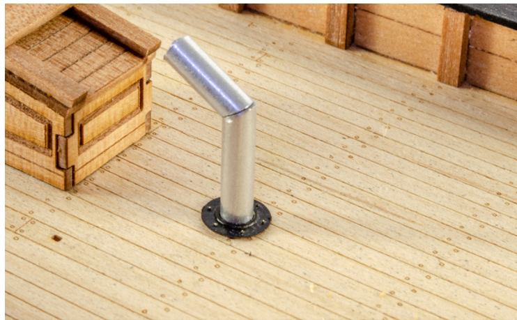
183. From the 0.4mm PE sheet, remove part #5 and paint black. Slide this onto the bottom of the chimney you just made and fit the assembly to the deck. NOTE: You may need to run a 3mm drill through the hole to clear away any MDF protruding into the hole area.
