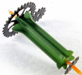
175. Prime and paint the windlass drum. We chose a flat green colour. Paint the PE parts in black. Slide #PE-3 onto one side and then one #PE-4 onto each side too, in that order. Don't use any glue here.
