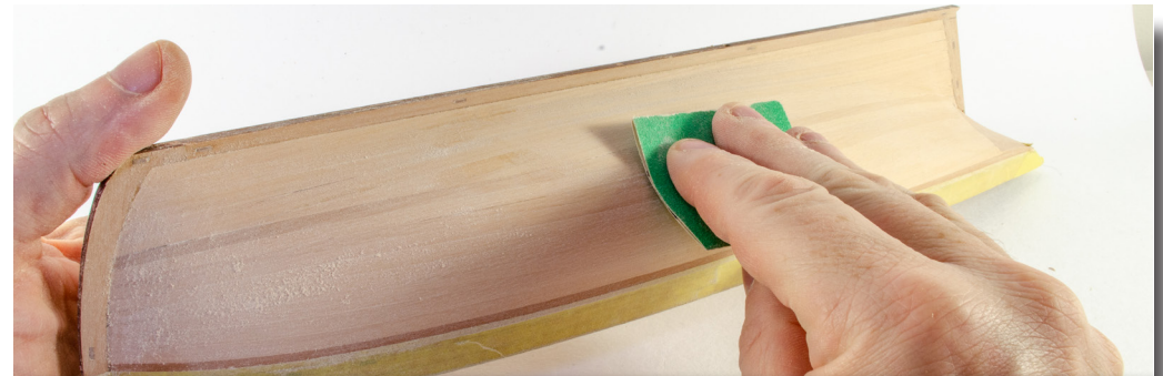
100. You must now use the strips of pear wood to plank the outside of the hull again, covering the initial layer. The first plank will sit directly under the bulwarks you just added. IMPORTANT: Try to add at least the first couple of planks as full length as some timber will be seen if using our paint scheme. Also note that it isn't appropriate to use brass pins for these planks as you could ruin the overall finish of the hull. Instead, we recommend using a good quality CA gel, such as that made by Gorilla. We apply this in small dots along the length of each plank before easing it into position. The glue grabs very quickly but allows you a second or so to reposition. It is also important that you taper your planks and edge-bevel them, so they sit snugly up against the previous plank.
