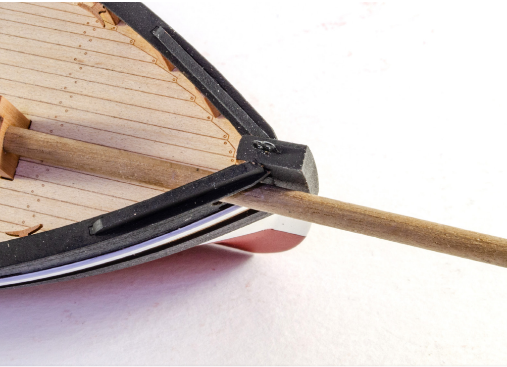
193. When complete, you should be able to insert a length of 4mm dowel through the hole and into the bowsprit support block, with no wobble at the bulwark.
