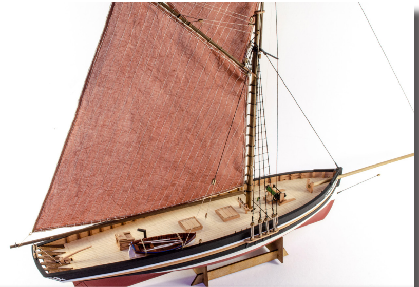
228. This photo gives you a good idea about how the main sail is rigged, with position of the sail on the mast.
