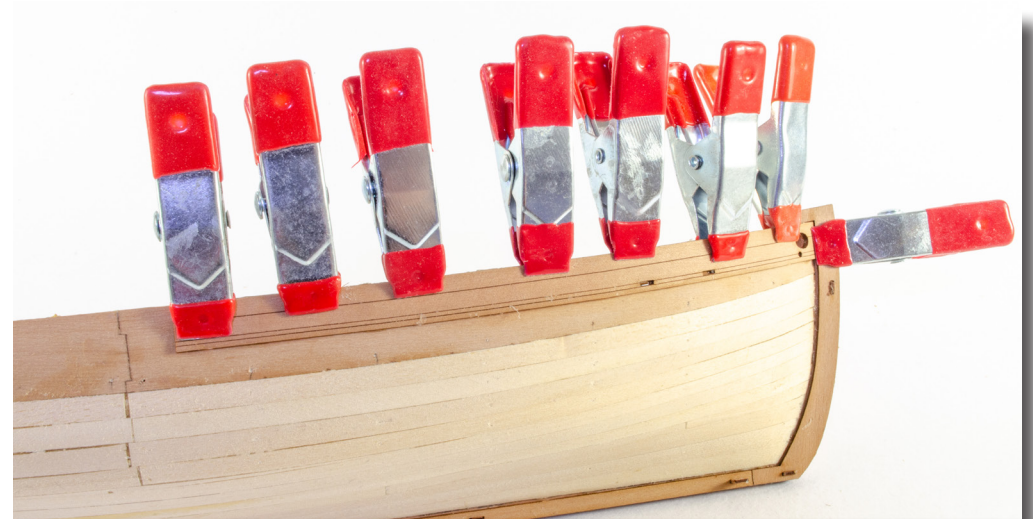
95. This is now glued and clamped to the outside of the right-side bulwark. You may need to trim/angle the front edge where it fits into the rebate, and also made sure the scupper holes (the two narrow slots) are aligned with the inner bulwark. Again, there is flexibility to slightly trim length from the front of this part. The top of this part must be level with the top of the inner bulwarks.
