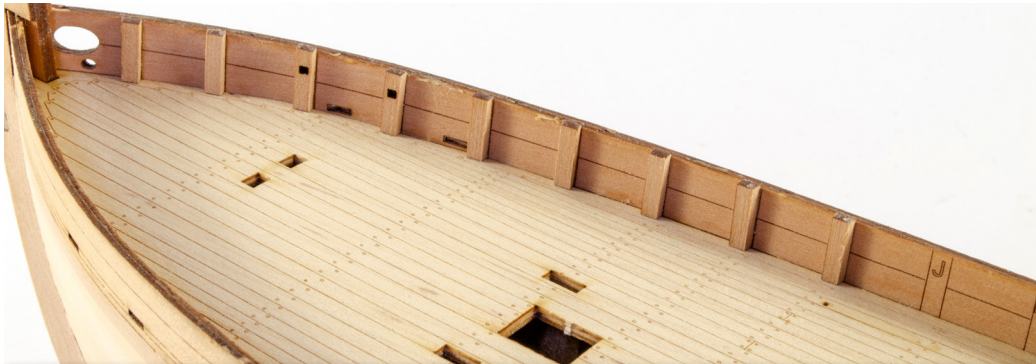
109. Remove one at a time from the parts sheet, and glue them inside the bulwarks, A, B, C, D, etc. This is how those initial ones will look.
