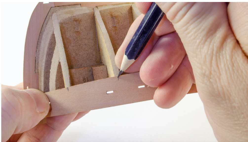
61. Insert the front edge of this part into the slot on the wooden prow, then clamp in place so the top edge of this is in line with top of bulkheads. Now use a pencil to mark the bulkhead positions.
