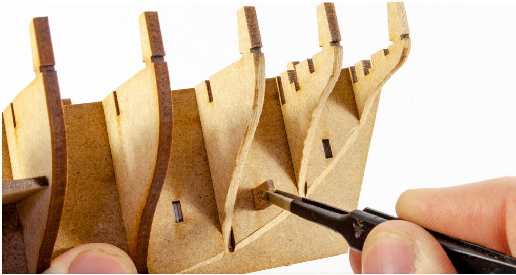
26. Now take the locating pegs #28 and glue into place, though all the way through the parts you just added, and through the keel.
