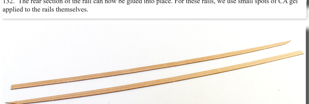
130. From the 0.8mm wood sheet, remove parts #63 and #64. These form the upper rail for the right-hand side of the hull. You can also remove parts #61 and #62 for the left-hand side of the hull. Don't get them mixed up. Note that when you sit them together, there is an engraved area. This needs to be masked so no varnish or paint gets in that area. Varnish the parts and then paint white.
