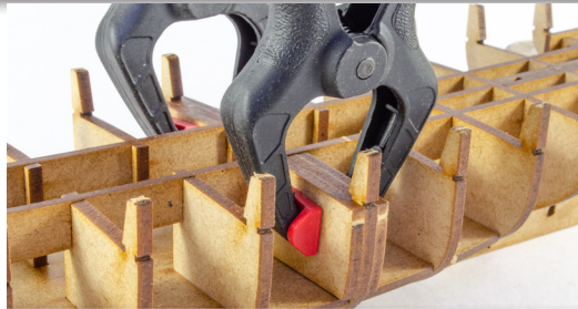
38. With the deck part properly pushed into place, parts #7a can be glued to either side of bulkhead #7, tripling the thickness in this area. Clamp until set.
