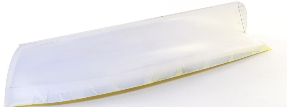
126. We primed our hull in Tamiya Fine Surface Primer (white) and proceeded to fill and sand any further blemishes which showed up. Once happy with the finish, a final coat of Plastikote Matt White was applied to the hull.
