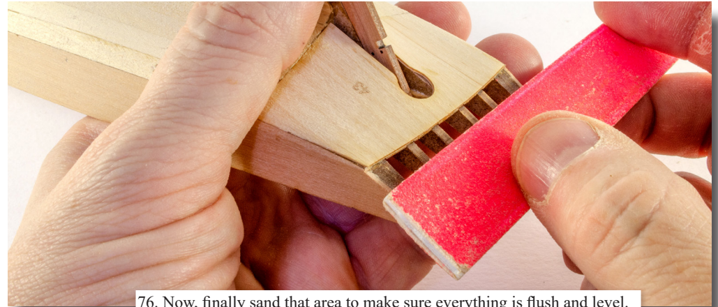
76. Now, finally sand that area to make sure everything is flush and level.
