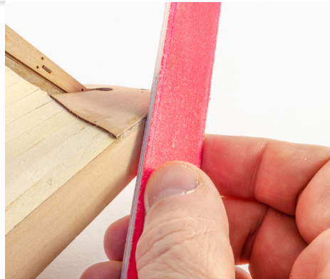
93. Sand the edges of part #53 flush with the sides of the hull.
