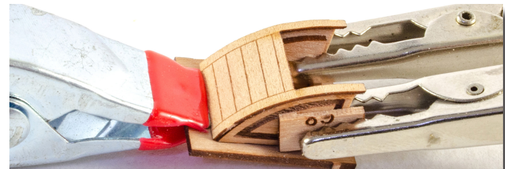
145. Carefully bend the part over the curved assembly. We suggest CA gel for this as you won't need to clamp anything.
