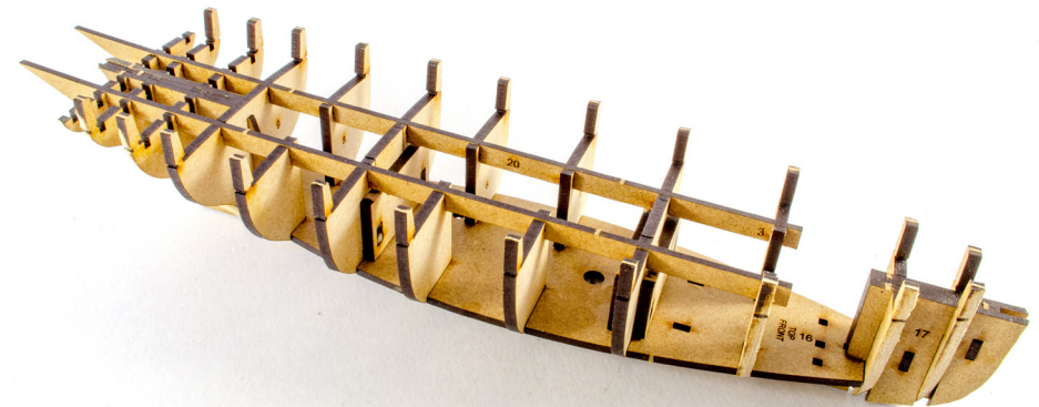
32. Dry fit (no glue) both parts 20 into the slots on top of the bulkheads. The front of parts 20 will first fit into the top of bulkhead #3, with the rear sitting at the stern. You may need to joggle the bulkheads a little to make it sit fully. Do not use any force. If you feel the need to use force, it's because something isn't sitting properly and you need to check your construction.
