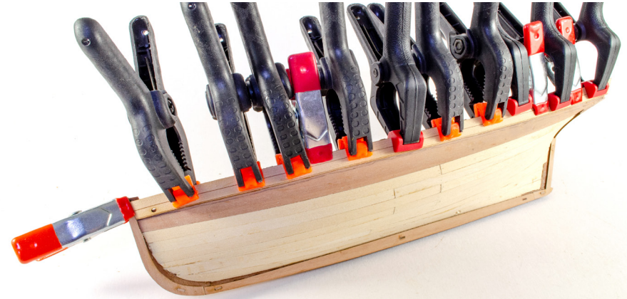
81. Take part #44 and glue into position so that the top edge is the same height as the inner bulwark you are gluing to. NOTE: The front of #44 will neatly sit in the rebate that the keel rabbet created, and up against that part. You may need to bevel #44 at the front edge, but we didn't need to for the prototype. Leave the bulwark to dry once clamped.
