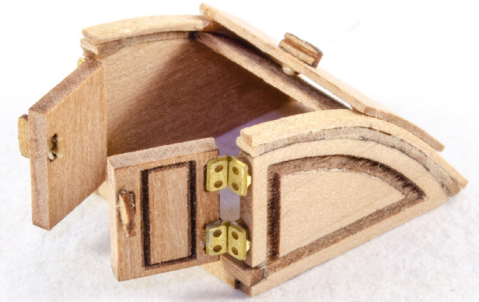
154. Glue the completed doors to the companionway, and add another handle #36 to the hatch roof.
