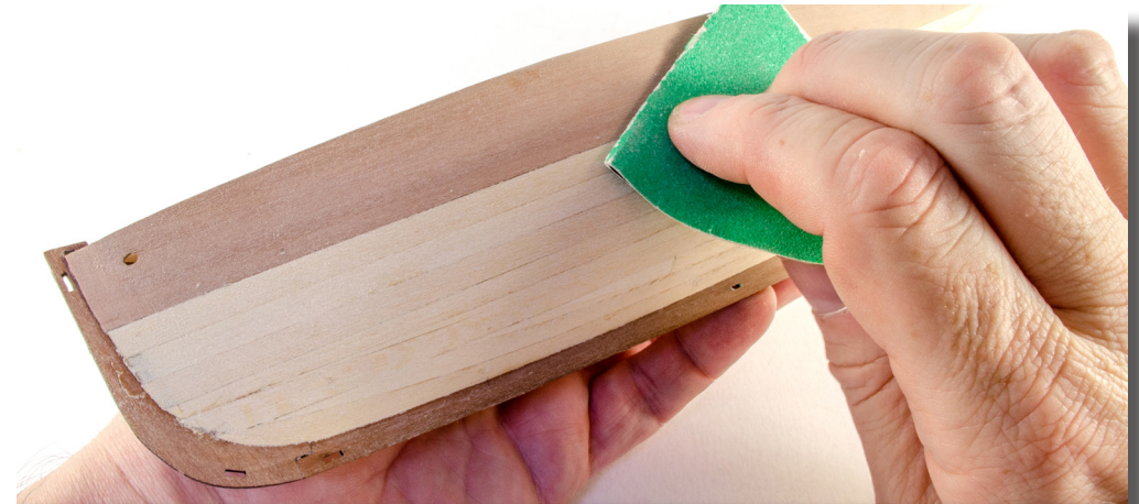
67. Using sandpaper or around 110 grit, sand the whole hull smooth so that the planking blends into the bulwarks and all planks are smooth to the touch. Ensure there are no unevenly-levelled planks and that you are creating a smooth surface onto which the next layer of planks will fit. The whole hull will feel like one unit. Towards the stern, gently round the rear of the bulwark where it curves into the inner stern counter.
