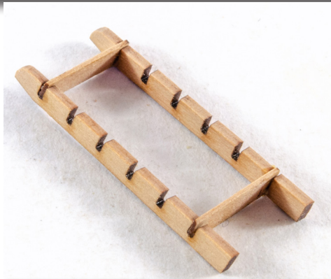
134. Glue the opposite ladder side into position and leave to set.
