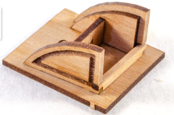
143. Make sure the assembly is properly positioned with the front bar up against the jig sides.
