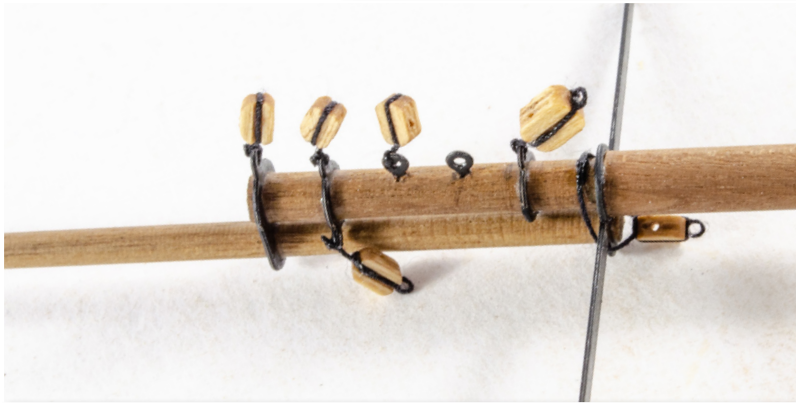
208. Fit the mast out with the PE eyelets and the correct rigging blocks.
