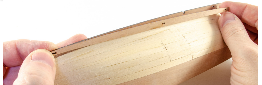
69. Test fit the keel rabbet part against the hull. You will find it only comfortably fits in one direction, where the peg locating holes align.
