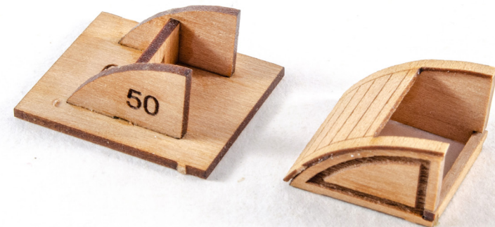
146. Once set, remove the assembly from the jig. The jig can be discarded.
