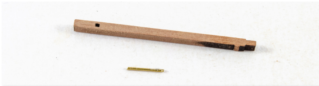
181. FAIR LEADING POST: Remove part #80 from the 2mm wood sheet. Also cut a length of 0.5mm brass wire, 6mm long. Glue the brass wire through the hole in the post.
