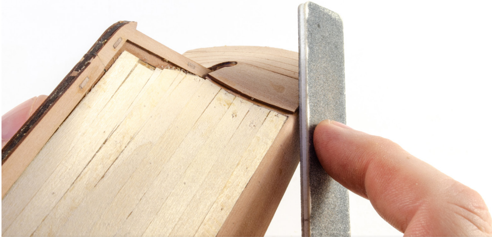
79. When the glue is dry, sand the overhanging areas of this part so they are flush with the side of the bulwark.
