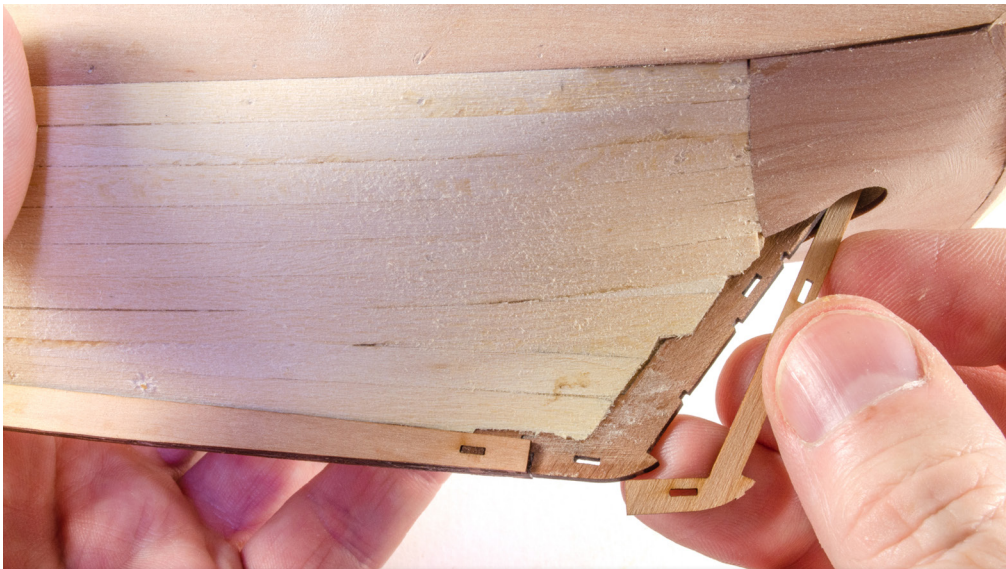
75. Slot part #57 up into the rudder post hole on Nisha and you will see how the locating slots align.
