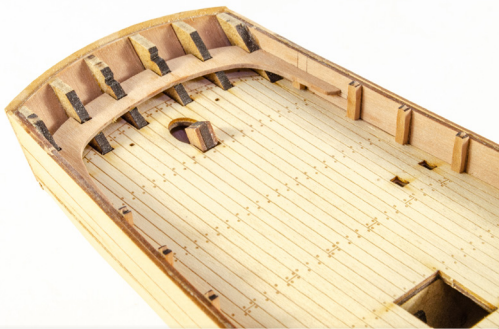
103. Glue this into position as seen here. This will sit into the notches on the stern timbers, and also on top of the short timberheads.
