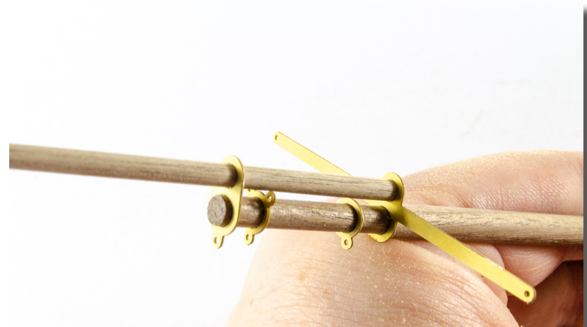
205. And here you see the assembled mast. There will be a small number of other PE parts to drill and fit to the mast.
