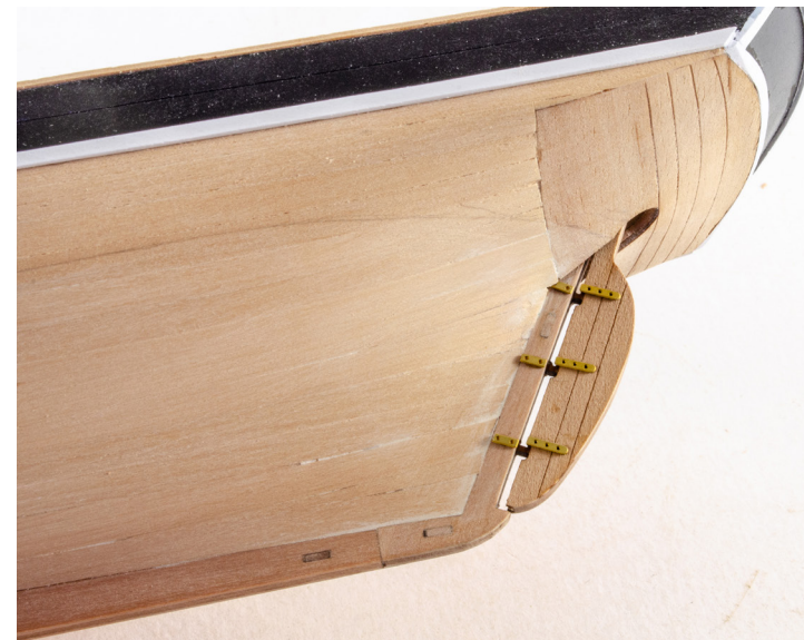
120. Glue the rudder to the hull. Now remove the six parts PE-17 from the PE sheet and glue on both sides of the rudder post, as shown here.
