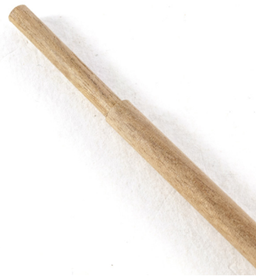
200. The lower mast section needs to be reduced in diameter towards the top.
