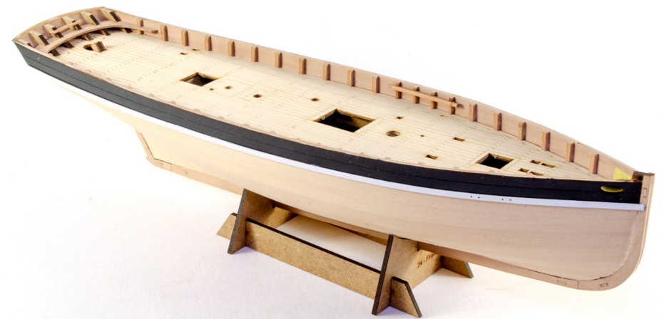
110. Using the lowest engraved line on the upper bulwarks, glue the rails into position directly underneath that line. You will need to bevel the front inner end a little, so it sits against the stem.
