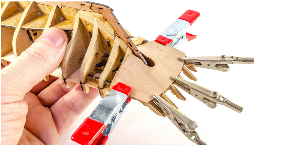
51. To make sure you get a good shape to this that matches your hull, soak the part in hot water for 30 mins and then clamp in place on the model. Leave this for over 12hrs to dry out as pear expands a lot when wet. It needs to be its original size when you come to fit it. Once dry, glue into position and leave to thoroughly set.
