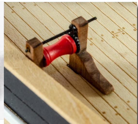
159. Slide the PE gear onto the thicker brass rod, followed by the drum, then glue the rod into #83. This will mean the engraving on part #33 is on the outside. Slip and glue the thinner rod into the wooden part, first locating through the small gear on the PE part. Lastly, fit the opposite wooden side.
