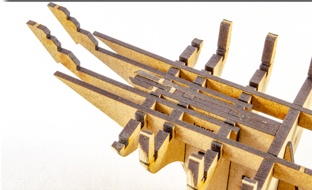
34. Dry fit (no glue) both parts at the stern, as shown. They will fit into the first series of bulkhead slots, adjacent to the parts you just fitted.
