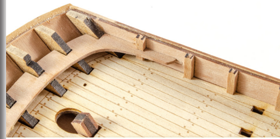
104. Now glue the top parts of timberheads 'U' into place over the part you just fitted.
