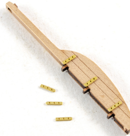
119. From the PE sheet, remove the six parts PE-18. These are the rudder hinges. Use CA to glue them into position on the engraved marks on both sides of the rudder.
