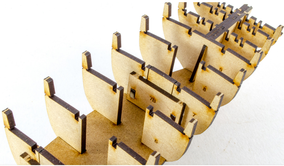
29. Now do the same for bulkhead #7, whilst fitting part 7a from the 3mm MDF sheet into the middle of bulkhead 7.
