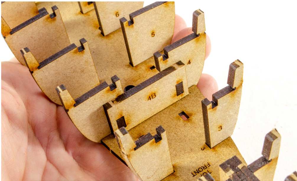
26. Using two of the pegs (13), glue 4b into position on one side of bulkhead #4.
