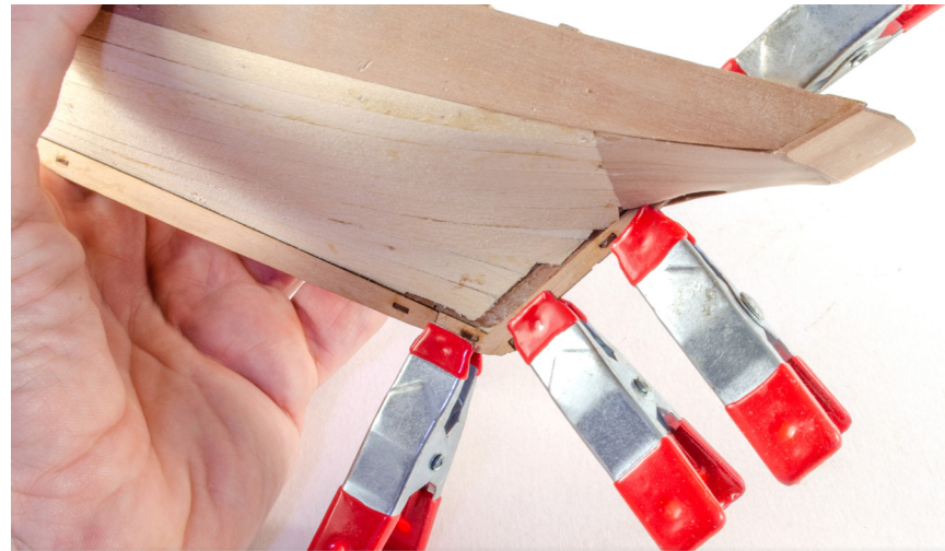
76. Once you are happy to fit the part, glue into position and clamp. When set, add the locating pins and glue part #57 into place on the opposite side of the model.
