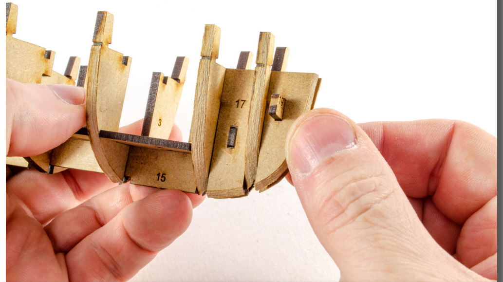
20. With both parts 17 in place, glue the locating pegs through the holes to ensure correct alignment. The locating pegs are parts 19, found on the 2mm MDF sheet.
