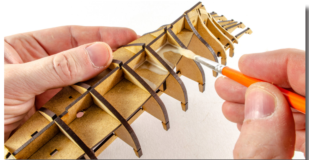
39. Make sure all parts are pushed into position and then paint dilute wood glue around the various joints and slots. Set aside to thoroughly dry.
