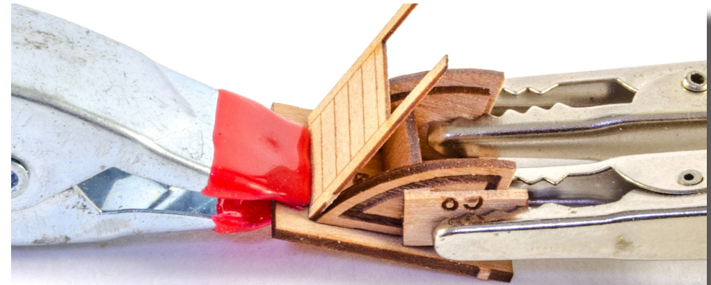
144. From the 0.6mm wood sheet, remove part #37. Two are provided in case you break one. Glue the read edge of this part into position as shown, using a clamp to stop it moving. Leave to dry. Note that I have used croc clips to hold the assembly to the jig, with slivers of wood to protect the outer, engraved sides.
