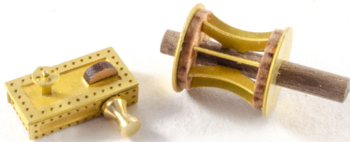
177. Your steam winch assemblies should look like this.
