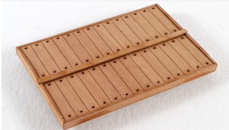
109. Remove the frame and sidewall assembly from the deck and glue the Fish Hatch Top Pattern (part 51) onto the assembly and then the Fish Hatch Front Centre Beam to the top as shown.
