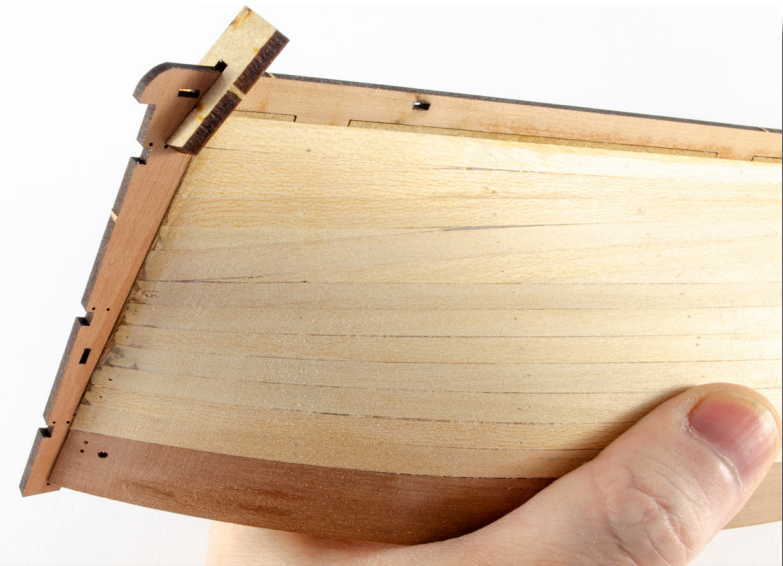
54&55 Using keel alignment clamps, part 25, clip the various keel sections to each other to help keep the various parts upright and square.
