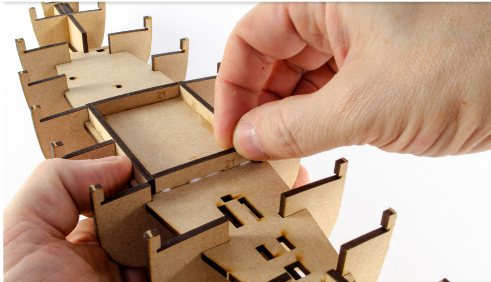
23. Both part 21 pieces must now also be glued into place. As we mentioned before, these also have different tab lengths, so check this before gluing in position. When installed, leave the glue to thoroughly set.
