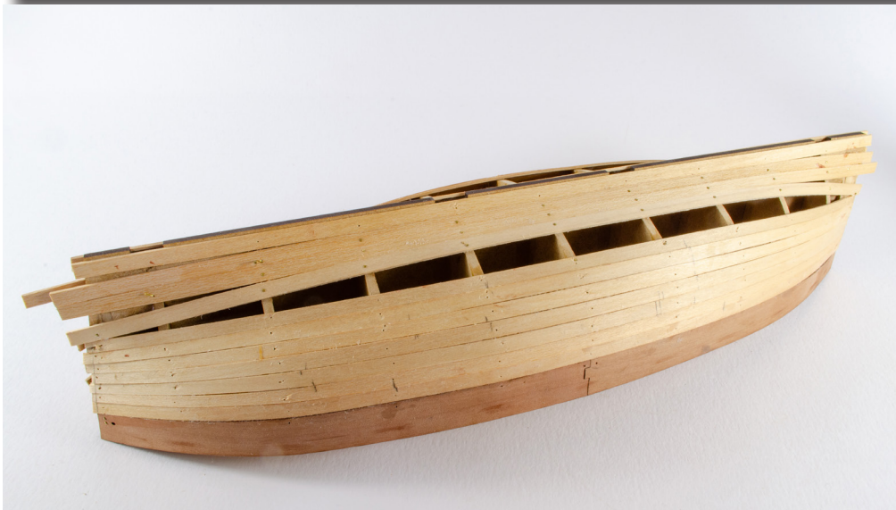
45. It won't be long before you notice that it becomes difficult to add the next plank along the edge of the previous. Here you must run the planks in the most natural way you can, as this picture shows. There will be gaps which we will fill a little later on.
