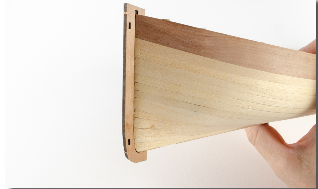
50&51 Make sure that the slot between the bulwark ends is wide enough to accept the Prow, part 26. If not, slightly open it up with a file or a knife. You shouldn't need to remove much material. Take the Prow and glue it firmly in position.
