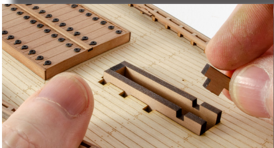
114. Now take the Foremast Opening End (part 32) and glue into its slot in the same channel, nearest the fish hatch. Lastly, glue the Foremast Securing Chock (part 33) into the notches between the two side parts.
