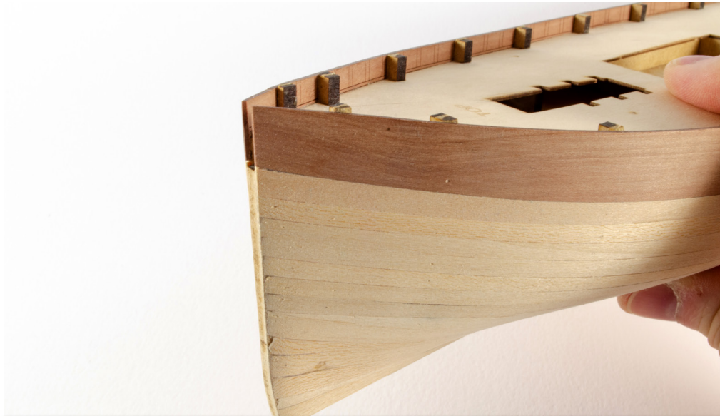
48. Ensure you finish the planks neatly at both stern and bow. This is how those edges should look
