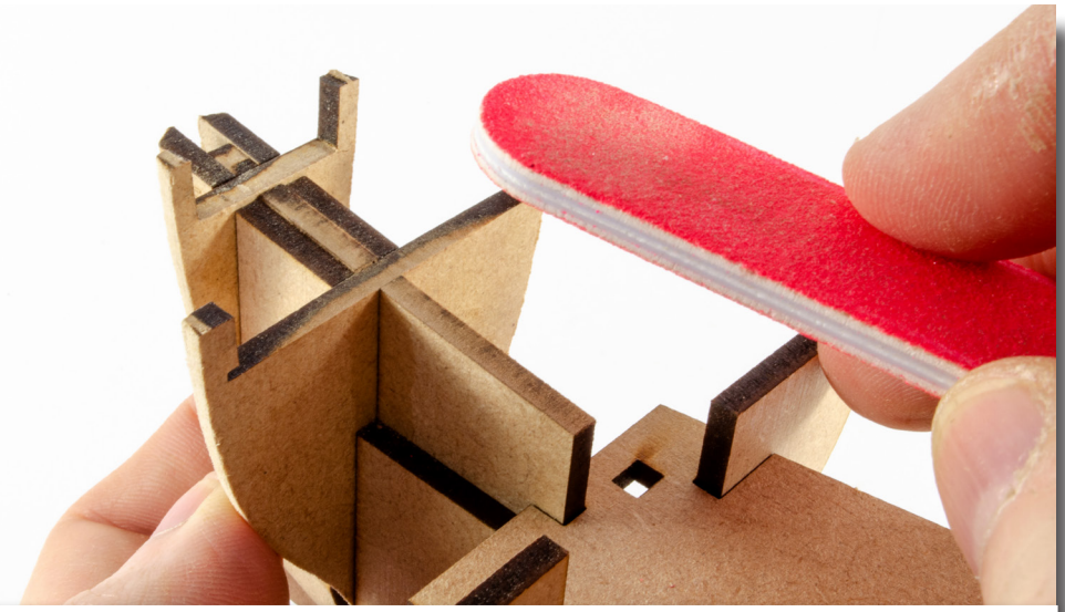
24. The line of the deck sweeps down from the stern and then upwards towards the bow. This is called the 'sheer'. Take a piece of sandpaper or a sanding stick and make the top of bulkheads 10 and 11, flush with the false keel.
