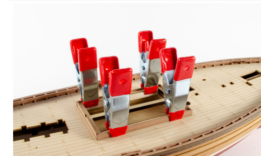
108. Glue the Fish Hatch Side Faces (parts 56) to the frame and clamp until dry.
