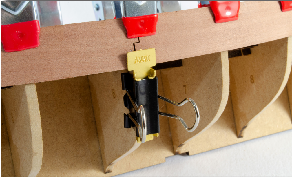
35. If you have a clamp like the Amati one shown, then these are ideal for temporarily pinning down the bulwark at the bottom edge until the parts have dried out.
