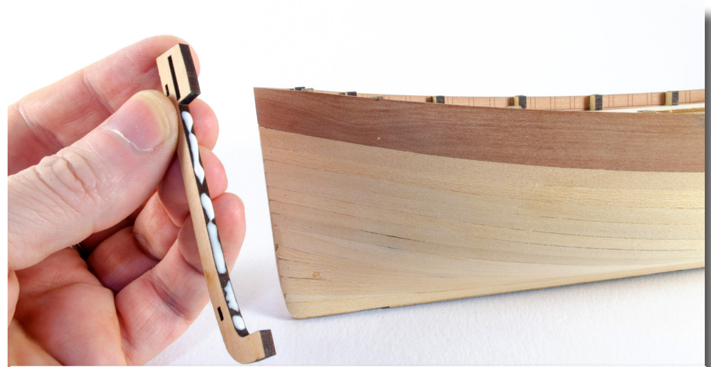
50&51 Make sure that the slot between the bulwark ends is wide enough to accept the Prow, part 26. If not, slightly open it up with a file or a knife. You shouldn't need to remove much material. Take the Prow and glue it firmly in position.
