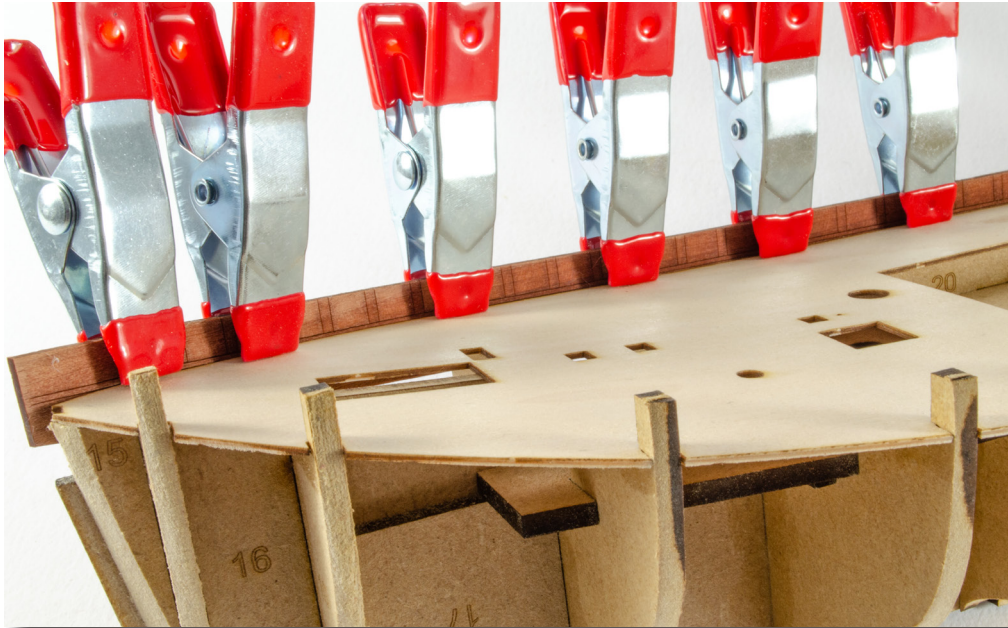
36. Once the parts are thoroughly dry, you can remove them from the hull. It's best to leave them for several hours to ensure this. The parts will spring back a little, but the majority of the curve will remain.
