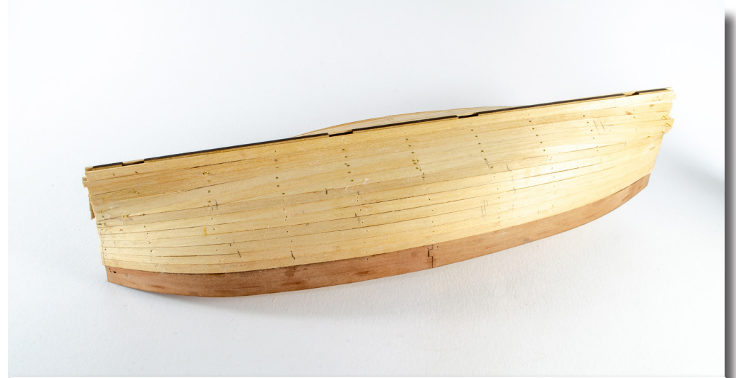
46. Don't be worried about those gaps. The infill pieces are what are known as 'stealers'. The pencil marks you see on the hull give an indication of the extent of the plank tapering.
