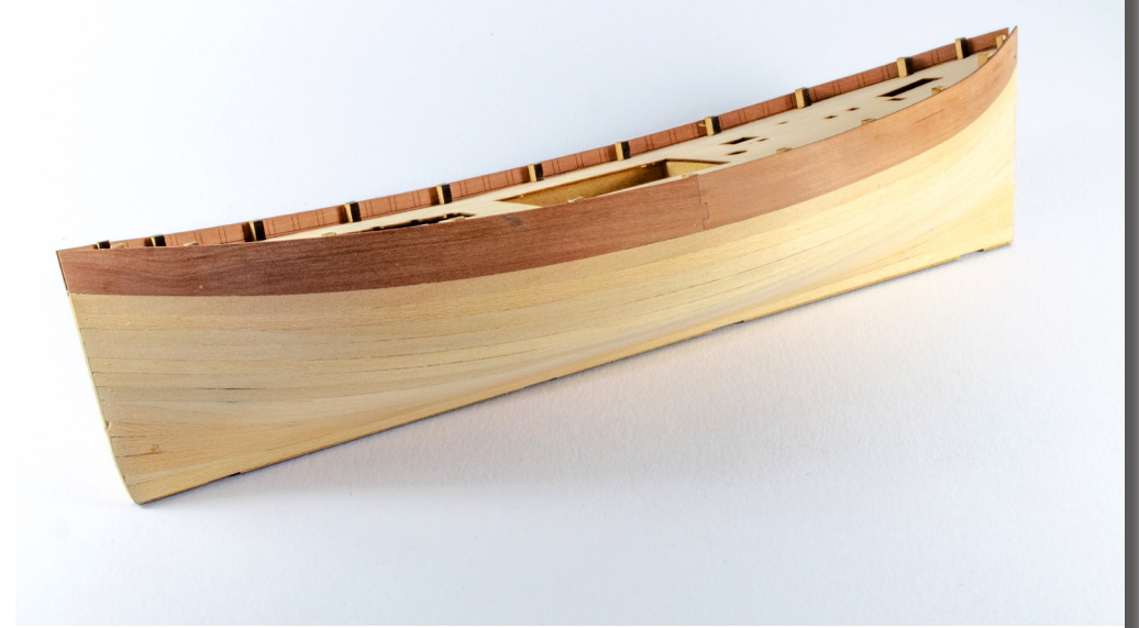
47. Using a piece of 80 or 120 grit abrasive paper, sand the hull smooth. Don't sand all the way through the planks though as this will be your base for the next layer.
