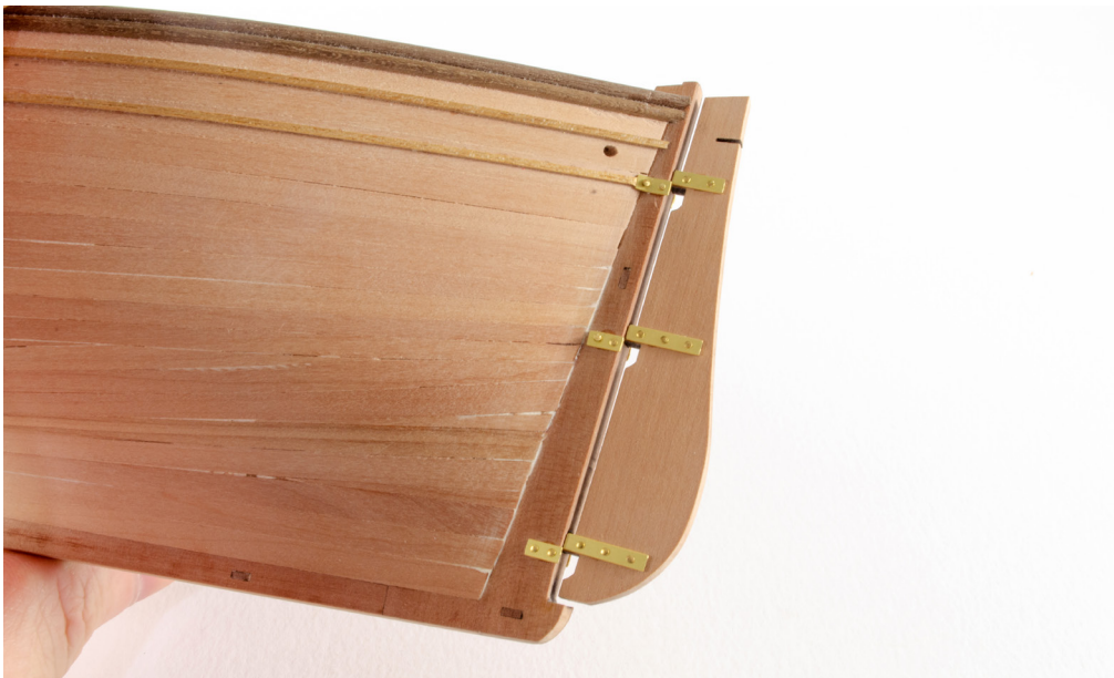
82&83 Remove the rudder straps/rudder post (parts PE5) from the photo-etch sheet and clean them up. Using the same technique as the rudder, place these into position on the stern keel post. You may need to slightly bend the upper parts if up next to the hull. Do not glue the rudder into position yet.
