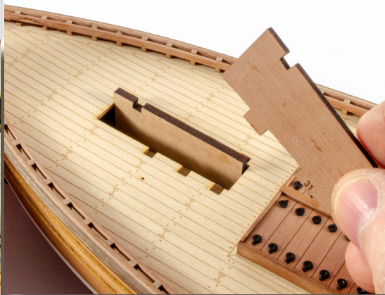
113. Remove the Foremast Opening Side parts from the 3mm Pear sheet (parts 31) and glue them into position as shown here.
