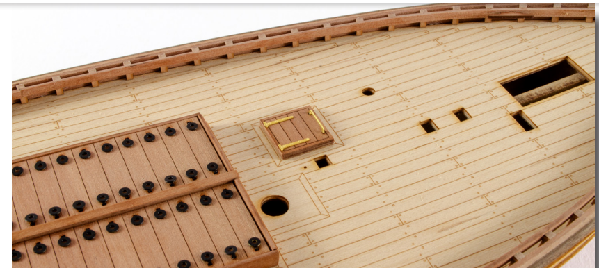
118, 119&120 Remove the Deck Hatch Combing (part 69) and the Deck Hatch Lid (part 70) from the 1mm pear sheet. Also remove two Door Hinge (PE-7) and a Hatch Handle (PE-6) from the photo-etch sheet and assemble as shown. Install the finished unit to the deck in the correct orientation.
