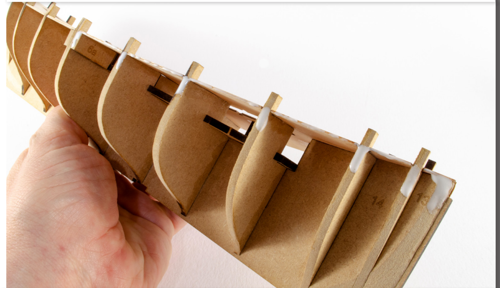
37. We can now fit those bulwark parts. Using wood glue (PVA, Titebond etc.), add glue along the edge of the deck and the bulwark, but NOT above deck height as we don't want those ears to be glued to the bulwarks.
