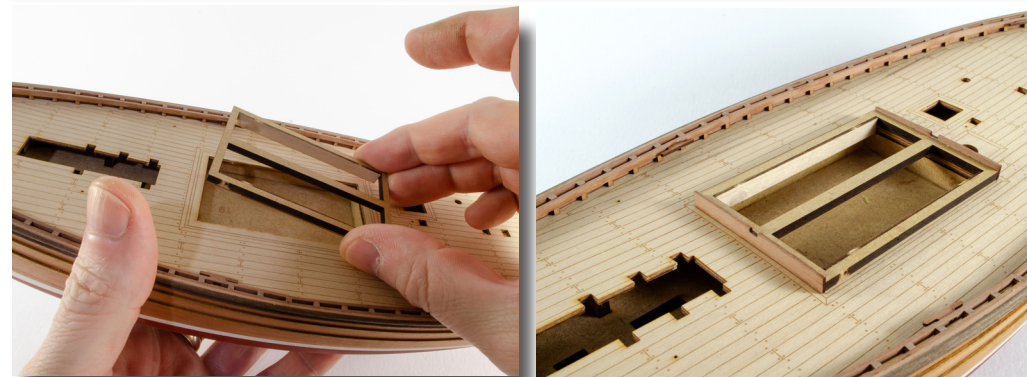
106&107 Dry fit the frame to the upper deck (no glue!) and glue the Fish Hatch Front and Rear Faces (parts 55) to the front and back of the frame. Make sure you don't get any glue on the deck.
