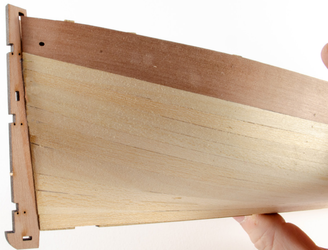
52. Now do the same for the stern post, part 29. This is how it should look when fitted.
