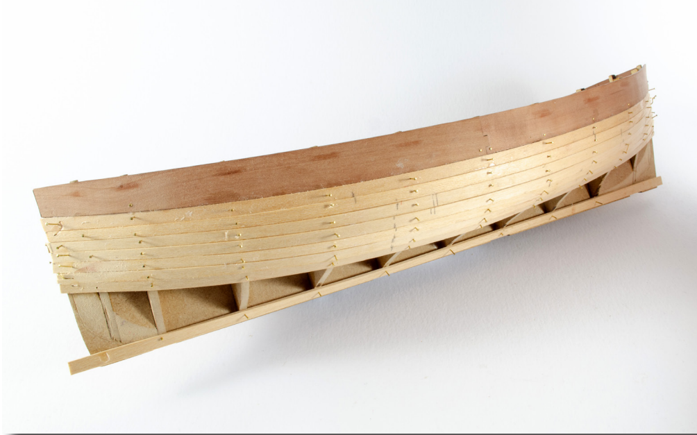
46. Don't be worried about those gaps. The infill pieces are what are known as 'stealers'. The pencil marks you see on the hull give an indication of the extent of the plank tapering.
