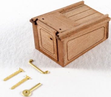
145. Remove parts 65, 66, and 67 from the 1mm pear sheet and glue into position as shown. Now remove the photo-etch parts PE-1, PE-6, and PE-7.
