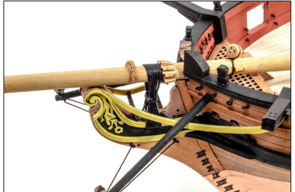
483. Add the gammoning as per plan sheet 1 & 2. Also add the bobstays.
