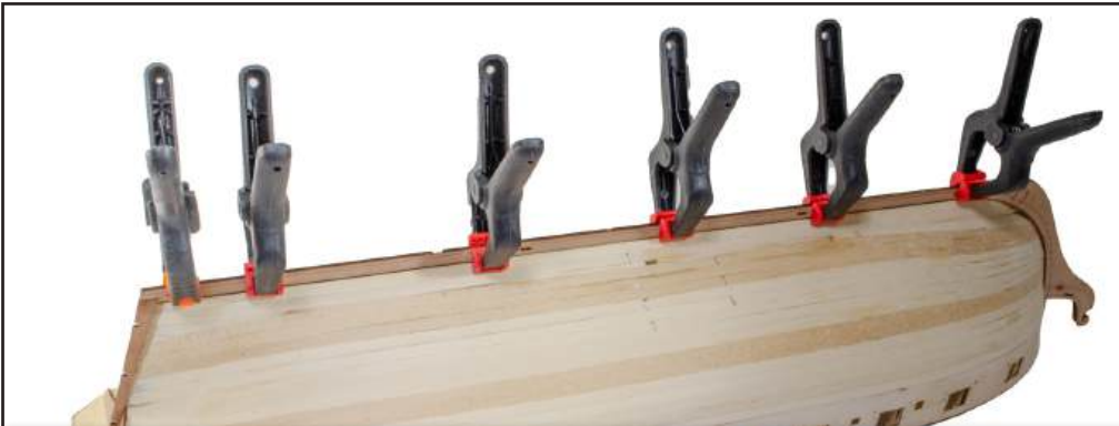
129. Fit these along the keel, as shown here, in the same manner as before. You will need four pegs K3 to help with alignment.
