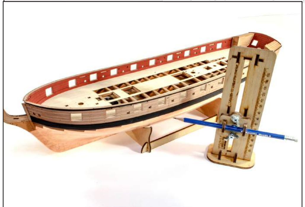
194. Sit the hull in the cradle, making sure the pin in the rear former sits into the hole in the underside of the keel. This makes sure your model is at the right attitude for a waterline to be marked. Use a waterline tool and lightly mark the waterline with the pencil. Check the position of this from the plan and ensure that the tool is at the correct height at bow and stern before you mark.
