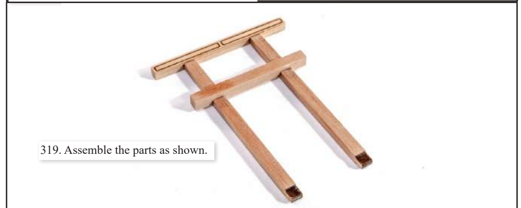
318. Assemble posts 264 with the beam 265 sitting into the slots. Ensure the assembly is 'square'. Also assemble the top of the gallows as with the previous gallows you just fitted.
