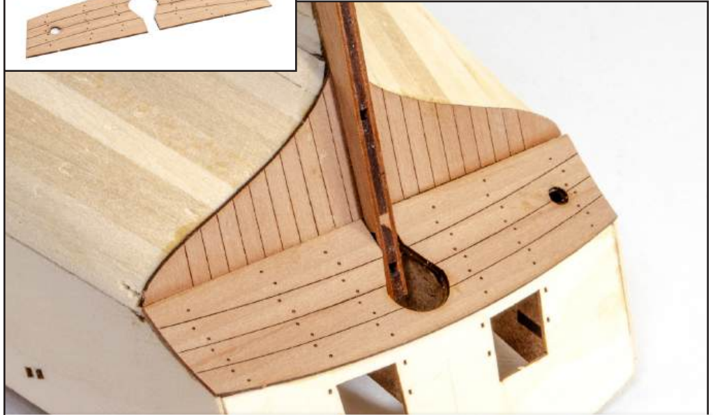
133. Glue part 110 into place as shown. This should naturally sit centrally due to the rudder post parts you just fitted, and the water closet hole on the left should align with the one in the ply level below. There isn't too much of a curve here, so you can just glue and hold this until it dries so you won't need to make pin marks in it. Sand the overhang of this part flush on both sides of the hull.
