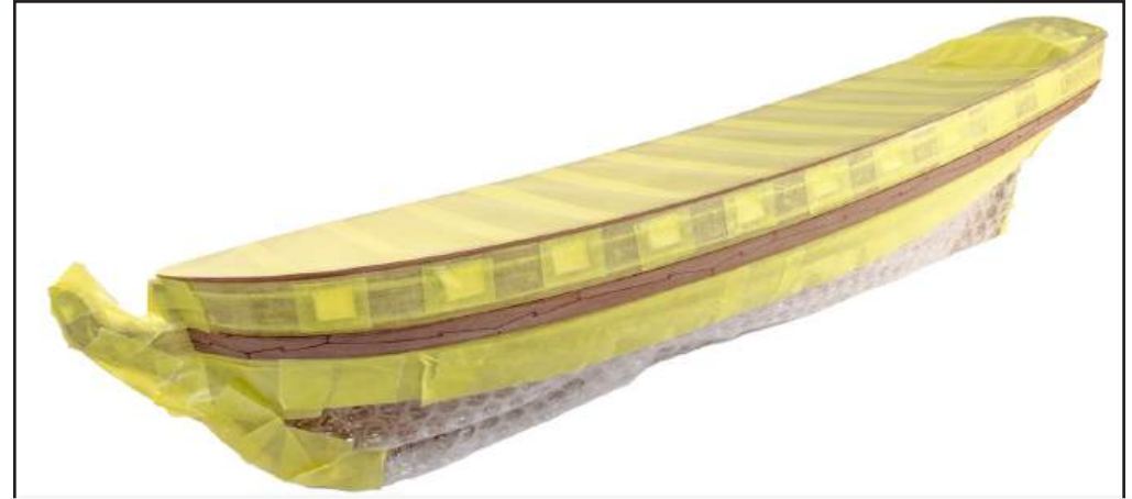
184. The wales and upper strip now need to be painted black. To do this, we masked the rest of the hull and used an aerosol for the black paint.
