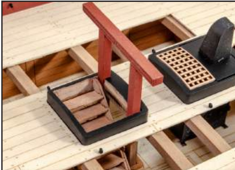
316. This can now be painted red and fitted through the openings in the corner of the fore ladderway, making sure that it plugs into the corresponding holes in the lower deck. NOTE: You only need to paint this assembly red from above the upper deck.
