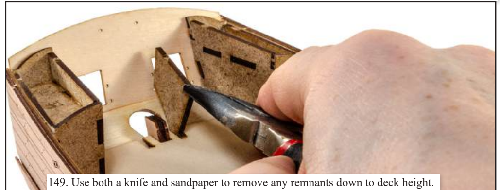
148. Using pliers or a suitable tool, twist off the MDF bulkhead ears above deck height. Also remove the two parts against the inner stern counter.
