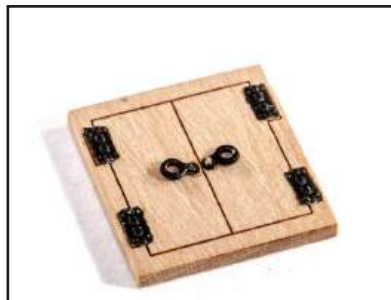
257. From the 1.5mm wood sheet, remove part 200. From the 0.4mm PE sheet, add two eyelets for handles. From the 0.2mm PE sheet, add some hinges PE-8.
