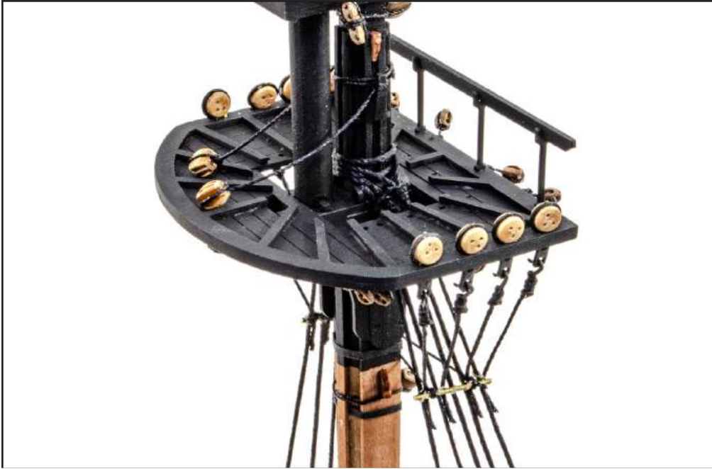
476. Add the 3mm deadeyes to the mast tops and then rig the futtock shrouds into them as shown on the plan.
