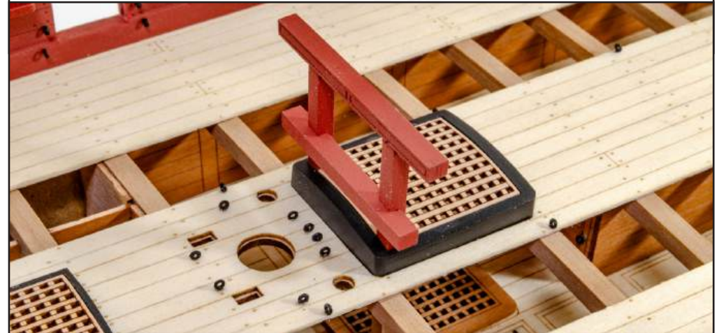
320. This should now also be painted red above deck height, and glued into position as shown, ensuring the bottom of the gallows plugs into the corresponding holes in the deck below.
