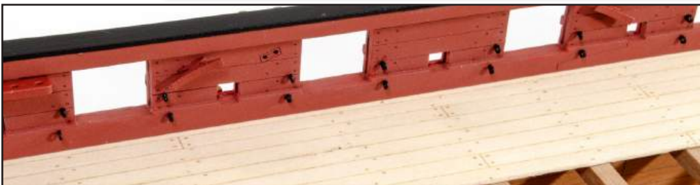
254. Now fit them along the inner bulwark as per plans. From the same 1.5mm wood sheet, remove all parts 218 and 219. These are the inner bulwark cleats. Paint them red and attach as per plan.
