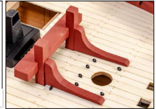
327. Glue those parts to the bitts as shown. A tip is to dry fit the bitts and then glue parts 266 against them to achieve the correct position. You can then remove the assembly, paint it red, and then glue into position as shown.
