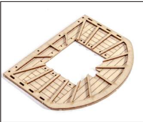
423. Glue together as shown, clamping until set. This is the main mast's 'mast top'.
