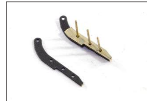
359. Sandwich one part PE-28 between two parts PE-27, using pins to align the parts and superglue to secure the parts.
