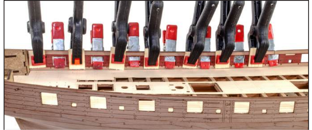
159. Now do the same for part 90R, seen here after gluing and clamping. You may need to trim this slightly at the rear so that it fits flat along the whole length.
