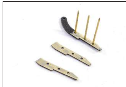
358. From the 0.4mm PE sheet, remove parts PE-27 and PE-28. You will also need a few brass nails.
