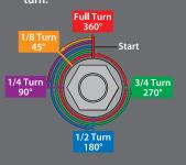
Do not run your model with the slipper clutch adjusting spring fully compressed. The minimum recommended slipper clutch setting is 1/2 turn counterclockwise from fully compressed.
