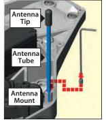
antenna wire is in the slot in the antenna mount, then install the set screw next to the antenna tube. Use the supplied 1.5mm wrench to tighten the screw just until the antenna tube is securely in place. Do not over tighten. **Do not bend or kink the antenna wire! See the** sidebar for more information. **Do not shorten the antenna tube**.
