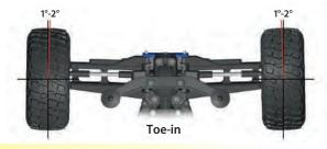
Toe Base Factory Settings Front: 0-degrees Rear: 2.5-degrees toe-in each side
