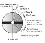
Important: Do not lean the high-speed mixture less than 2 turns out from closed (see illustration). Also, be sure to allow the engine to cool between each run.
