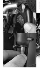
Remove the 4mm locknut from the front pipe hanger. Pull the pipe from the rear exhaust header. STEP 1:
