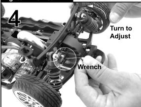
With the diff screw & outdrive locked together with the 1/16" allen wrench tighten (about the same as a top on a jar) by turning the right rear tire toward the front of the car.
