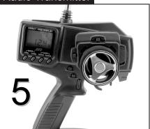
Turn on the transmitter and check the display for adequate power.
