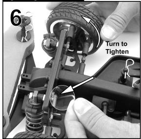
Lock the diff screw & outdrive together with the 1/16" allen wrench and tighten (about the same as a top on a jar) by turning the right front tire towards the front of the car.
