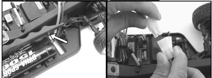
Install the battery pack into the car with the wires at the front. Note the tab on the battery strap that goes behind the edge of the pack. Secure with clips at front and rear. Note that the plugs are made so they can only be plugged in one way.
