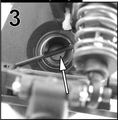
Insert 1/16" allen wrench thru slots in outdrive & diff screw to lock together.
