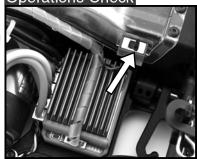
Switch on the car and check for correct operation before running. NOTE: The speed controller is preprogrammed and ready to use.
