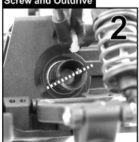
Line-up the slot in the diff screw with the slots in the outdrive - (the drive shaft has been removed for photos.)
