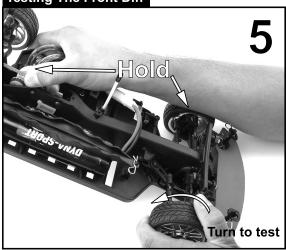
Try turning right front tire toward the rear of the car while holding the left front tire and spur gear.
