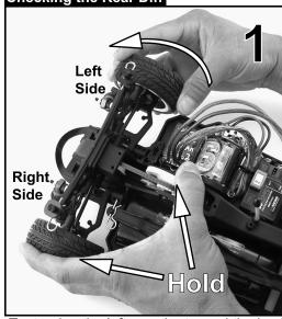
Try turning the left rear tire toward the back of the car while holding the right rear tire and spur gear.
