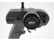
6. ALWAYS turn on the transmitter first by sliding the switch "ON". The small red and green lights above the switch should both light up. If not, please check for low or incorrectly installed batteries.
