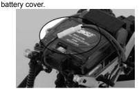
**4.** Plug in the battery lead into the speed controller lead and replace the body.
