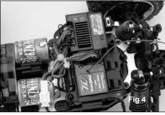
Once the battery is charged, remove the body clip from the front of the battery tray (fig. 2) and lift up the front of the tray (fig. 3). Install the battery pack as shown (fig. 4), reinstall the body clip and plug the battery pack into the ESC.
