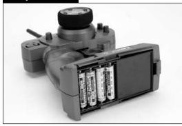
Remove the transmitter battery cover by sliding the cover from left to right. Install four (4) AA batteries into the battery holder. Pay close attention to the correct direction of the positive (+) and negative (-) ends as marked in the tray. Once all four batteries have been installed, reinstall the battery cover by sliding it on from right to left.
