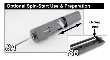
Slide the battery access panel opposite the hand strap back and remove the cover. Remove hex starter shaft from the back side of the cover (fig. 8B) and press the O-ringed end into the drive cup. Slide a charged 7.2-volt 6-cell "stick pack" (not included) into the Spin-Start and plug it in. Note that the plug is made such that it can only be plugged in one way. Carefully tuck the plug wires under the battery access panel and slide shut.
