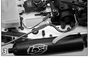
The Limited Edition Aftershock includes a 6-volt rechargeable battery pack. This needs to be charged before running. Follow the charger manufacturer's instructions to charge it with a preferred charge rate of no more than 1 amp.
