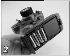
Install the 4 AA-size alkaline batteries in the transmitter making sure the positive (+) and (-) negative ends are oriented correctly. Use only quality alkaline or rechargeable NiMH (nickel-metal hydride) AA size cells.
