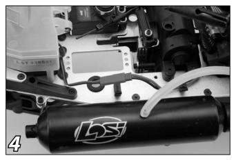
After the receiver battery is charged plug the red plug from the battery into the mating red plug that goes into the radio box. Note that the plugs are constructed so they will only fit one way easily. Use the black plastic clip on the chassis to secure the wires so they do not touch any of the hot or moving parts.
