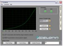
Below is an example of an accelerated ramp up to full throttle.
