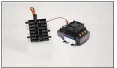
The Xcelorin 8th Quick Programming Card (8QPC) is used to make all adjustments to the active profile in your ESC. Any ACTIVE profile can be modified.
