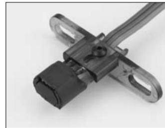
*Bracket adjusted for 90-size engine*
