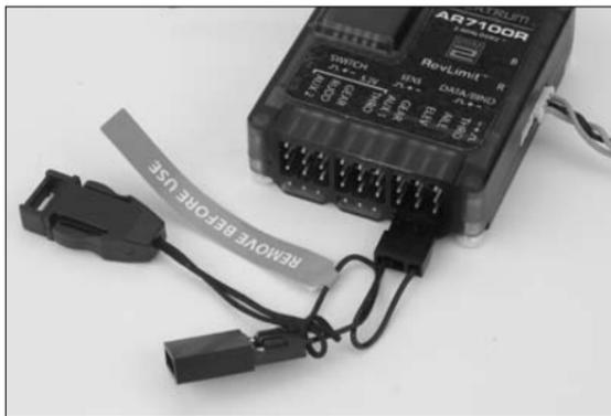
2. Turn on the soft switch. Note that the LEDs on all receivers should be flashing indicating that the receiver is ready to bind.
