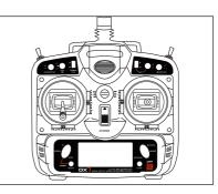
Press and hold the bind button on the back of the transmitter while turning on the transmitter. The button will flash for several seconds, then the LED on the transmitter and receiver will remain solid on, indicating a successful bind.
