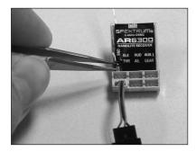
Power on the receiver. If the receiver is installed in an electric aircraft, turn on the speed controller to power up the receiver. If the receiver is going to be powered by a separate battery, plug the battery into any unused port. The amber light will blink, indicating the AR6300 is in bind mode.
