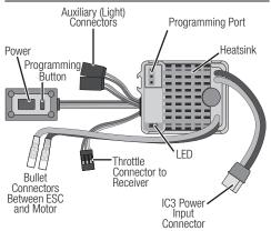
**NOTICE:** Always disconnect the battery from the ESC when you have finished operating your vehicle. If you leave the battery connected with the power switch in the OFF position, the ESC will continue to draw current when connected to the battery, resulting in possible damage to the battery through over-discharge.
