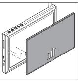
2. Open the clamp on the front of the Headset Adapter and set the monitor into the Headset with the screen facing in.
