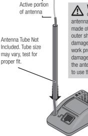
WARNING: Do not kink, **CLL** cut or damage the antenna wire. The antenna is made of a coaxial wire: if the outer sheath becomes damaged, the receiver will not work properly. If the antenna is damaged in any way, replace the antenna before attempting to use the receiver.
