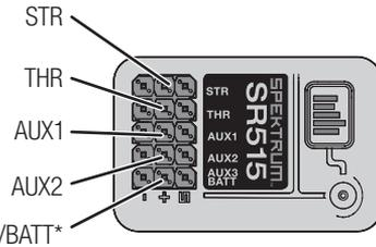
**\*IMPORTANT:** AUX 3 on the SR515 shares the servo port with the battery. A Y harness (SPMA3008) is required on the AUX 3 port to use all 5 channels with a receiver battery.
