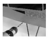
2. Drill hole for insert. Drill slightly under sized to assure snug fit.
