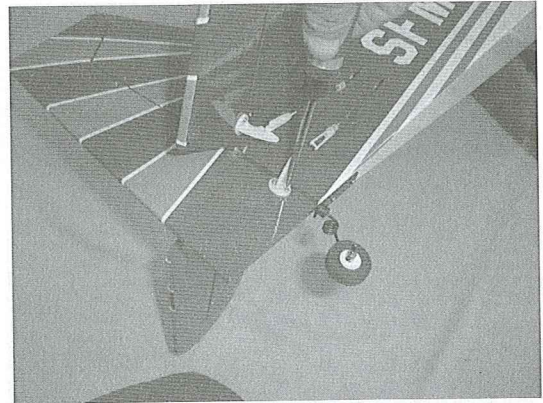
Repeat the same procedure to attach the rudder control horn on the rudder.
