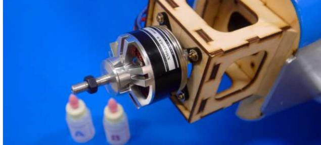
Use Epoxy to secure the motor mount on the fuselage and reinforcing blocks on two sides of moor mount.
