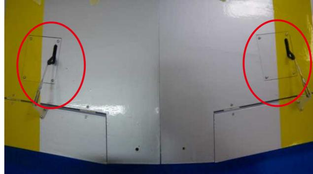
If use Y-harness on the flap, please install the left wing and right wing servos at the same side. If want to use mixer on the radio, the location of both servos must be on different side.
