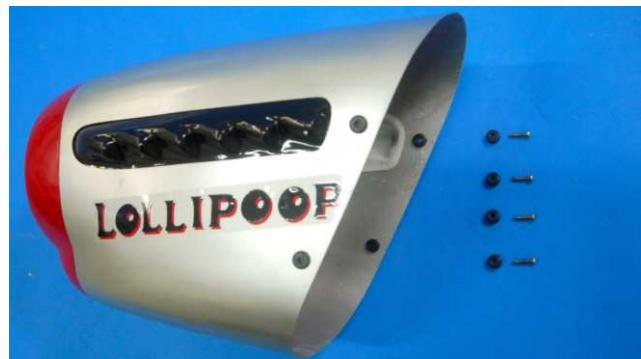
Installing the anti-vibration rubber inside the cowl. Try to fit the cowl to the motor or engine. When satisfy the location, use M2.6x12 tapping screws to secure the cowl in position.
