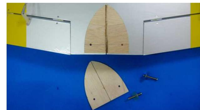
Place the main wing upside down. Take the reinforcement planking out of the hardware bag. Try to place the planking along the trailing edge and set its center line on the center line of main wing. Use screws to hold the planking in place for temporary.
