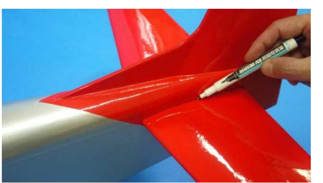
Remove the elevator out of the horizontal. Trial fit the horizontal in place on the fuselage. Please note the distance to the tip of the horizontal must be equal on both sides. Please refer to the last drawing. When you are satisfied with the alignment, use marker to carefully trace around the top and bottom of the horizontal where it meets the fuselage.
