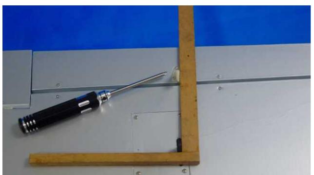
Place the triangle rule along the servo arm to the trailing edge for setting the location for installing the control horn on the aileron. Use 1.5mm hand driller to drill holes for the control horn. Place the control horn in position and the strap on its back and secure with M2x25mm screws.
