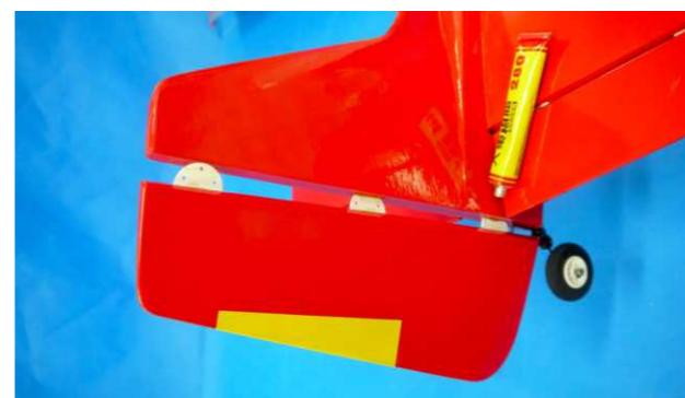
Spread Super glue on the one half of hinges and insert the hinges to the hinge slots on the rudder. Spread Super glue on the other half of hinges and insert the hinges to the slots on the vertical.
