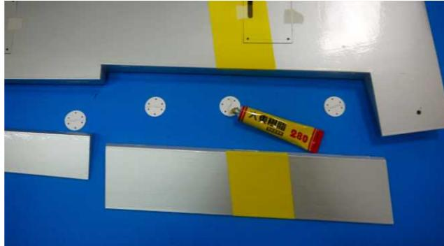
Spread some Super Glue on the top and bottom one-half of each hinge. Insert the hinges into the main wing until the hinge line is even with the trailing edge of the main wing.
