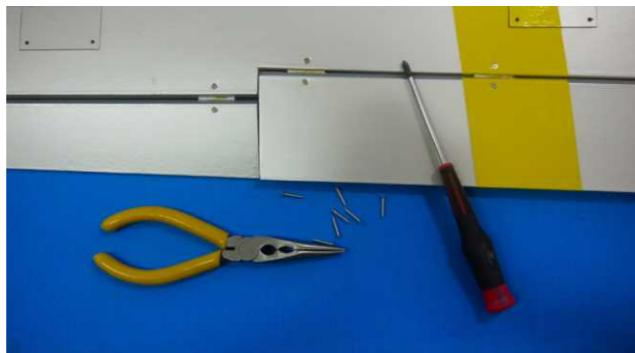
Spread some Super Glue to the remaining half of each hinge and place the aileron and flap onto the main wing. Secure the hinges with 2x15mm tapping screws. If the end of the screw is too long, use side-cutter to trim the end.
