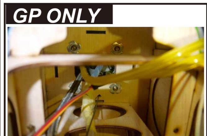
Push the claws nails to the holes inside the fuselage. It's better to use the engine screw M4x30 hex screw to secure the claws nails hard into the planking. Drop instant glue around the claws nail for securing it in place. Don't let the instant glue touch the screw.
