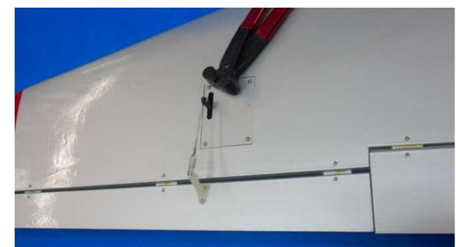
Thread the clip to the rod. Slide one piece of 5mm silicone tube to the connection of the control horn and clip. Use Z-bender to make a Z bend on the rod for connecting with servo arm.
