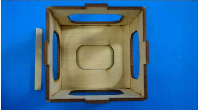
Use wood glue to secure the reinforcing block on the bottom of motor mount. Spread Epoxy on every corner for reinforcement.
