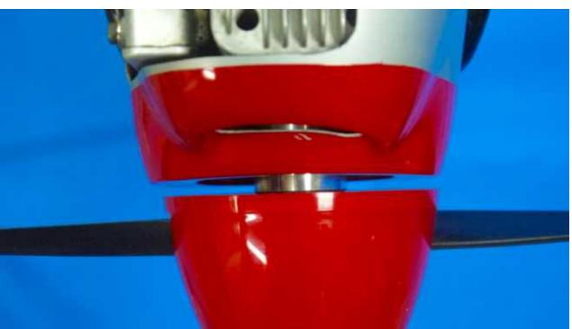
Assemble the spinner with propeller. Install the spinner to the motor. Please keep the distant between spinner and cowl around 2mm.
