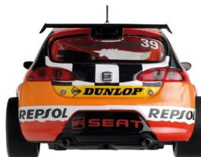
The tilting of the motor-rear axle assembly also works actively to stop you coming off the track in circumstances when it would be unavoidable with any other chassis. You need to accelerate at the right time; skids are short and impulsive, and the car tends to follow the slot pretty well.
