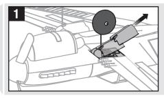
2. Lift the end of the landing gear wire above the stop.
