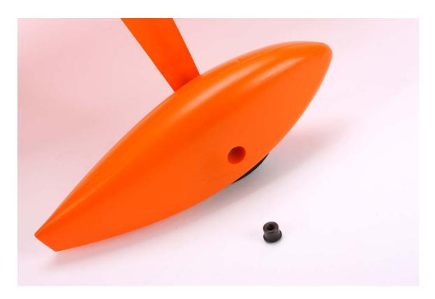
2. Apply a small amount of thread-lock to the inside of the wheel nut.
