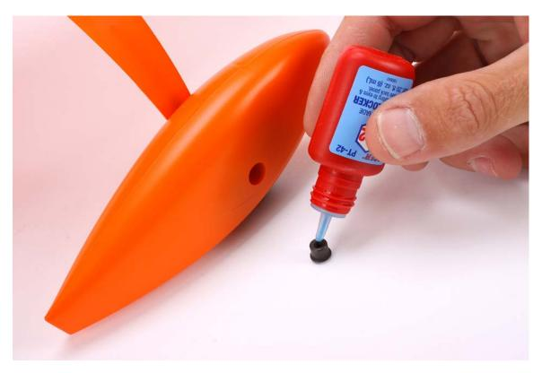
$3. \;\;$  Install the wheel nut and allow the thread-lock to thoroughly dry.
