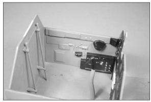
☐ 4. Prepare the headrest by trimming the excess material around the headrest using hobby scissors. Glue a balsa block (not included) in the headrest so it can be attached to the headrest mount.
