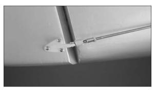
☐ 8. Center the tail wheel. Use side cutters to trim the cable so there are equal parts of cable for the steering inside the fuselage. Use the M3 x 4 setscrews to secure the wire eyelets in the pushrod connectors. Leave 3/8 inch (9mm) of the eyelets extending through the connectors. The screws only need to be snug at this time.
