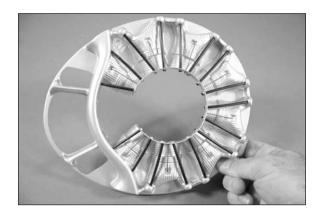
Remove only the amount of material shown. Removing additional material will only increase the pressure inside the cowling, causing the engine to overheat.
