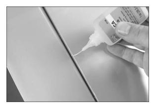
→ Do not use CA accelerator when gluing the hinges. Always allow the CA to soak into the hinge for the best bond between the hinge and surrounding wood.
