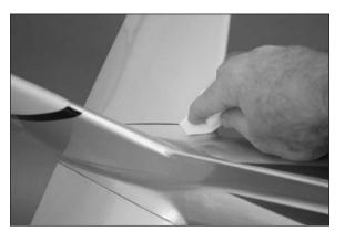
$\square$  12. Use a pin vise and 1/16-inch (1.5mm) drill bit to drill a hole in the center of the four hinges slots. Prepare both the elevator and stabilizer at this time.
