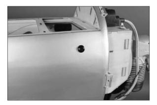
→ We added two short pieces of fuel tubing to the carburetor needles to help align the screwdriver during adjustments.
