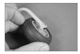
→ Remove the excess axle using a rotary tool and cut-off wheel. Make sure to remove the axle so the heat from cutting does not cause the tail wheel adapters to deform.
