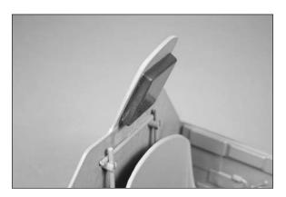
$\square$  7. Mount the cockpit kit in the fuselage using two 4-40 x 1/2-inch socket head cap screws and two #4 washers. The front of the cockpit keys into the former in the fuselage. Use a 3/32-inch hex wrench to tighten the screws.
