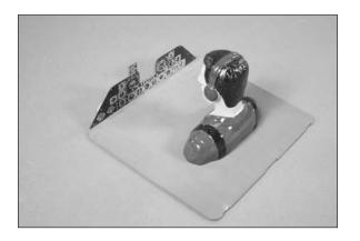
$\square$  3. Use medium CA to glue the cockpit floor into the canopy hatch. Allow the CA to fully cure before placing the canopy hatch on the fuselage.
