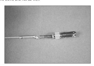
☐ 10. Attach the clevises to the middle holes on the steering arm, then slide the clevis retainers over the forks of the clevis to make sure they don't open accidentally. Check that the cables will not cross in the rear of the fuselage when the tail wheel is installed.
