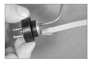
☐ 7. Place the stopper back in the tank. Use a #1 Phillips screwdriver to tighten the M3 x 20 machine screw to secure the stopper. Don't over-tighten the screw as you could damage the fuel tank. It needs to be tight enough to create a seal between the tank and stopper. Slide the fuel tubing onto the brass tubes outside the tank. Make sure to wire the tubing to the brass tubes so it will remain attached during the operation of your model.
