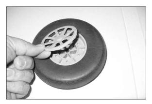
→ Place a drop of light machine oil on the axle before installing the wheel so they will rotate freely on the axles.
