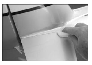
☐ 11. Apply epoxy to the stabilizer tube on the opposite side of the fuselage and the stabilizer as described in steps 8 and 9. Slide the remaining stabilizer into position and use a paper towel and isopropyl alcohol to remove any excess epoxy. Allow the epoxy to fully cure before proceeding.
