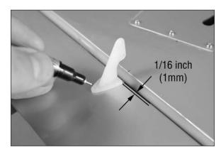
□□ 10. Use a drill and a 1/16-inch (1.5mm) drill bit to drill the three holes for the control horn mounting screws. The holes only need to be 3/8 inch (10mm) deep for the screws. Do not drill through the top of the aileron. Use a #1 Phillips screwdriver to thread an M2.5 x 12 sheet metal screw in each hole. Remove the screw and place 1–2 drops of thin CA in each hole to harden the surrounding wood. Attach the control horn using three M2.5 x 12 sheet metal screws and a #1 Phillips screwdriver.
