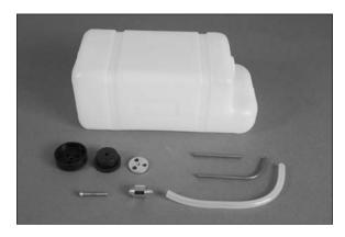
☐ 2. Use a hobby knife and #11 blade to remove the material so two of the three holes in the stopper pass completely through. Slide the straight and pre-bent brass tubes through the smaller stopper plate. Position the front of the tubes even with each other.
