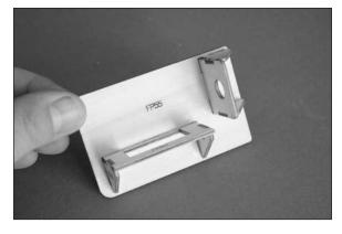
☐ 2. Prepare the retract servo by installing the brass eyelets and grommets. Position the servo in the tray and use a pencil to mark the location for the servo mounting screws.
