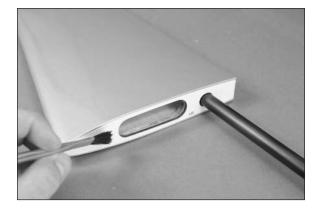
□ 9. Apply a thin coat of epoxy to the exposed wood of the fuselage. Also apply a small amount of epoxy to the smaller tubes installed in step 7.
