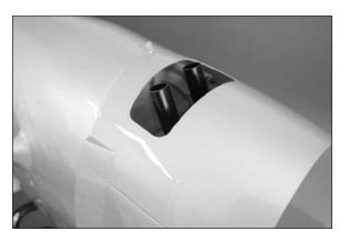
☐ 10. Enlarge the hole in the spinner backplate to fit the motor shaft. The recommended gas engine will require a 10mm hole, while the recommended E-flite® motor will require a 12mm hole.
