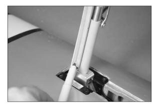
□□ 13. Remove the gear door. Place two pieces of low-tack tape where the stiffener will be positioned. Use sandpaper to roughen the area to provide a surface to glue the stiffener to the gear door. The tape will prevent removing the paint from the surrounding area. Once prepared, use medium CA to glue the stiffener to the gear door.
