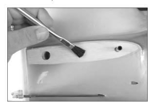
☐ 10. Slide the stabilizer into position, fitting it tightly against the fuselage. Use a paper towel and isopropyl alcohol to remove any excess epoxy before it can cure.
