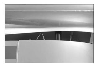
$\square \square$  3. Secure the wing using a 1/4-20 x 2-inch nylon wing bolt.
