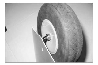
□□ 10. Secure the wheel using another wheel collar that will be flush to the outside edge of the axle. Tighten the setscrews using a 1.5mm hex wrench. Make sure to use threadlock on the setscrews to prevent them from vibrating loose. Install the hub cap back on the wheel once the setscrews are tightened.
