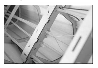
☐ 8. Prepare the cable ends in the tail wheel opening by passing the cable through a copper crimp, then through the hole in the 4-40 threaded eyelet. The cable then goes back through the crimp. Use crimping pliers to compress the crimp, securing the wire. Prepare one end of both wires at this time.
