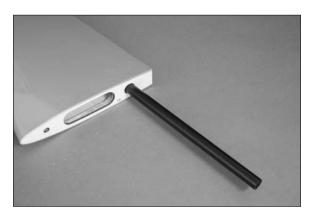
→ Make sure the stabilizers are mounted correctly. The top covering will overlap onto the bottom covering, which can be seen along the outside edge of the stabilizers.
