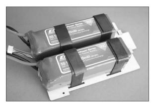
$\square$  10. The battery tray can now be installed in the fuselage. The front will fit under the tabs in the structure behind the firewall. The rear is held in position using two 4-40 x 1/2-inch socket head screws. The batteries connect to the speed control using a Y-harness.
