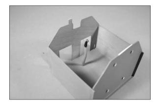
→ We drilled a small hole in the bottom of the stick and used a #2 x 1/4-inch sheet metal screw to secure the control stick to the cockpit floor.
