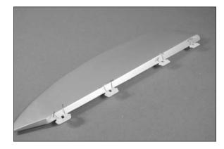
→ Make sure the elevators are mounted correctly, as there is a hardwood block installed in the bottom-side for mounting the control horn. The top covering will overlap onto the bottom covering, which can be seen along the outside edge of the elevators.
