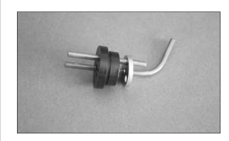
$\square$  3. Slide the plastic cap over the tubing at the front. Start the M3 x 20 machine screw using a #1 Phillips screwdriver. The screw only needs to be in far enough to keep the large stopper plate from falling off.
