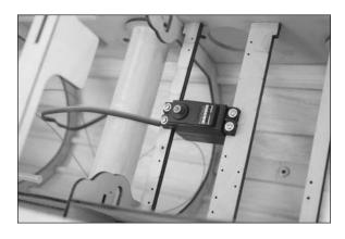
→ Should the laser cut holes not align with your servo, you will need to use a pin vise and 1/16-inch (1.5mm) drill bit to drill new holes to mount the rudder servo.
