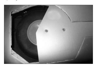
□□ 12. With the retract in the DOWN position, place the stiffener so it almost touches the landing gear strut. This is necessary so it will clear the surrounding structure. Use a felt-tipped pen to mark the location of the stiffener on the gear door.
