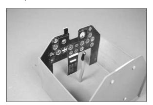
☐ 3. Fit the side panels in the cockpit. Once fit, use medium CA to glue the side panels into position. Glue the seat into the cockpit using medium CA. Position the seat so it is centered behind the control stick.
