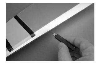
☐ 3. Place two T-pins in each of the three CA hinges as shown. This will center the hinge evenly between the rudder and fin when the hinges are installed.
