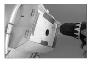
☐ 3. Use a drill and 7/32-inch (5.5mm) drill bit to enlarge the holes. Use four 8-32 x 1-inch machine screws, four #8 washers and four 8-32 blind nuts to secure the motor box to the firewall. Make sure to use threadlock on the screws to keep the hardware from vibrating loose.
