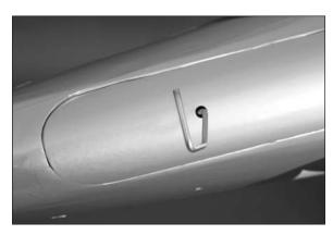
☐ 13. The cover is secured to the fuselage using five M2.5 x 12 sheet metal screws. Use a pin vise and 1/16-inch (1.5mm) drill bit to drill the holes. Use a felt-tipped pen to mark the position of the former on the fuselage so the screws can be located when they thread into the former. Use a #1 Phillips screwdriver to install the screws.
