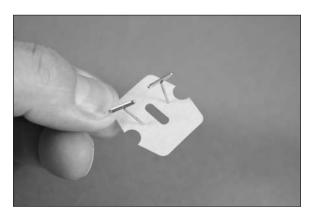
□□ 4. Insert the hinge in the aileron hinge slots. Center the opening in the center of the hinge with the hole drilled in step 2. The T-pins will rest on the leading edge of the aileron when the hinge is installed. Install all three hinges at this time.
