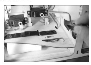
☐ 4. Connect the leads to the receiver, including the 18-inch (457mm) extensions for the flaps and ailerons and the switch harness for the receiver battery. When using dual receiver batteries, connect the switches to a Y-harness, then the Y-harness into the battery port of the receiver. Wrap the receiver in 1/4-inch (6mm) foam and secure it to the plywood receiver tray using a hook and loop strap. Use medium CA to glue the plywood receiver tray to the servo mounting rails.
