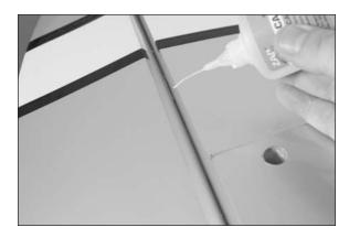
→ Do not use CA accelerator when gluing the hinges. Always allow the CA to soak into the hinge for the best bond between the hinge and surrounding wood. ☐ 7. Once the CA has fully cured, check that the hinges are secure by gently pulling on the control surface. If not, apply thin CA to any hinges that are not glued and recheck. Move the control surface through its range of motion several times to break in the hinges. This will reduce the initial load on the servo during your first flights.
