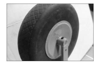
□□ 7. Check the operation of the retract. You will find the wing rib requires slight trimming toward the leading edge to clear the wheel and allow the retract to lock in the UP position. This is necessary as the assembly of the wing can not be accomplished if the rib is trimmed to fit the wheel during production.
