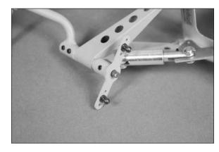
☐ 8. Attach the tail wheel by inserting the correct adapters in the wheel to match the diameter of the shaft. The shaft goes through the wheel, then into the tail gear. Secure the axle using the setscrew in the gear.
