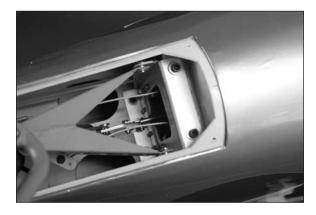
→ We recommend taping the air lines to a pushrod tube to keep them from falling back into the fuselage.
