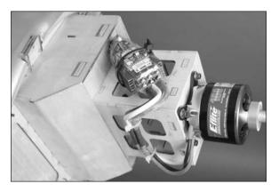
☐ 6. Assemble the battery tray support using medium CA. Note the position of the slot in the rear support, as it must be positioned correctly to fit over the fuel tank stop inside the fuselage. Also install the two 4-40 blind nuts using pliers. Place a drop of thin CA on the prongs of the blind nuts to keep them from accidentally falling out, making sure not to get CA in the threads.
