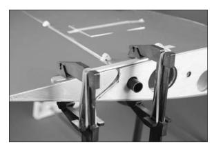
□□ 10. Once the epoxy has cured, remove the tape and clamps. If any of the flap hinges (only the flap hinges) appear to be loose, apply thin CA to the hinge where it enters the flap and wing to complete the flap hinging process.
