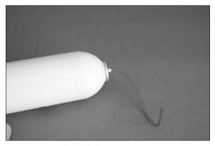
☐ 12. Place a drop of silicone adhesive on the air tank. Slide the tank into the fuselage. It only takes a small amount of adhesive to keep the tank in the fuselage.
