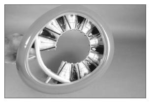
$\Box$  4. Fit the cowling over the engine. Use a rotary tool with a sanding drum to slowly remove the material from the radial engine so it fits over the carburetor. Once fit, use six 4-40 x 5/8-inch socket head cap screws and six #4 washers to secure the cowl to the fuselage. Use a 3/32-inch hex wrench to tighten the screws.
