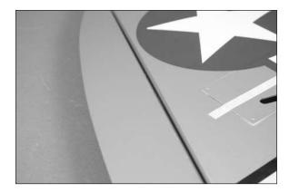
□□ 6. Prepare the three pinned hinges by applying light machine oil to the hinge point. This will help prevent the adhesive from entering the hinge and causing it to not move.
