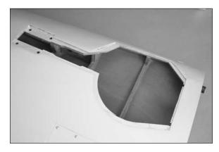
□□ 3. Cut a piece of red and purple air line to a length of 15 inches (381mm). Place a quick disconnect on each line. Make sure to use one connector with the O-ring and one without to avoid connecting the lines incorrectly. Guide the air lines through the openings in the wing from the root to the retract mount. Fittings have been installed to route the air line so it doesn't interfere when the retracts are in the UP position.
