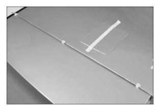
□□ 8. Once satisfied with the fit, note the position of the hinges. Remove the flap and hinges. Mix a small amount of 30-minute epoxy and glue each hinge into position in the flap and wing. Use a toothpick to apply epoxy in both the holes for the hinges and to the hinges themselves.
