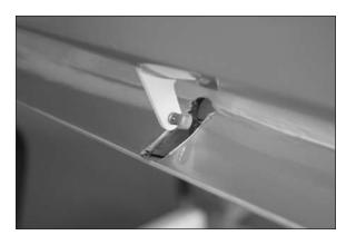
□□ 15. Use a pin vise and a 1/16-inch (1.5mm) drill bit to enlarge the holes in the flap servo cover for mounting the servo. Thread a servo mounting screw in each hole using a #1 Phillips screwdriver. Remove the screw, then apply 1–2 drops of thin CA in each hole to harden the surrounding wood.
