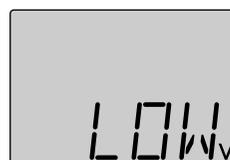
The low battery alarm is meant to be a safety feature only. Do NOT operate your radio below 9V. Always shut your radio off as soon as possible after the low battery warning tone to avoid loss of control.
