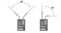
4 If your model includes metal conductive items which may impact the receiver's ability to clearly receive the radio frequency signal, we suggest mounting the receiver so that the receiver antennas exit both sides of the model. This will allow the best radio frequency signal condition at any flying attitude.
