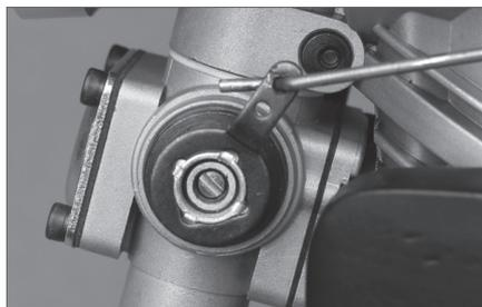
1. Use a secure method to attach the throttle linkage to the throttle arm on the carburetor.
