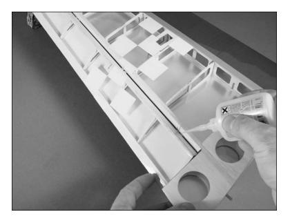
**Note**: Placing a #11 hobby blade between the aileron leading edge and wing trailing edge to position the aileron will result in a nice free moving hinge for 3D throws without any binding.
