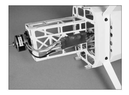
• 2. Connect the speed control to the radio system and motor battery. Check that the motor is rotating in the correct direction. It will rotate counterclockwise when viewed from the front of the aircraft. Use the instructions with your speed control to correct a motor that is operating in the wrong direction. • 3. Slide the cowling onto the fuselage. Secure the cowl using four 2mm x 8mm sheet metal screws.
