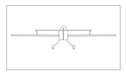
• 4. Double-check the adjustments from Steps 1 through 3. Use a felt-tipped pen to trace the outline of the fuselage onto the top and bottom of the stabilizer.
