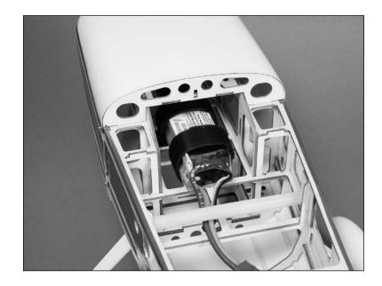
**Note**: Place a piece of hook and loop tape on the bottom of the battery and on the fuselage where the battery rests. This will keep the battery from shifting forward or backward during extreme maneuvers.
