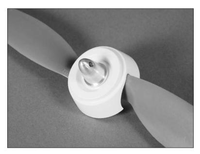
• 7. Install the propeller assembly onto the motor shaft. Tighten the propeller nut using a hex wrench slipped through the hole in the propeller nut.
