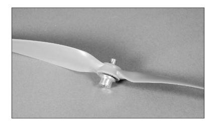
• 5. Slide the <sup>1</sup>/<sub>2</sub>-inch (13mm) plastic washer onto the adapter.
