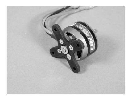
• 2. Attach the Outrunner motor to the front of the firewall using four black #4 washers and four 4-40 x <sup>3</sup>/<sub>8</sub>-inch socket head screws.
