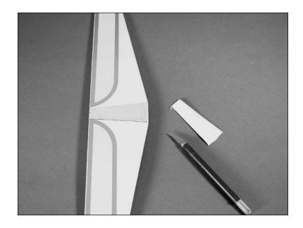
**Note**: You can use a soldering iron instead of a knife. This will eliminate the chances of cutting into the wood. O 6. Slide the elevator into position, then the stabilizer.
