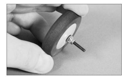
○ ○ 3. Attach the wheel to the landing gear using a black #4 washer and 4-40 lock nut.
