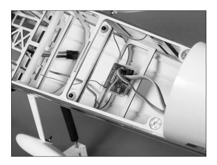
**Note**: Do not cut or change the length of the antenna wire, as this will reduce the range of your radio system.
