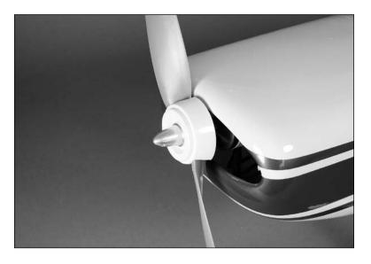
**Note**: Make sure to check the balance of the propeller after enlarging the hole in the propeller.
