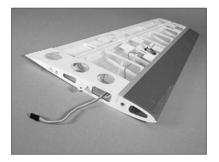
••• 3. Secure the aileron servo using the screws provided with the servo.
