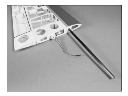
• 2. Remove the hatch from the fuselage. Slide the wing panel with tube into position on the fuselage.
