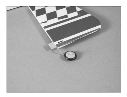
2. Hinge the rudder and fin, using the same process Ο as described in Aileron Hinging. Use three hinges for this process.
