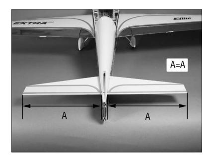
2. Measure from the stab tip to the wing tip. Adjust the Ο stab until the measurements are equal.
