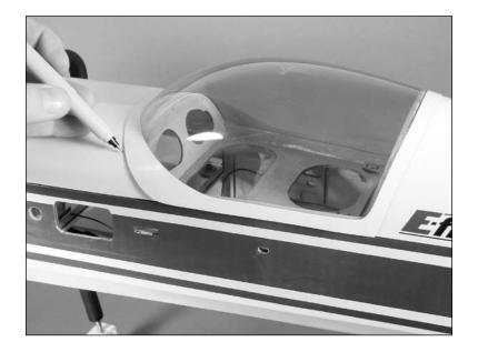
• 3. Use medium grit sandpaper to roughen the covering <sup>1</sup>/<sub>8</sub>-inch (3mm) inside the line drawn. Also roughen the outside <sup>1</sup>/<sub>8</sub>-inch (3mm) of the canopy. Clean the sanded areas using a paper towel and rubbing alcohol.
