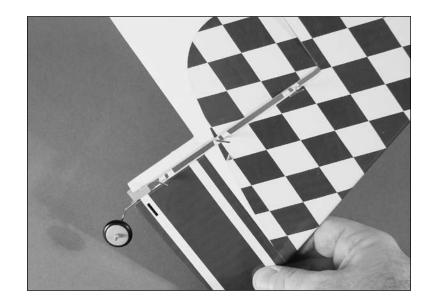
Ο 3. Place the fin in position on the fuselage. Trace the outline of the fuselage onto both sides of the fin.
