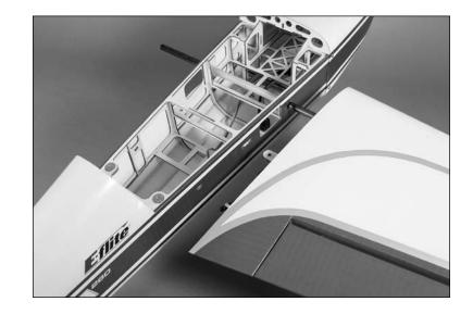
○ ○ 3. Slide the remaining wing panel into position. Secure the panels using 4-40 x <sup>1</sup>/<sub>2</sub>-inch machine screws with #4 washers (silver) using a <sup>3</sup>/<sub>32</sub>-inch hex wrench.
