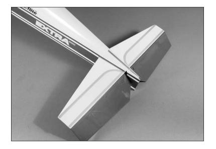
• 7. Follow the same procedure for hinging the ailerons to hinge the stabilizer/elevator. Use six hinges for this step.
