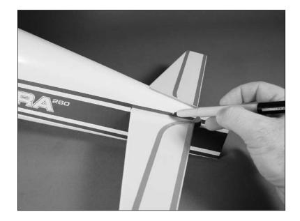
• 5. Use a sharp hobby knife to cut the covering slightly inside the lines drawn. Be very careful not to cut into the underlying wood, as this will weaken the stab and cause it to fail in flight.
