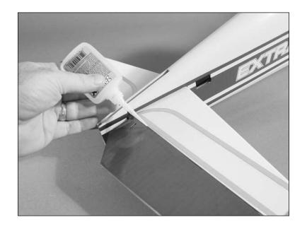
**Note**: Start with the two hinges at the center nearest the fuselage. Continue outward to the center hinges, then the hinges at the tips. Be careful not to damage the joiner section of the elevators.
