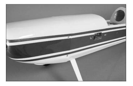
*Hint*: Use thin CA to harden the holes drilled into the cowl mounting tabs. This will help to prevent the screws from vibrating loose in flight.
