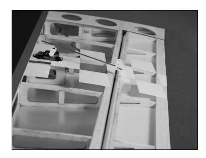
• 7. Attach the micro control connector to both servo arms. Be sure to use the included retainer to secure the micro control connector to the servo arms.
