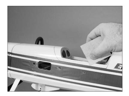
• 4. Use Formula 560 canopy glue to glue the canopy to the fuselage. Use masking tape to hold the canopy in position until the glue fully cures.
