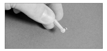
OO 8. Turn on the radio system and center the aileron trim and stick. Make sure the aileron servo is operating properly using the transmitter. Slide the pushrod wire through the micro connector. Install the servo arm parallel to the aileron hinge line. Center the aileron, and secure the position of the wire using the 2mm x 4mm screw and a Phillips screwdriver.
