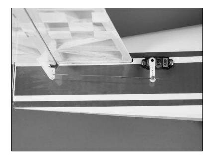
**Note**: The Extra 260 is designed to use an optional pull-pull rudder linkage when using a lightweight motor and battery. The items for the pull-pull system are available separately.
