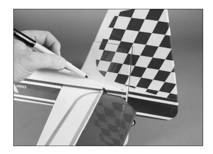
• 4. Remove the covering from the bottom of the fin using the same technique used for the stabilizer.
