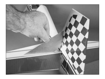
• 6. Use thin CA to glue the fin to the fuselage.
