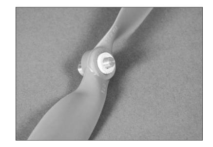
• 6. Slide the spinner backplate onto the adapter. Thread the propeller nut onto the adapter, but do not tighten it at this time.
