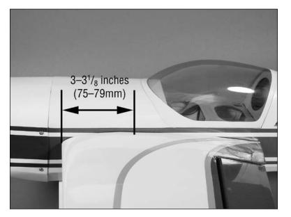
After your first flights, the Center of Gravity can be adjusted for personal preference.
