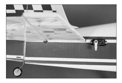
*Hint*: It is easiest to pass the extension through the former, then to the rear of the fuselage and retrieve it at the opening for the servo.
