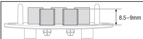
3. Remove the two screws holding the servo connector plate to the wing.
