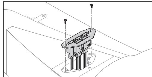
12. Loosen the setscrews for any connectors that require adjustment. Slide the connectors up or down until they are flush with the surface.
