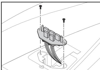
4. Lift the plate from the wing, taking care to not disconnect any servo leads.
