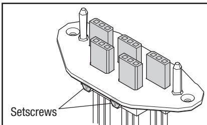
6. Using a screwdriver, push up on each of the connectors from the bottom of the plate until they are fully seated against the stop in the mounting plate. Check each connector to ensure they fall within the 8.5–9mm range above the mounting plate and adjust accordingly.
