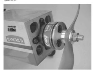
NOTE: Photo shows typical installation of motor and x-mount directly to the outside of the firewall. There are other options available including mounting the motor inside the fuselage or extending the motor further forward using aftermarket mount extensions when using cowls
