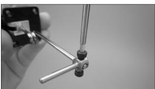
4. Install the wheels on the axles. Slide the brass wheel collar onto the axle and secure it using a 1.5mm hex wrench. Apply threadlock to the setscrew to prevent it loosening due to vibration.
