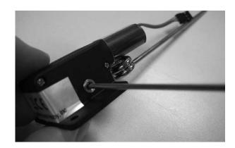
2. Test fit the retract unit in the wing or fuselage to determine the strut length and axle location. Cut the strut to length using a cutoff wheel in a rotary tool.
