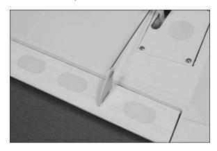
16. Pass the pushrod through the pushrod connector and center the aileron. Use a #1 Phillips screwdriver to tighten the screw in the pushrod connector to secure the pushrod wire. Use side cutters to remove the excess wire. Support the clevis and the wire while doing this to not damage the model.
