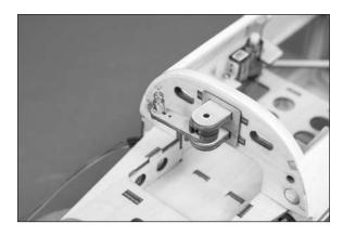
5. The end of the nose gear wire may have to be filed slightly to remove any burs or edges for an easier fit.
