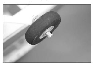
18. Fit the wheel pant over the wheel and its components. Make sure the wheel pant is positioned between the gear and the washer that was installed in Step 12. You may need to reposition the 2mm nut to fit the wheel pant into position.
