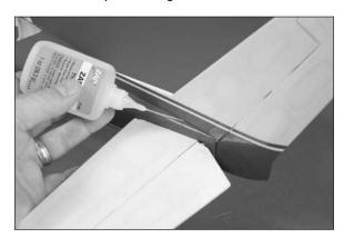
7. Also apply a small amount of thin CA where the tab at the front of the vertical fin fits into the fuselage. It may be necessary to hold the fin tightly against the fuselage until the CA fully cures.
