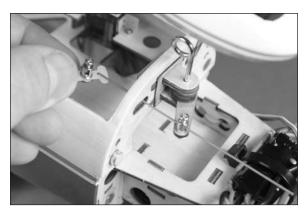
O 10. Center the rudder servo using the transmitter. Attach the servo horn to the rudder servo using the screw provided with the servo and a #0 Phillips screwdriver. The arm will be parallel to the rear edge of the battery plate in the fuselage, just like the elevator servo.
