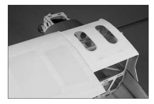
4. Place the remaining wing panel into position.
