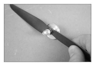
7. Slide the assembly on the motor shaft. Position the assembly so there is a small 5/64-inch (2mm) gap between the backplate and cowling.
