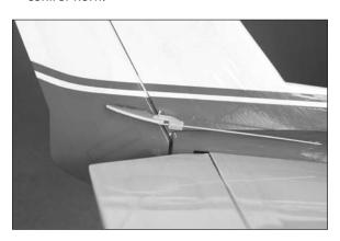
13. With the radio system on and the rudder servo centered, check that the control surface is aligned with the fixed surface. Use a square between the two surfaces. Use a #1 Phillips screwdriver to secure the pushrod in the pushrod connector.
