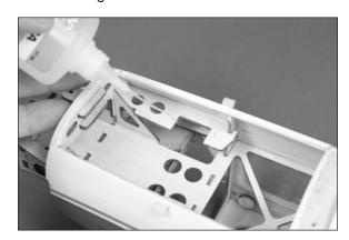
OO 6. Use the screws provided with the servo and a #0 Phillips screwdriver to secure the rudder servo in the fuselage. Use care not to push too hard on the mounting rails while tightening the screws.
