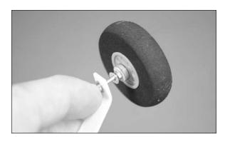
17. Once the wheel is in position, place one of the wheel collars on the screw. The round side of the collar will be against the wheel. Use a 1.5mm hex wrench to temporarily tighten the setscrew.
