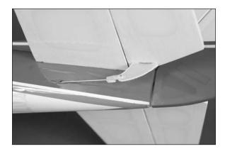
5. With the radio system on and the elevator servo centered, check that the control surface is aligned with the fixed surface. Use a square between the two surfaces. Use a #1 Phillips screwdriver to secure the pushrod in the pushrod connector.
