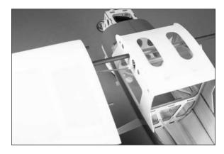
3. Slide the wing so it fits tightly against the fuselage as shown.
