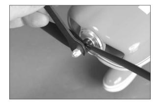
9. Place the spinner cone on the propeller. Use the screw included with the spinner assembly and a #1 Phillips screwdriver to secure the cone in position. Make sure the propeller is centered in the openings so the spinner does not rub against the prop blades, which could potentially cause them to fail.
