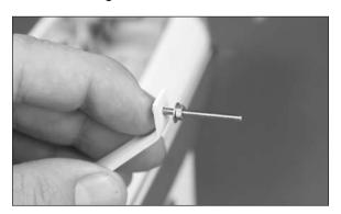
OO 16. Slide the plywood spacer on the screw, then the wheel.
