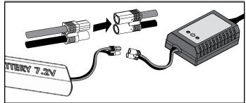
The vehicle battery charger produces 2000 milliAmps (2 Amps) per hour. Divide the mAh capacity on the label of a battery by 2000 to know how long battery charging will require. For example, a fully discharged 1800mAh battery requires 0.9 hours (54 minutes) to charge.
