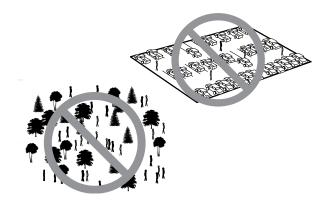
• ALWAYS operate your vehicle in a wide open area. Operating the vehicle in a small space or indoors can cause overheating at low speeds. Operating at low speed increases heat in the electronic speed control (ESC). Overheating can damage the vehicle and failure may result.
