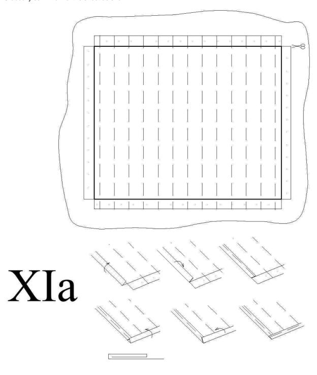
b) Sew rope 49 around the perimeter of the sail. Towards the centre of the sail tie the rope to control the sails 43.
