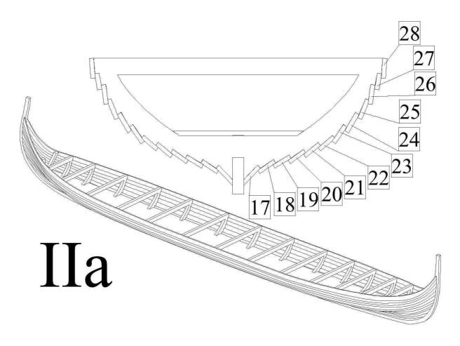
b) Cut off the parts of ribs 1-13, which overlap overboard. Attention! Ribs 15 and 16 leave in the original state.
