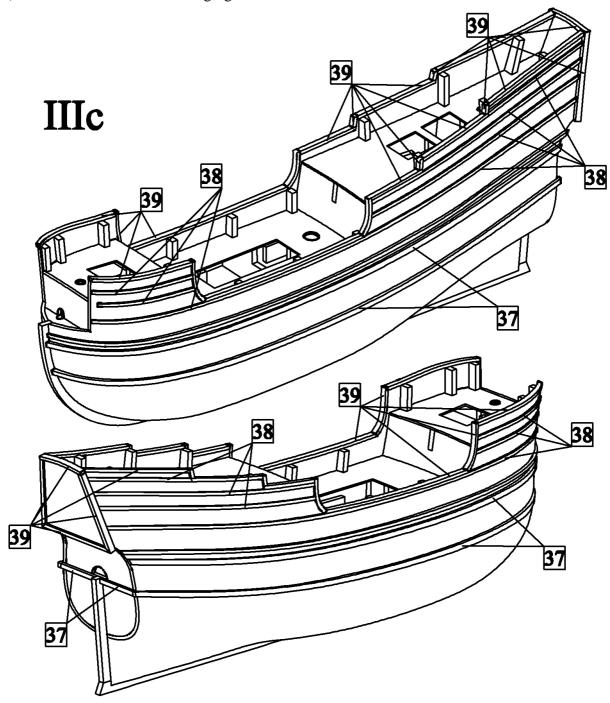
d) Carefully cut off parts of the frames which overhang the decks.
