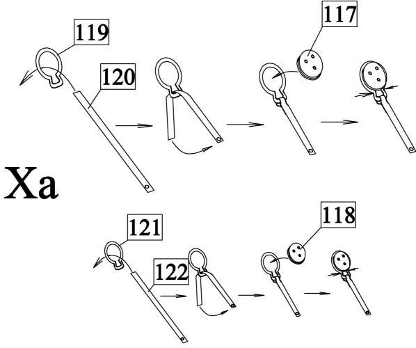
b) First glue the deadeyes to the channels and then glue capping strips 123 to the channels too.
