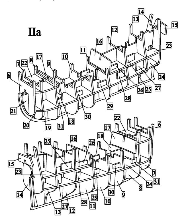
b) Grind the frames on the bow and stern as it is shown in the figure.
