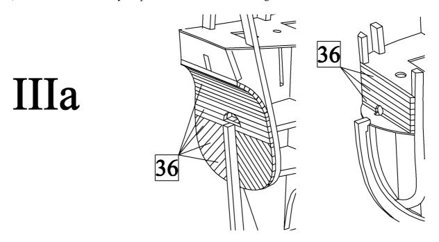
b) Plank the hull by strips 36. Make the planking in directions from the bow to the stern. Finally plank also the stern.
