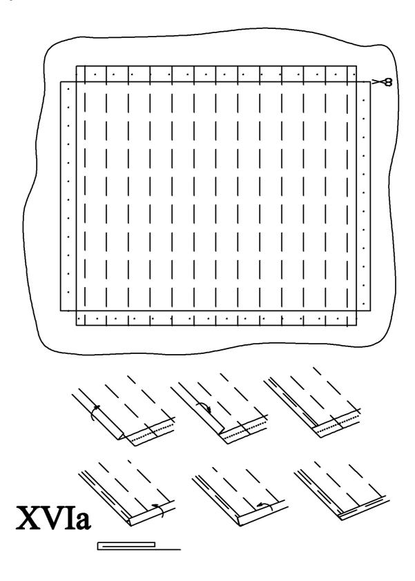
b) To the circumference of the sails sew on ropes 157 so that in the corner of the sail will eyes with diameters about 3mm. Then tie ropes 135 to the sails.
