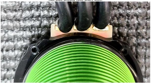
**Step 3: Slide O-Ring over motor to last ribbed fin.**
