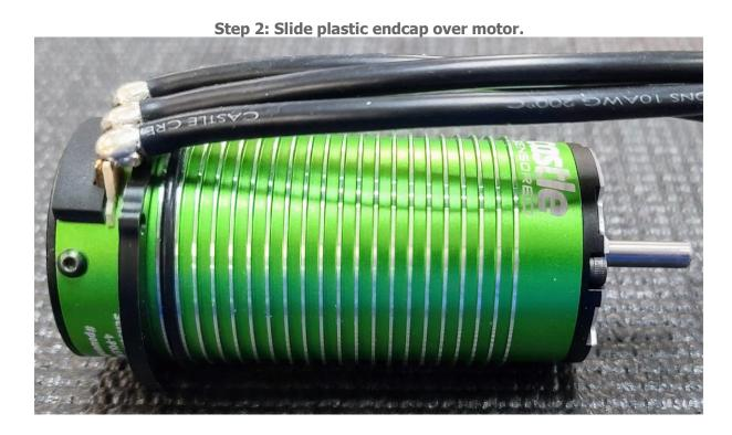
Notes: Align recessed side with motor wires. Recessed holes should face back of motor, flat side should face shaft side.
