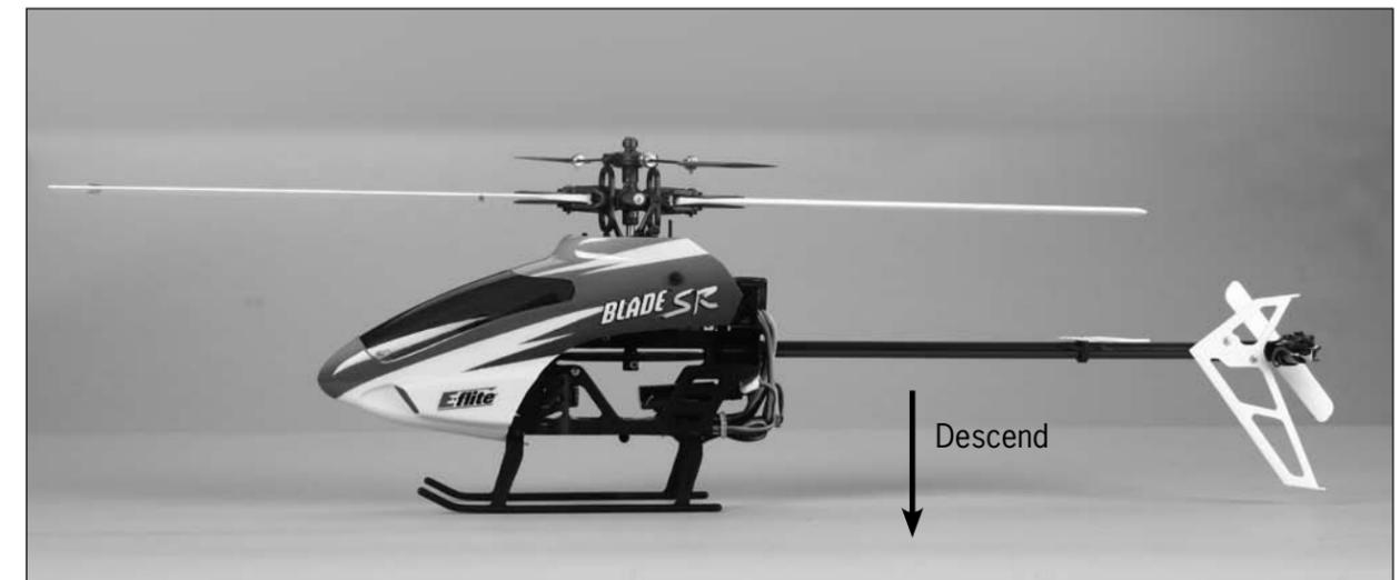
After lifting the model off the ground you can balance the throttle/pitch by carefully moving the left-hand stick up and down so the model will hold a stationary hover without climbing or descending.
