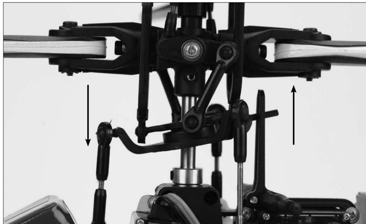
With the stick pulled back, the swashplate will tilt toward the rear.
