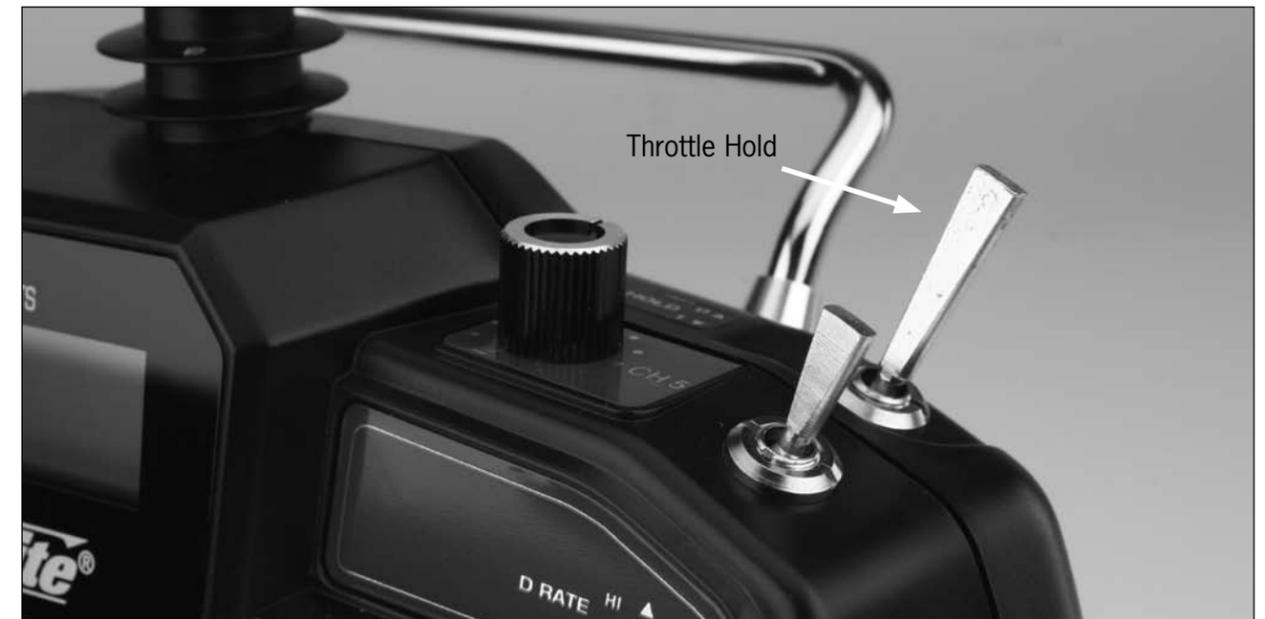
When the throttle hold switch is toggled toward the rear of the transmitter (position 0), throttle hold will be off. When throttle hold is on, the transmitter will be in the normal or stunt flight mode (depending on the position in which the F MODE switch is set).
