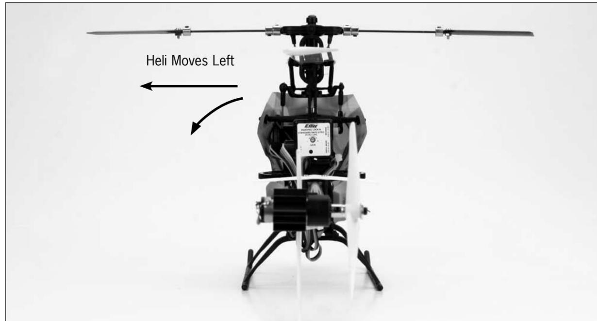
Moving the stick to the right will roll the helicopter to the right, allowing the helicopter to be flown to the right.
