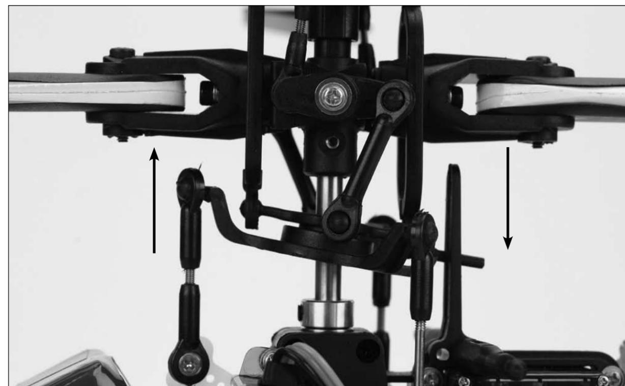
While viewing the helicopter from the rear (tail boom toward you), move the right-hand stick left and right to check aileron roll control. When the stick is pushed to the left, the swashplate should also tilt left.
