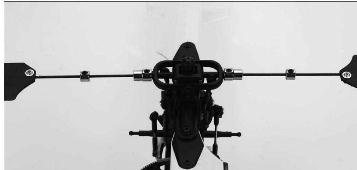
Dampening of the rotor head (main rotor blades) can also be adjusted in order to fine-tune the cyclic response of your model. In general, stiffer dampening will result in quicker cyclic response. The dampening of your Blade SR has been set to provide good stability right out of the box, and we suggest that you make your first flights with this amount of dampening before making any changes.
