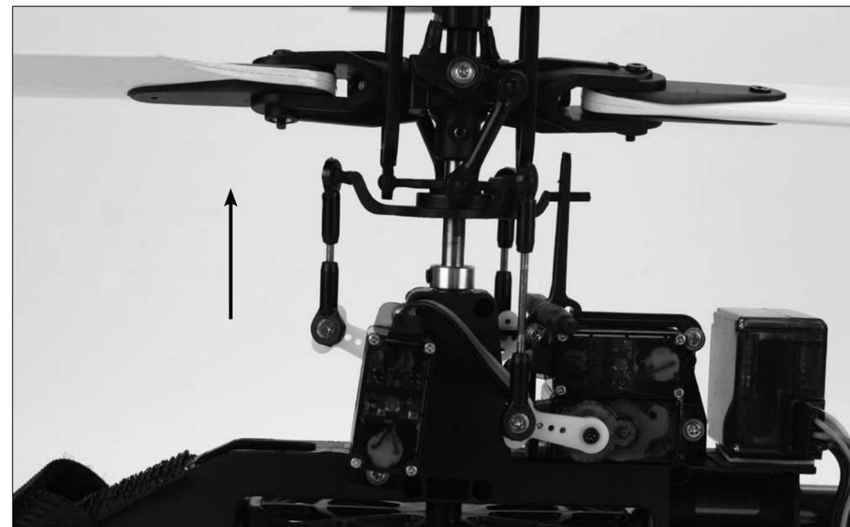
Again viewing the helicopter from the left or right side, move the right-hand stick forward and aft to check elevator pitch control. When the stick is pushed forward, the swashplate should also tilt forward.
