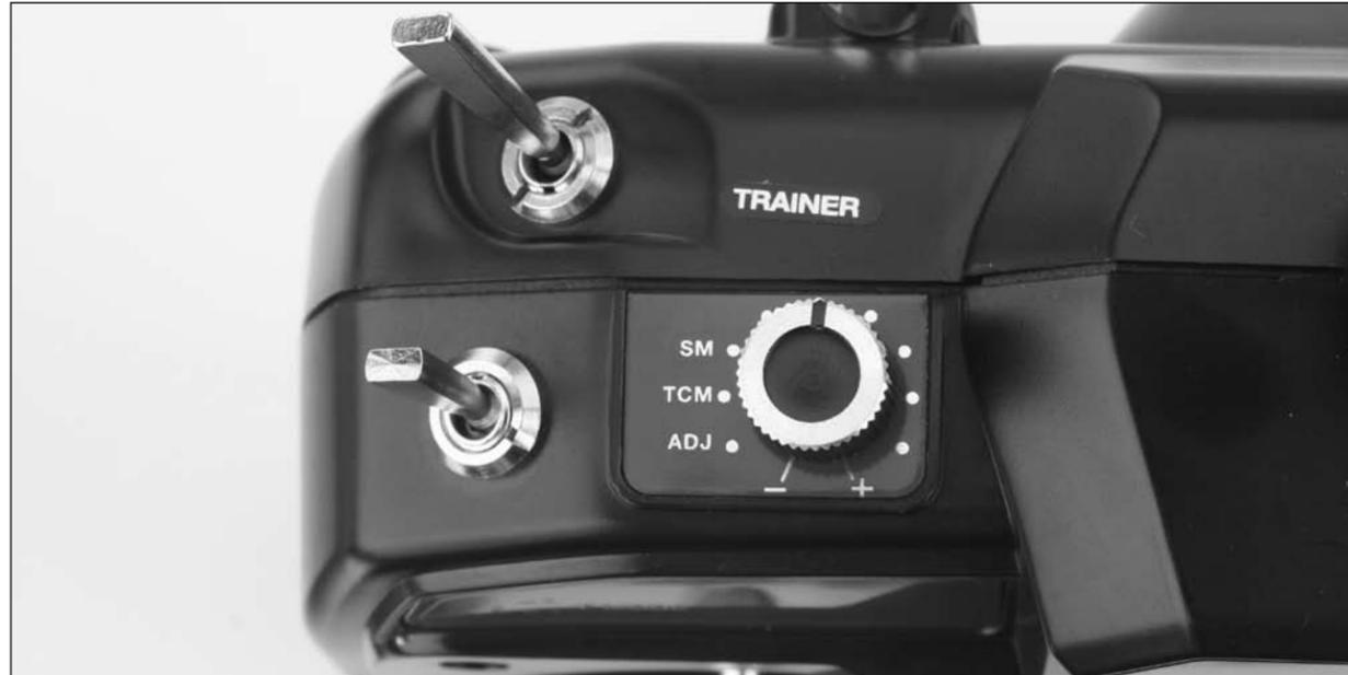
The SM TCM ADJ knob offers you the ability to adjust the main rotor head speed, and in turn the collective and cyclic control response of the model between the endpoints of the throttle curve in the stunt flight mode. Typically, a higher main rotor head speed will result in quicker collective and cyclic control response around middle stick.
