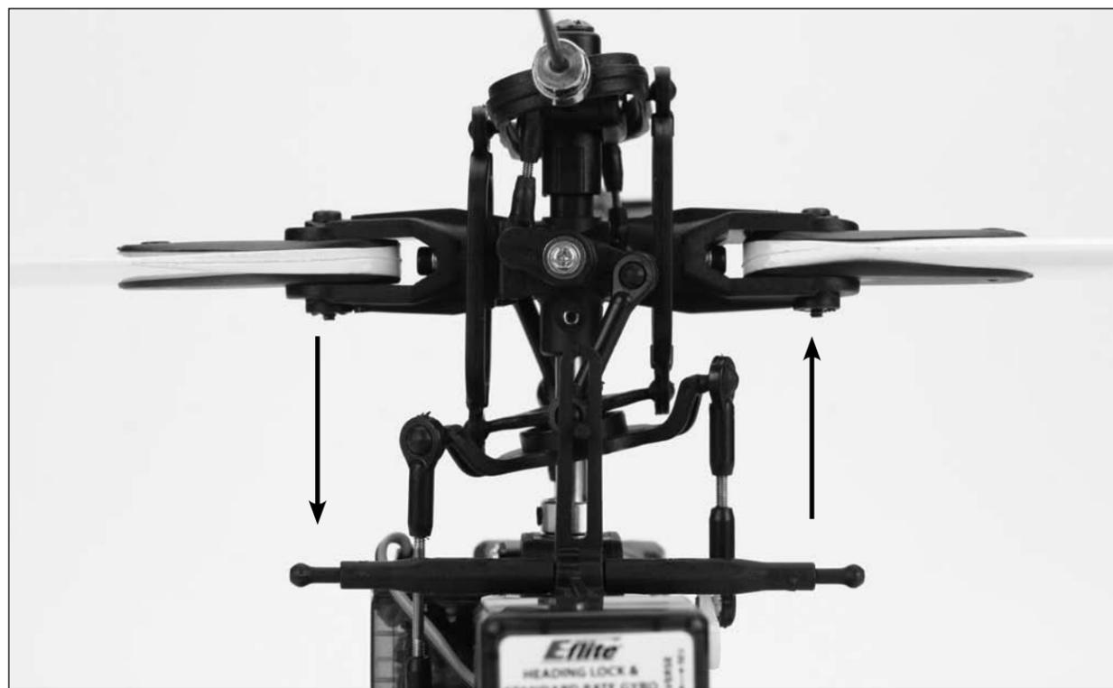
With the stick pushed right, the swashplate will tilt to the right.
