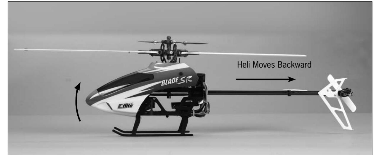
The elevator trim can be used to help keep the helicopter from drifting forward or backward when in hover with no elevator stick input. For example, if the helicopter drifts forward when in hover, pull the elevator trim downward until the helicopter hovers as level as possible with no forward drifting.
