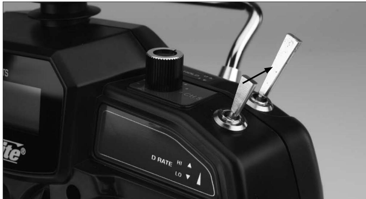
Toggling the switch toward the front of the transmitter (position LO) allows the control rates to achieve their lowest maximum values. This is typically the preferred rate for low-time and other pilots interested most in a reduced amount of control that allows for smoother and more easily controlled hovering and flying.
