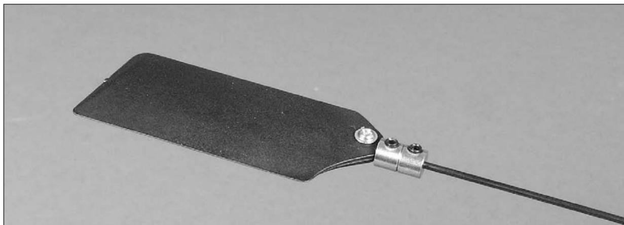
If, after the first few flights, you would prefer to have even quicker and more aggressive cyclic response, you can reposition the outer flybar weights so that they are closer in to the head/main shaft on the flybar. It is usually best to move the weights in only a small distance at a time before making each subsequent test flight, until you find the position at which you prefer the cyclic response most.
