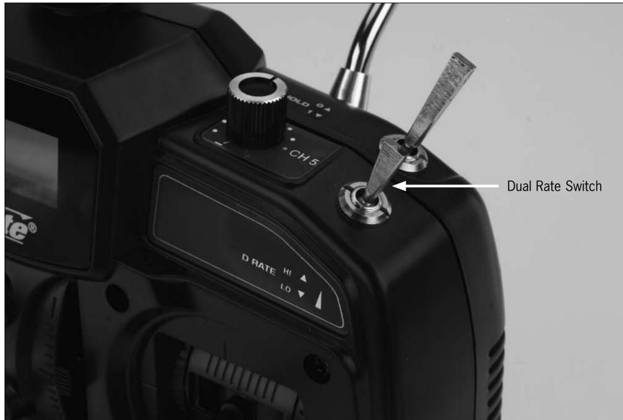
Toggling the switch towards the back of the transmitter (position HI) allows the control rates to achieve their highest maximum values. This is typically the preferred rate for experienced pilots interested in more control response for forward flight and basic aerobatic maneuvers.
