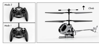
Decreasing the speed of the main rotor blades by lowering the left-hand stick will cause the model to descend.
