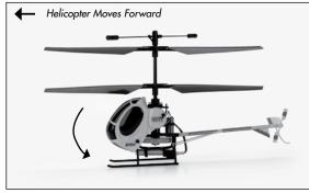
Pulling the elevator stick backward will pitch the tail of the helicopter downward, allowing the helicopter to be flown backward.
