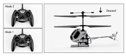
After lifting the model off the ground you can balance the throttle by carefully moving the throttle stick up and down so the model will hold a stationary hover without climbing or descending.
