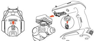
STEP 1) Carefully slide the top part of the CGO2-GB (that also attaches below the nose of the Q500 Typhoon) onto the mount below the front part of the SteadyGrip™ A corresponding 'click' will be noticed once the CGO2-GB has securely been installed into the slide-in mount on the SteadyGrip™.
