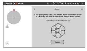
NOTICE: The battery level must be above 30% to start the update process.
