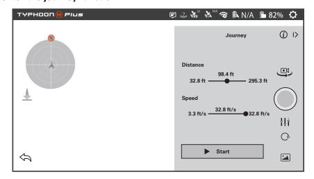
Distance can be adjusted manually between 32.8ft and 295.3ft, and speed between 3.3 ft/s and 32.8 ft/s.
