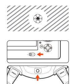
**STEP 3**: Lift the TYPHOON H PLUS airframe straight and level. When the LEDs on two motors start to blink green as illustrated, turn it forward as shown by the red arrow until a tone is heard and the two LEDs turn off.
