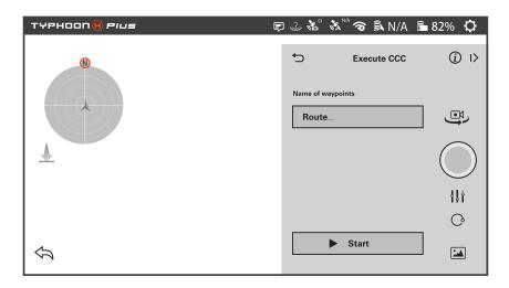
**Save**: Tap Save and the current route will be saved. The name of waypoints can be defined by the pilot. **Start**: Tap Start, TYPHOON H PLUS will fly back to waypoint 1 automatically.
