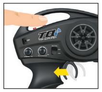
You can fine tune the speed to exactly match your pace by adjusting the multi-function knob on the transmitter. Turn the knob clockwise to increase speed, counterclockwise to reduce speed. You can accelerate and drive faster with the Cruise Control set, and the vehicle will resume the set speed when the throttle is released (*Resume function*).
