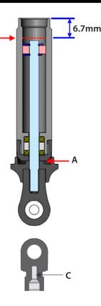
Important: The shocks are assembled at the factory with a center-to-center distance (between the rod end balls) of 90mm. Any time the shocks are removed and disassembled, this distance should be checked to ensure proper operation of the suspension.
