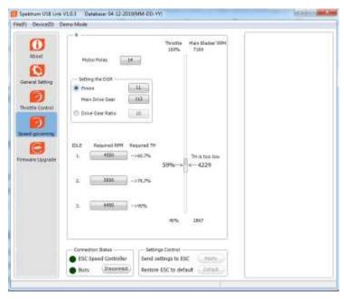
When you adjust the throttle curve, please make sure that the motor can run at this preset speed even if the motor load is heaviest. Please note that the governor mode function is automatically disabled if the throttle volume is less than 60% or more than 90% to allow for proper motor control in high and low load scenarios.
