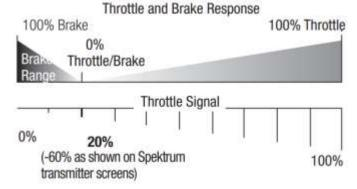
Brake Force – This option is adjustable from level 0 (\* Default) to level 7. The higher the level, the stronger the braking effect. Brake Force is only effective in the "Normal brake" mode.
