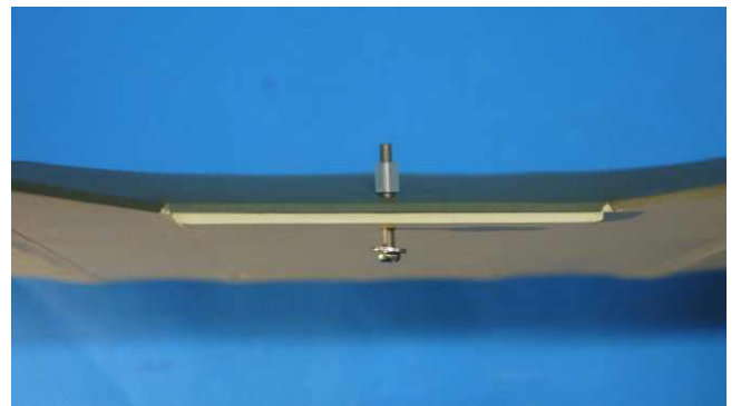
Prepare M3x25, washer and plastic nut.
