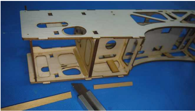
According fuselage cut 3X5mm wood strips and attach with instant glue.
