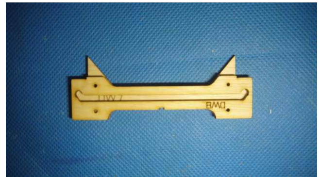
Prepare Dw7 and DW8. Place DW7 on the bottom and glue DW8 on it.
