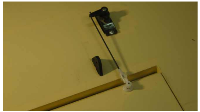
Put Z bend part to connect the servo arm.
