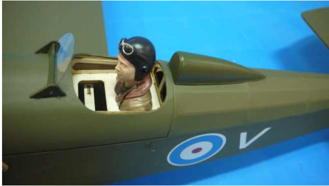
Place the pilot pillow behind the pilot.
