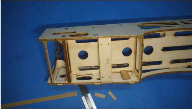
Cut triangle wood strips and attach inside of F21 with instant glue.
