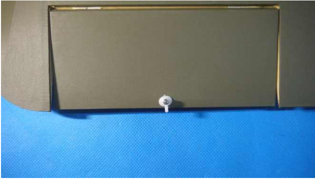
Secure the control horn set onto the aileron of second wing.
