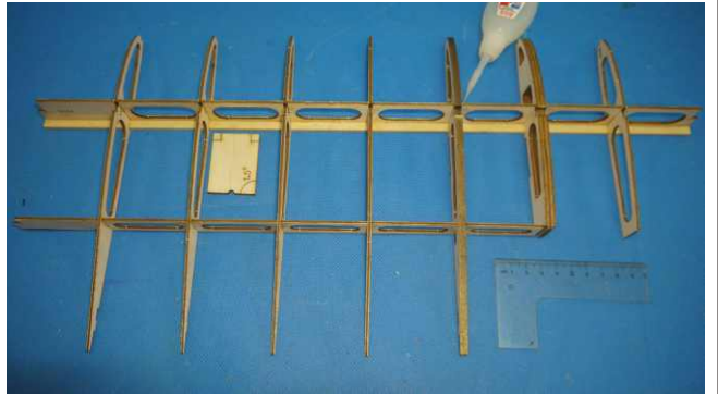
Please the wing ribs on W14 and secure with instant glue. (Please make sure every rib is vertical.)
