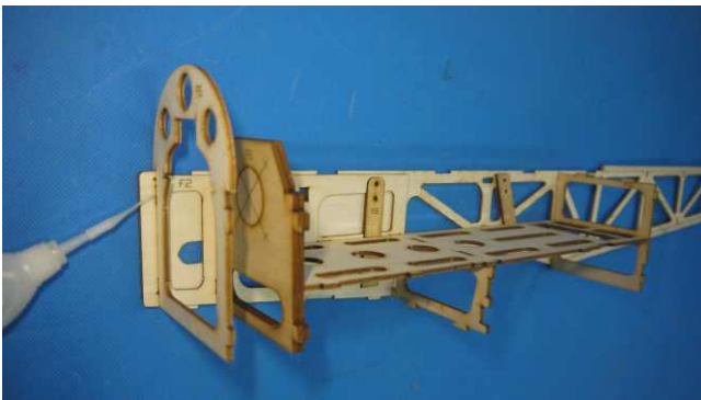
Attach C11 with F8, then attach with right side F2.
