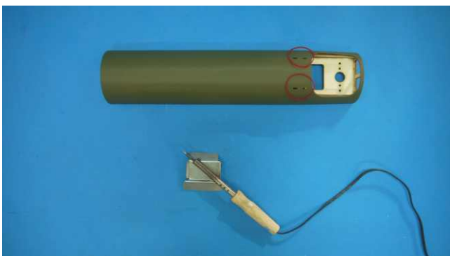
Remove the covering as the circle marked. (Small hole)
