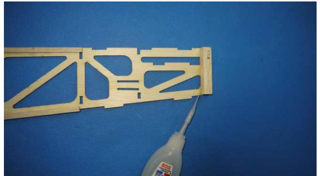
Attach F16 with instant glue.
