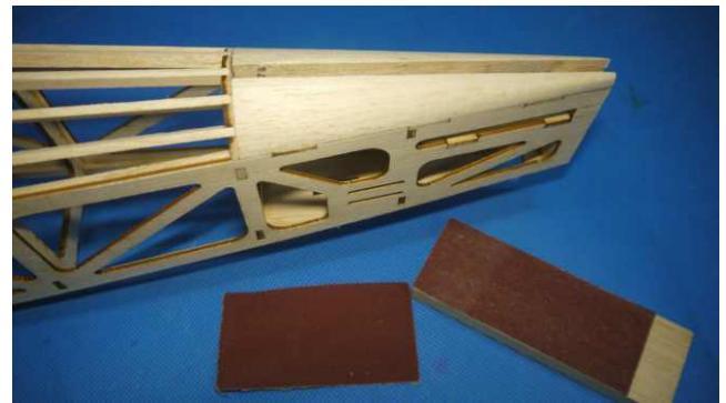
Cut off extra piece and sand it until smooth.
