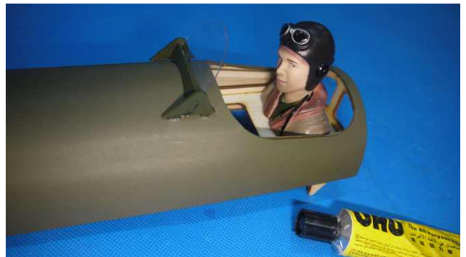
Attach C14 and C15 with instant glue. Then paint it. After covering attach window with instant glue.
