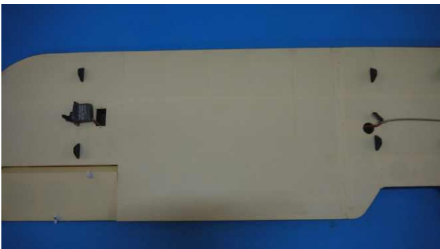
Place the servo into the servo hole and pull out the servo line to the wire exit.
