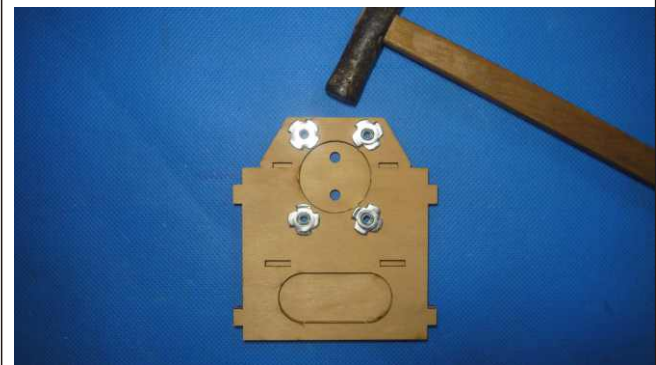
Take four clutch nails and use a hammer to place the clutch nails into these holes
