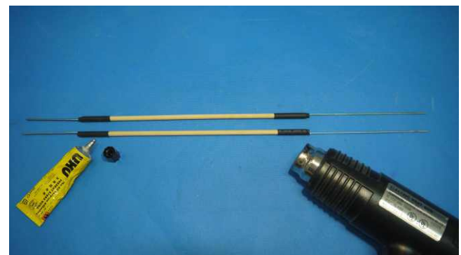
Prepare above part and assemble the rod for the elevator and rubber. Slide in shrinking tube on the conjunction. Use heat gun to make the tube shrinking for the reinforcement.
