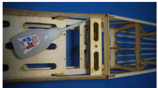
Attach into the fuselage with instant glue.
