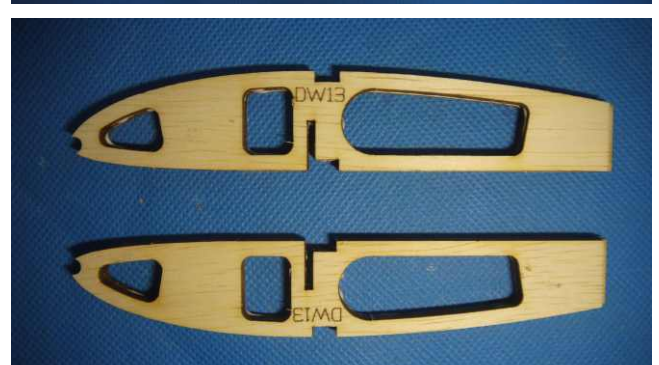
Prepare 2 pieces of DW12 and 4 pieces DW13. Place DW12 in the middle and glue DW13 on both side.
