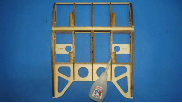
Attach W9,W13 and W11 with instant glue.
