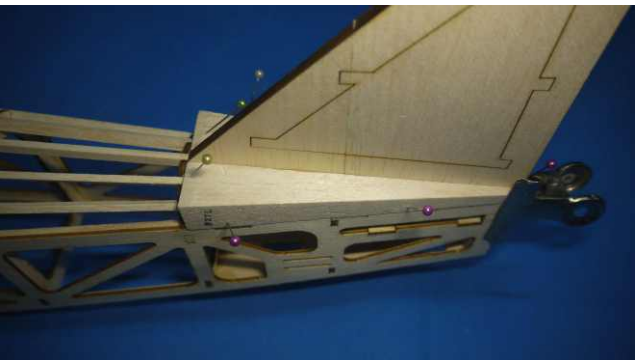
Secure both side you attached.
