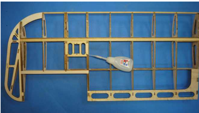
Prepare ?? then attach with instant glue.
