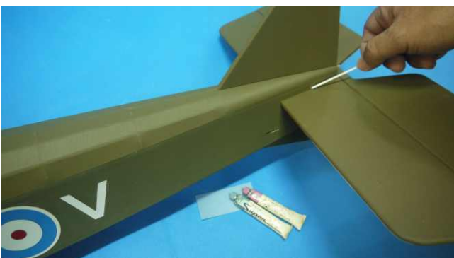
Apply Epoxy to secure all these parts to the fuselage.
