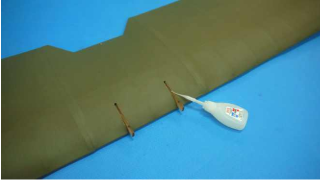
Place 2 pieces of DW10 and attach with instant glue.
