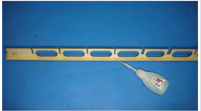
Cut 3X6.5X464 mm hard wood strips and attach with instant glue. The angle between W14 and hard wood is 90 degrees.
