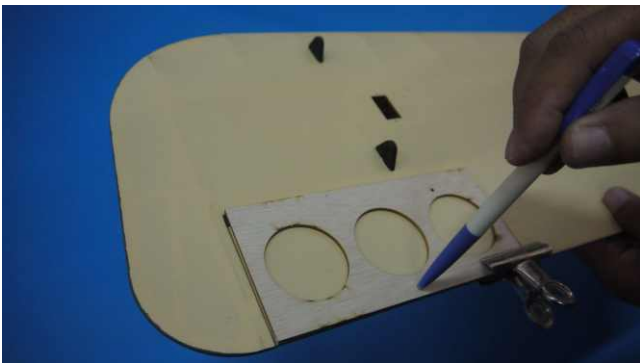
Place 2 pieces of DW10 and attach with instant glue.
