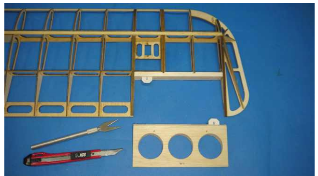
Cut the hinge holes and install the fiber hinges.
