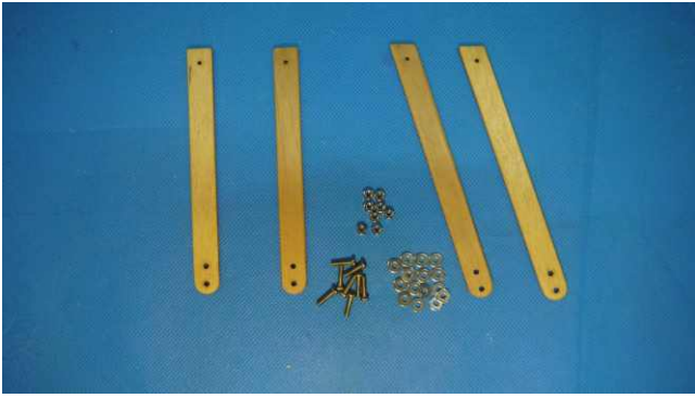
Prepare F28,F29, M2x10,M2 nut and washer
