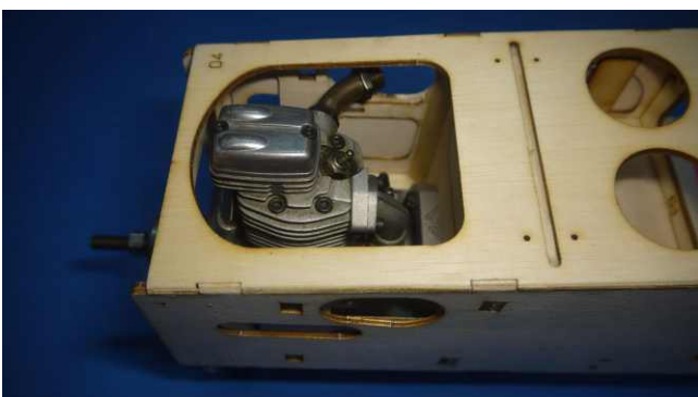
Install engine(Remove Exhaust Pipe)
