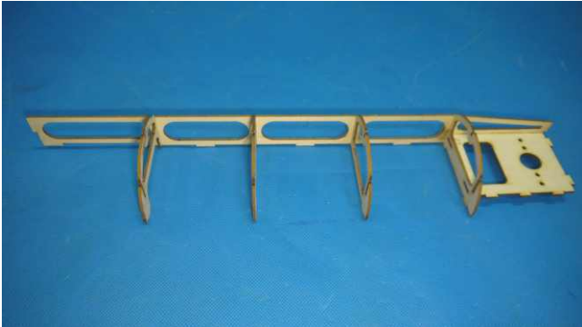
Join C5, C5, C6, C7, C2 to C1.
