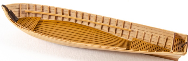
Using superglue (CA), glue the floor/deck sections into place as seen here.
