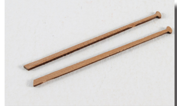
75. Take the two Till Arm parts 75 and glue them together. When dry, sand the Tiller Arm to round the edges and then drill then end of it to insert a cut-off brass pin that will be used to pin it to the rudder. Do NOT glue the tiller arm to the rudder yet.
