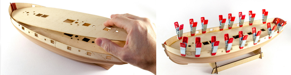
64. The laser-engraved deck can now be fitted over the ply deck. Test fit it first, and if you need to sand the edges at all, use medium grade paper. I now used wood glue, running thin beads around the edges of the deck and openings, and adding spots in other areas. The deck is then sat in position and a series of small clamps sat around the edges, holding it in position while it dried. If you do want to put weight on the middle area, please put some paper on the deck first to protect it from any marks.
