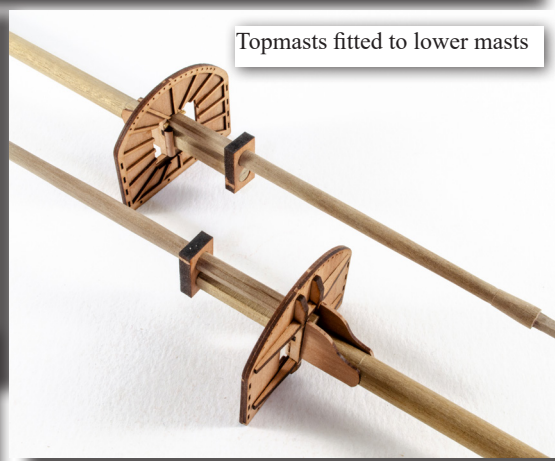
Fore and main topgallant masts showing the lower ends with main caps in place, followed by the 'fids' or stoppers.
