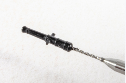
122. Drill the rear of the resin Half-Pounder swivel gun barrels, using a 0.8mm drill, and glue the gun handles into position.
