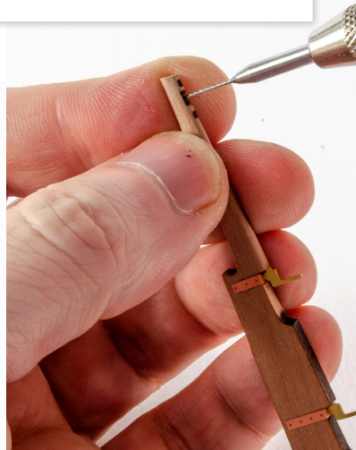
73. Drill a 0.8mm hole in the top of the top of the rudder, in the position shown. This will be to fit the tiller arm.
