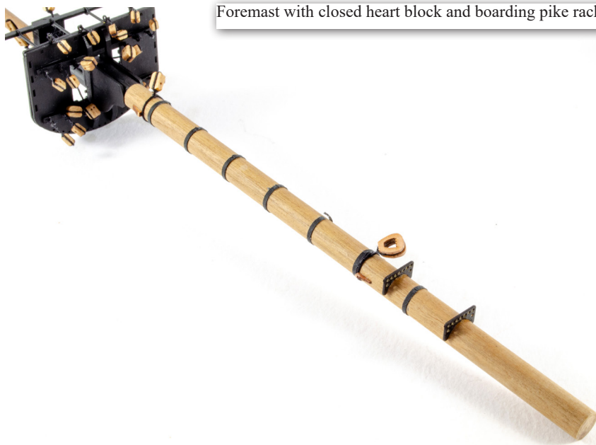
Foremast with closed heart block and boarding pike rack in place
