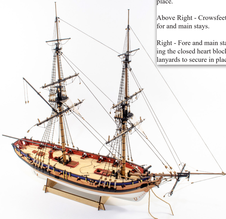
Below - All mast stays rigged in place.
