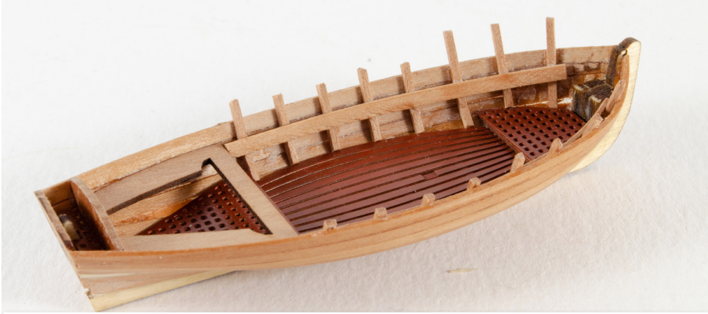
137. Now we need to fit the inside rail. I marked the top of the rail on my prototype as 2.5mm down from the top of the bulwark, but with evaluation, this would be better being located about 4mm from the top bulwark, but the sequence you see is the same. Split another 3mm strip and glue the rails 1.5mm wide, along the ribs using PVA and allow to set. Trim and sand the protruding ribs from the top of the bulwarks.
