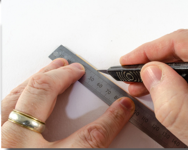
45. Make a pencil mark about 1/4 to 1/5 of way down from the width of the plank (at each end), and then taper using these two points. A very sharp knife is recommended, and also do this with several shallow cuts and don't try to cut through all at once. You also may wish to soak the plank before cutting as this can make tapering easier.
