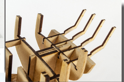
29&30. Glue the Stern Frame Patterns into their relative positions at the stern, making sure you push the parts fully into position as seen in this photograph.
