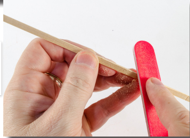
47. As you progress with your planking, you'll find that you will need to bevel the edges of them to ensure you don't have any edge-edge gaps. A sanding stick (shown) or a piece of medium grade sandpaper is advisable.
