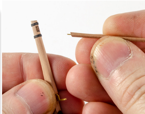
74. Cut two strips of the supplied Black Cartridge Paper F-38 (approx. 1.5mm wide) and glue to the rudder, in the positions shown.
