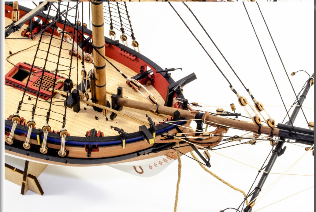
Right - Fore and main stays showing the closed heart blocks and lanyards to secure in place.
