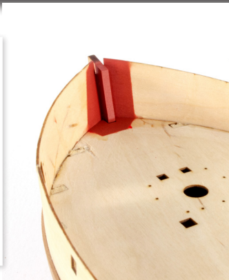
63. Before you add the laser-engraved deck, the inner bow and stern need to be painted in a suitable red colour. It will be more difficult to do this later without accidentally getting paint on the deck. For this, I used Plastikote Red Oxide primer, after first masking off the rest of the hull with adhesive tape.
