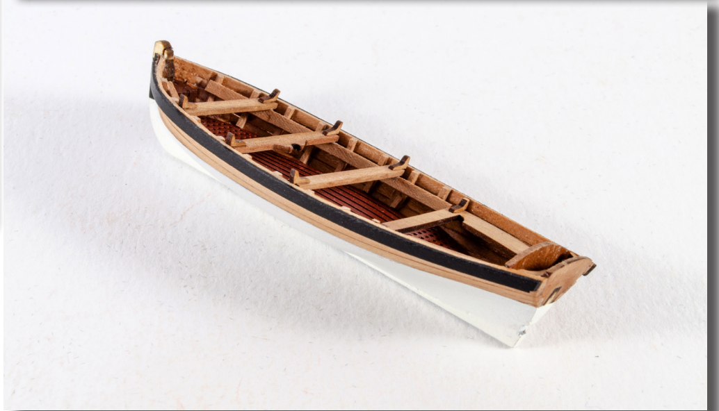
140. Add a strip of 1.5mm x 1mm wood along the top of the bulwark so it sits at the same height as bulwark top. Paint this black. Add the gunwale by simply cutting 1mm x 3mm wood strip to 1.5mm width, and gluing to the top edge of the bulwarks, leaving 1mm gaps for the oars to sit.
