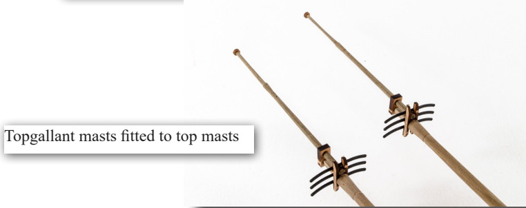
Fore and main top masts showing the lower ends with main caps in place, followed by the 'fids' or stoppers, which stop the mast from falling through the lower trestle trees.
