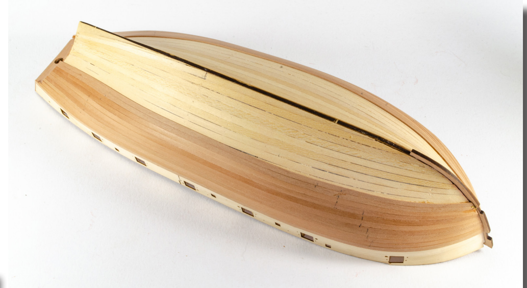
60. Work your way down the hull, tapering each plank at both bow and stern. I still tend to alternate the planks, although the hull is now very strong and not prone to warping. To glue this second layer, I used CA gel (Gorilla Glue), applied in a thin line from the nozzle. Don't apply too much as you don't want it to start oozing from between the planks, although we can sand that down later. If you need to use infill/stealers, this will be in the lower area of the hull, and it will be hidden by a layer of paint. Do NOT plank above the master plank at this stage. Also don't throw away the short end 'cut-offs' of planks as we can/will use them later. If you find that a plank needs to be soaked before fitting, you can do this in hot water, but it's not advisable that you glue it whilst wet, or shrinkage could occur after gluing.
