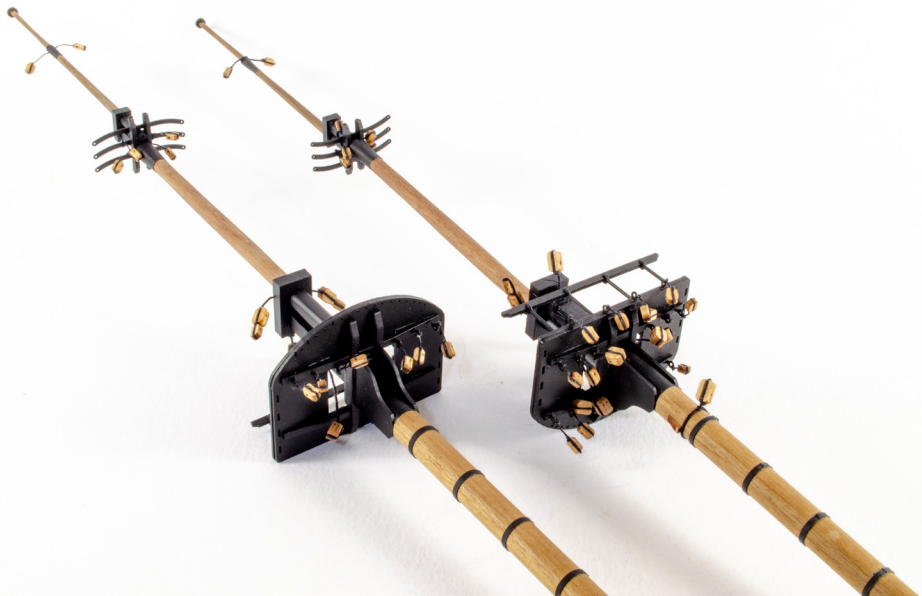
Foremast with closed heart block and boarding pike rack in place
