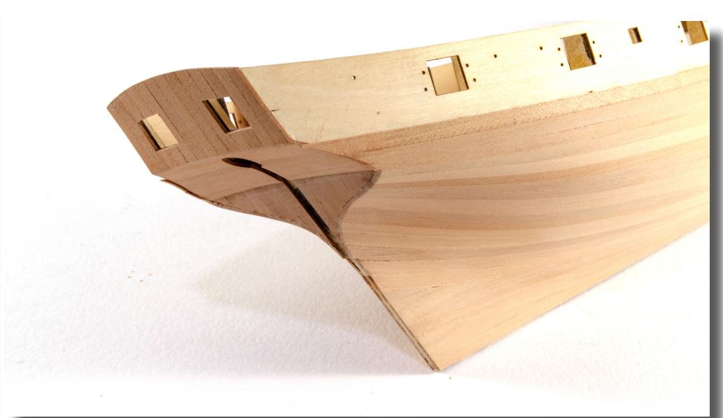
61. Trim and sand the second layer planks at the stern so they are flush with the stern planking.
