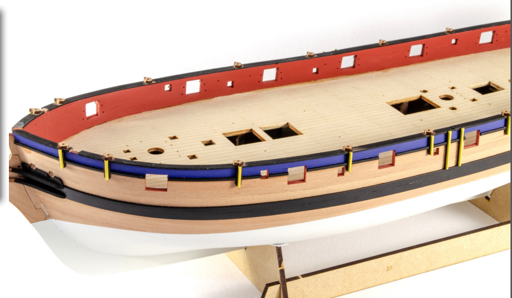
90. Cut two Cathead timbers (139) from the 4mm wood sheet. Also remove two Cathead Cleats (PE-35) from the 0.6mm brass sheet. Glue these into the Catheads, check the plan for orientation. Paint the Catheads in black and add the Cathead End Cap Decoration PE-6 after painting them yellow. We used Humbrol 74.
