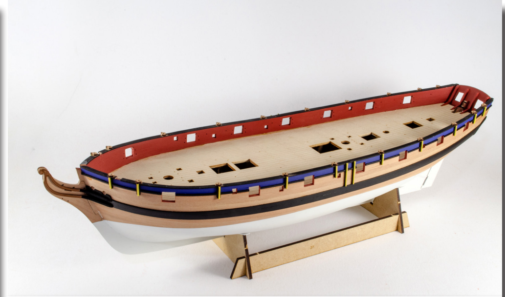
91. Cut the Swivel Gun Post Support Timbers (40a/b, 41a/b, 42a/b/c, 43a/b, 44a/b) from the 0.8mm ply sheet and paint them yellow before gluing in position as shown in this photo and the illustration. These are specific to their location, so don't mix them up. Now glue the Half-Pounder Gun Bases #103 into position on the gunwale, above the Upper rail and swivel gun post patterns.
