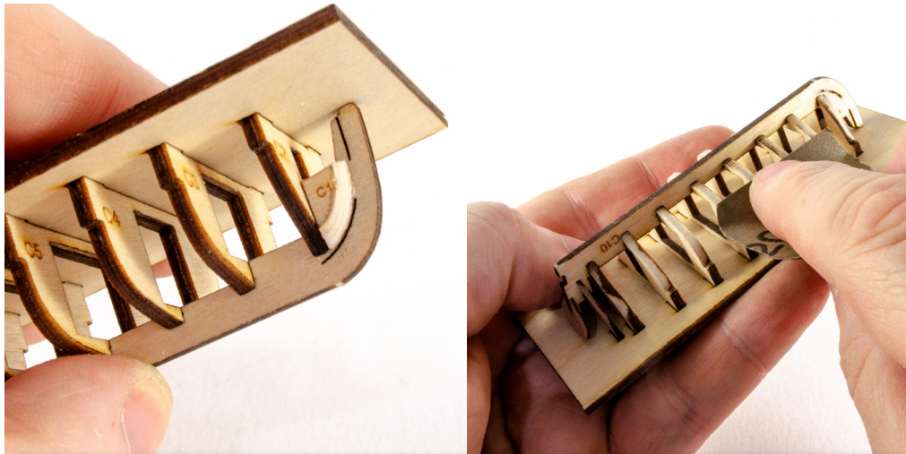
132. Bevel and glue into position the Cutter bow planking patterns C11, as shown here. When these have dried, sand the frame smooth, or fair it. This allows for the planks to lie across them with most contact.
