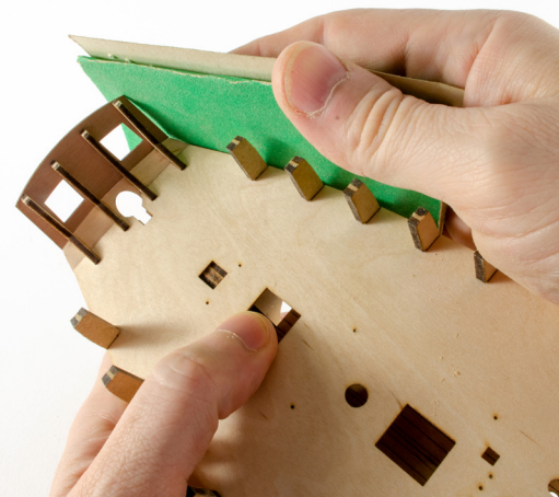
37. Carefully sand the edges of the stern patterns so that the lower counter edge is flush with the deck edge. Also give the fore and aft bulkheads a final sand for the gun port patterns and planking to have maximum contact with the edges of the bulkheads. It is also a good idea to evenly thin the MDF where the stern post will fit. On our prototype, we thinned this down to about 1mm. To do this, mark a pencil line right down the middle of this length so ensure you thin this evenly. We also tapered the bottom of the False Keel in towards the sternpost location, thinning the deadwood area too.
