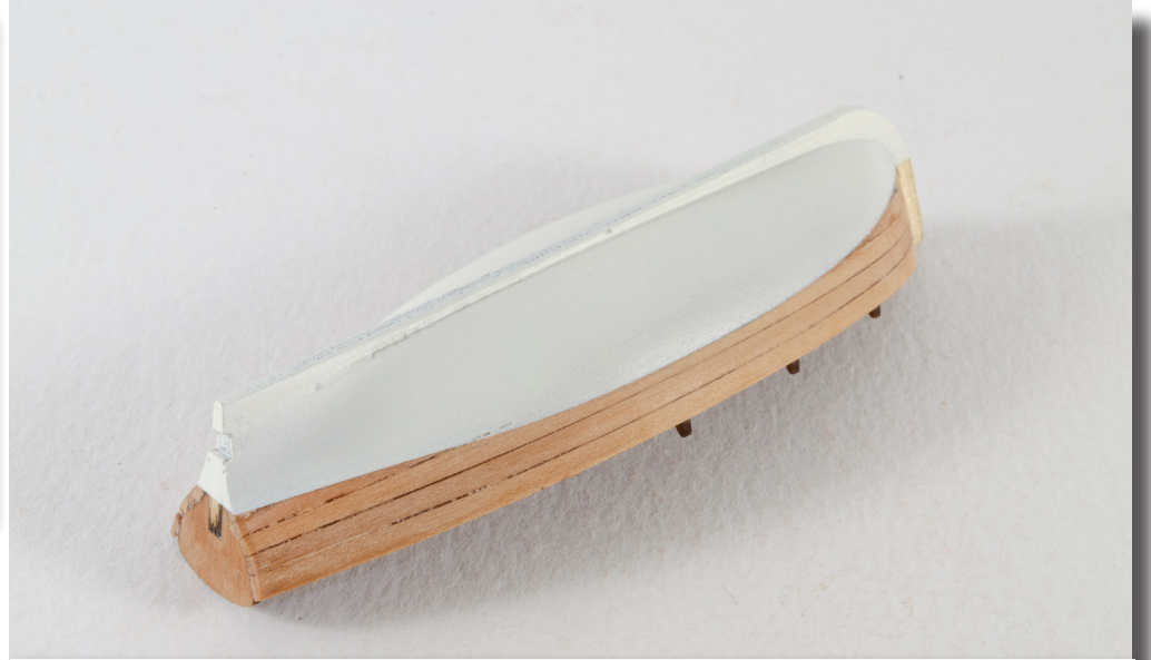
139. Mark the hull waterline using drawing reference and mask the model before spraying the underside with white paint.
