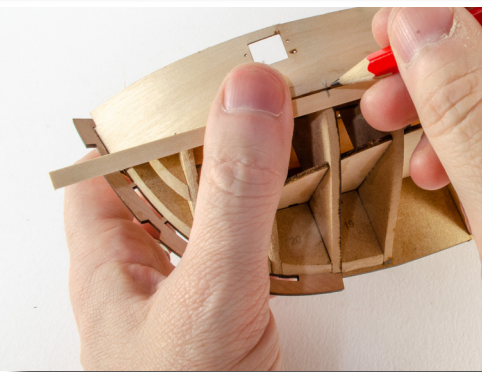
44. We can now start the first layer of planking using the 1.5x5mm limewood strips. You will need to taper these planks as you fit them, otherwise they won't conform to the hull shape as you progress. This is a very easy task. First, lie your first plank below the plywood Bulwark Patterns and where the plank tries to overlap the ply, make a pencil mark. Do this at front and rear of hull. Put a rough forward and end mark on the plank too.
