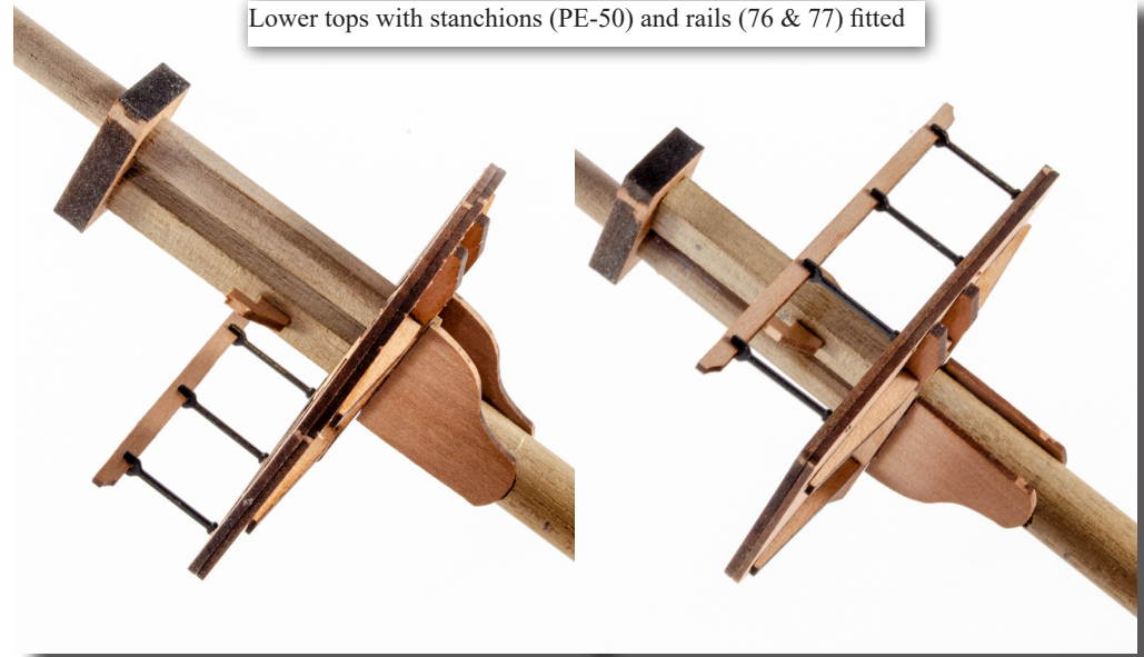
Fore and main masts complete. Refer to the full size plans for fitting and location of mast bands and cleats.
