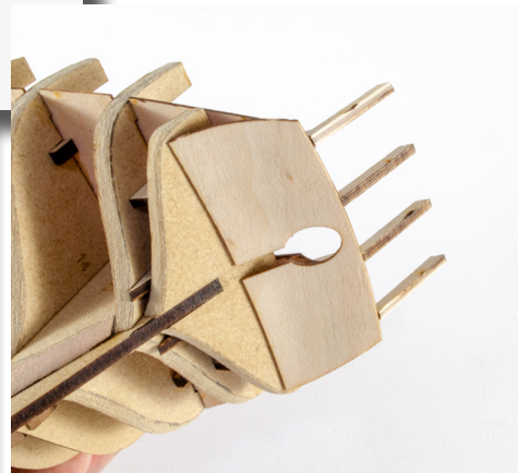
34. Take the Stern Counter 38 from the 0.8mm Ply sheet, and glue into position as shown. The temporary Stern/Rudder post will simply help to make sure you align the stern counter in the correct position. You may wish to soak the Stern Counter in hot water for 30 minutes to make it more pliable. We recommend that you use CA gel for this as you will have a few seconds to position it correctly, and you also won't need to pin into the thin frames.
