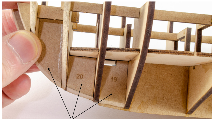
26. Now glue the Bow Pattern 20 between Bulkheads 2 & 3, and Bow Pattern 19 between Bulkheads 3 & 4, as shown in this photo.
