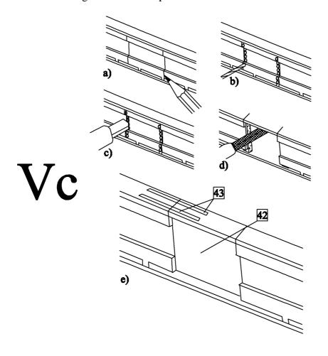
d) Firs grind rudder into needed shape. Then glue copper plates o the hull and rudder. Finally glue ruder together with hinges 46 and 47 to the hull.
